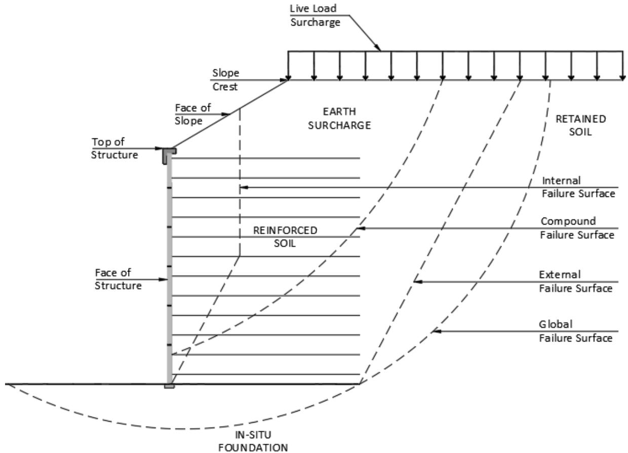
Fig 1. MSE Failure Surfaces for Stability Analyses
