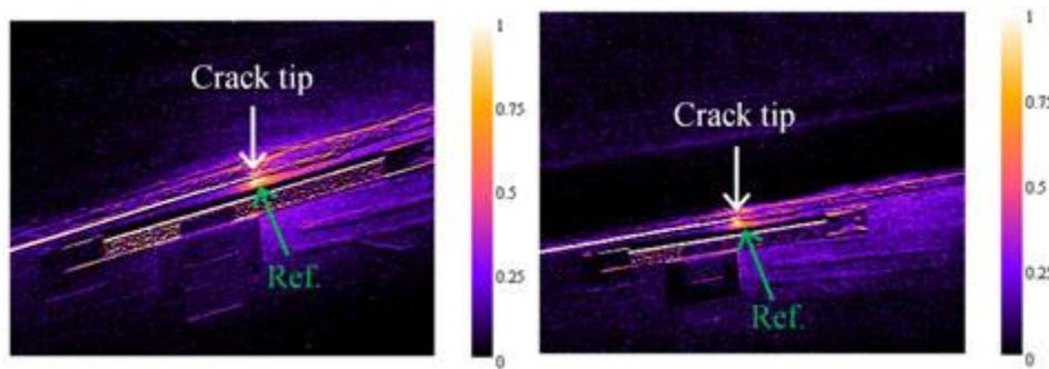
Figure 8: Result of crack detection in actual steel deck from distant place (Sakagami et al. 2010).
