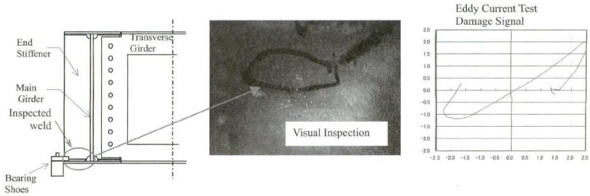
Figure 4: Detection of under coating cracks (Ichinose et al. 2007)
