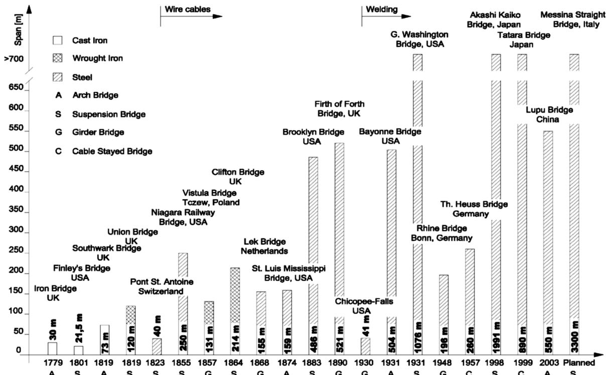
Figure 2: Histogram of the development of steel use in bridge construction since 1779 (Biezma and Schanack 2007)
