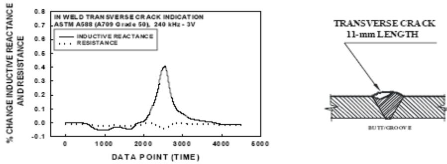
Figure 3: reactive and resistive components of signal response for transverse-to-weld Crack (Bader 2008).
