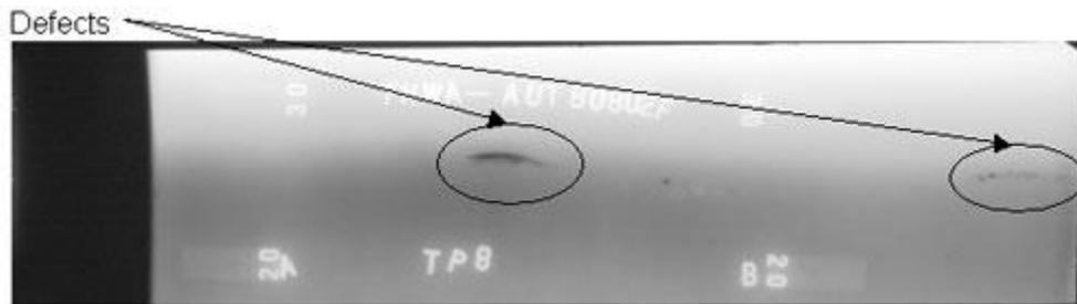
Figure 5: Typical radiograph image showing locations of two cracks (Bader 2008)
