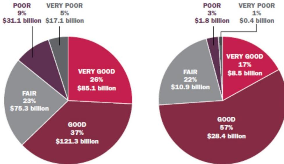
Figure 1: Physical condition rating by replacement value For Roads (Left) and bridges (Right). (Canadian infrastructure report card 2016)
