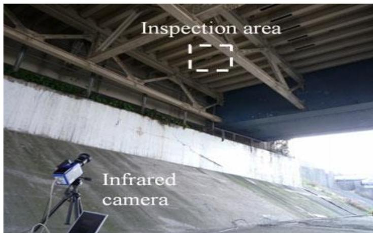
Figure 7: Self-reference lock-in measurement with telescopic lens for actual steel bridge (Sakagami et al. 2010).
