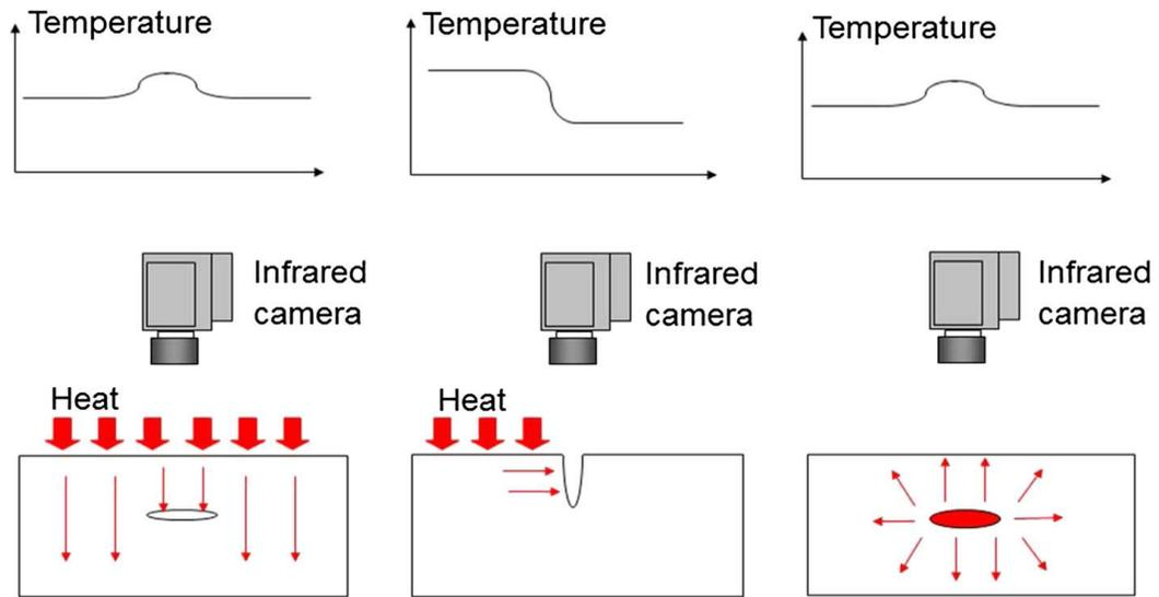
Figure 6: Illustrations of thermal nondestructive testing classification (Sakagami et al. 2010).
