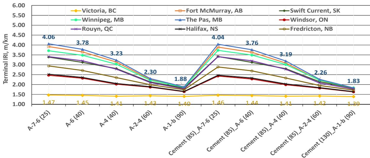
Figure 2a. Trends of the predicted IRI with variations of subgrade materials (native vs soil-cement)
