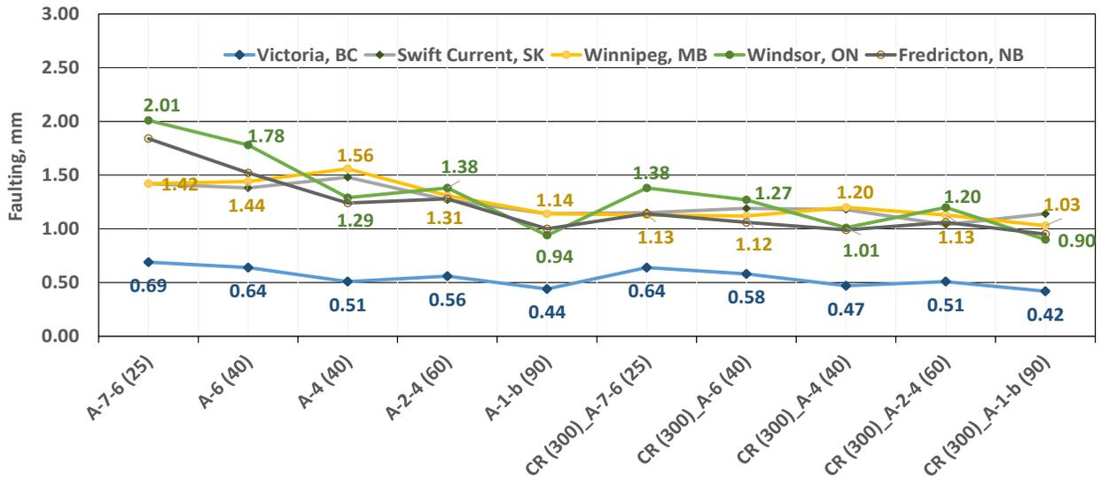
Figure 4. Trends of the predicted faulting with variations of subgrade materials (native vs granular subgrade)
