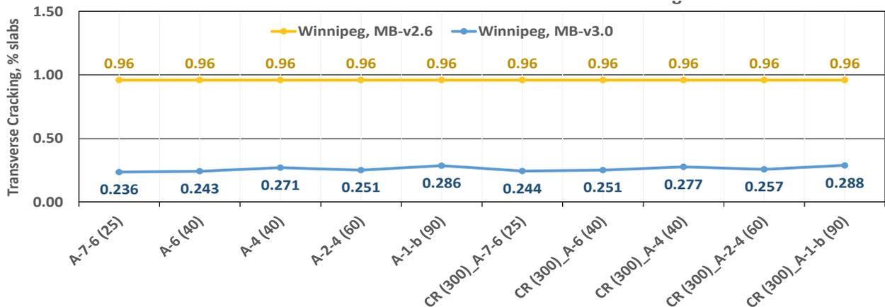
Figure 7. Trends of transverse cracking with variations of subgrade materials (software v2.6 vs v3.0)
