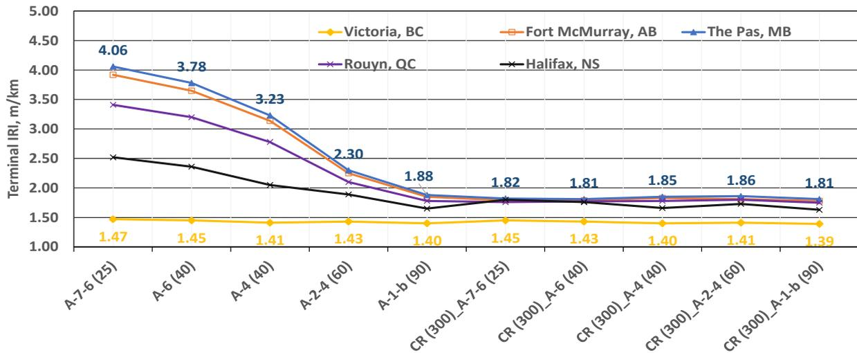
Figure 2b. Trends of the predicted IRI with variations of subgrade materials (native vs granular subgrade)
