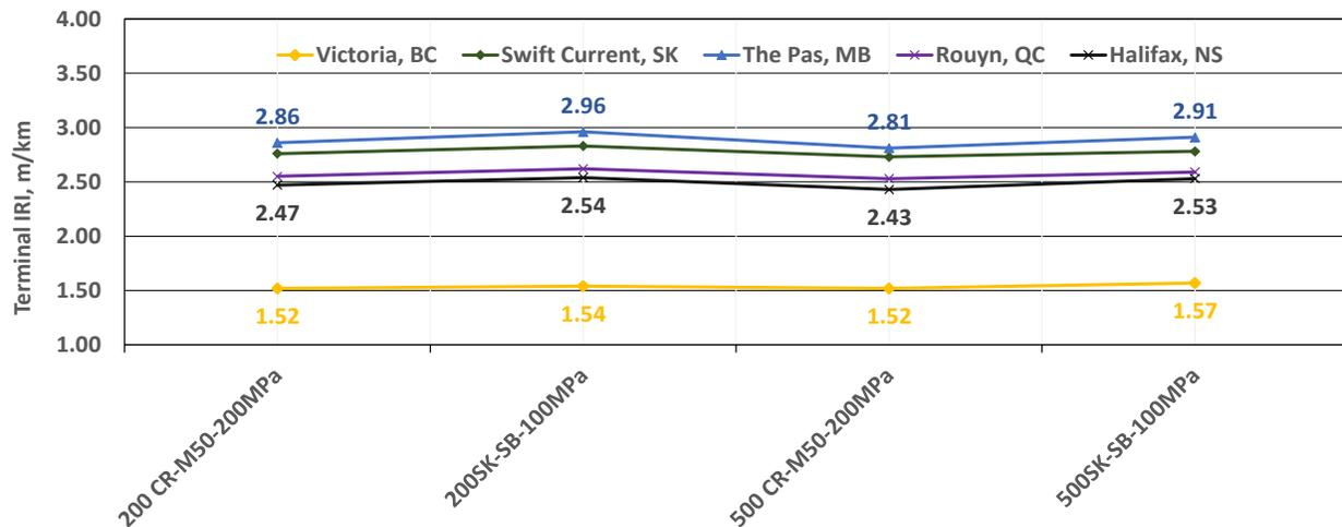
Figure 14. Trends of the predicted IRI with variations of subbase layer materials and thickness (v2.6)
