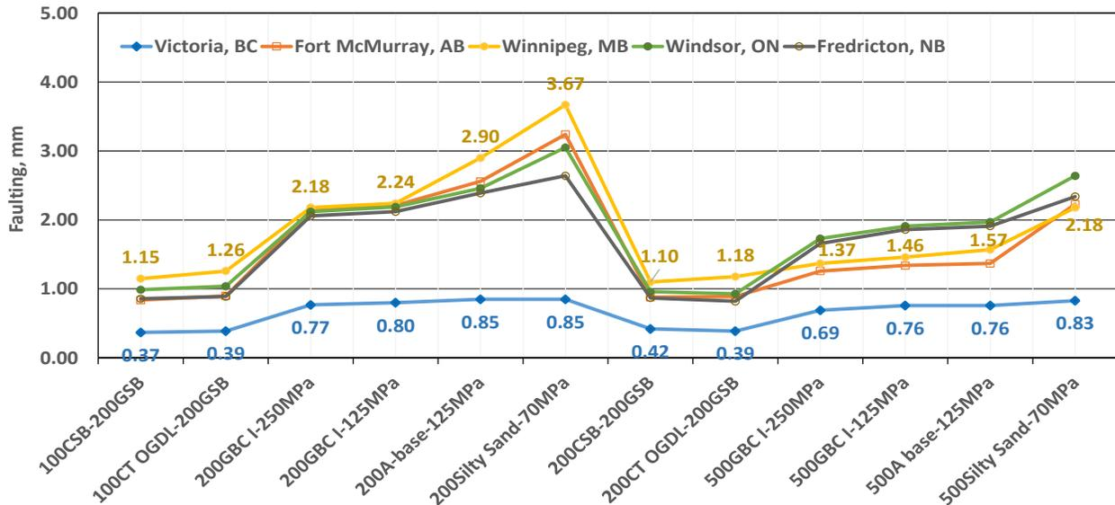
Figure 10. Trends of the predicted faulting with variations of base layer materials and thickness (v2.6)
