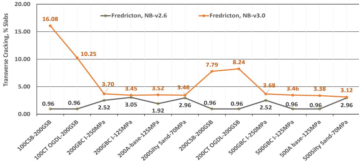
Figure 13. Trends of transverse cracking with variations of base layer materials and thickness (v2.6 vs v3.0)
