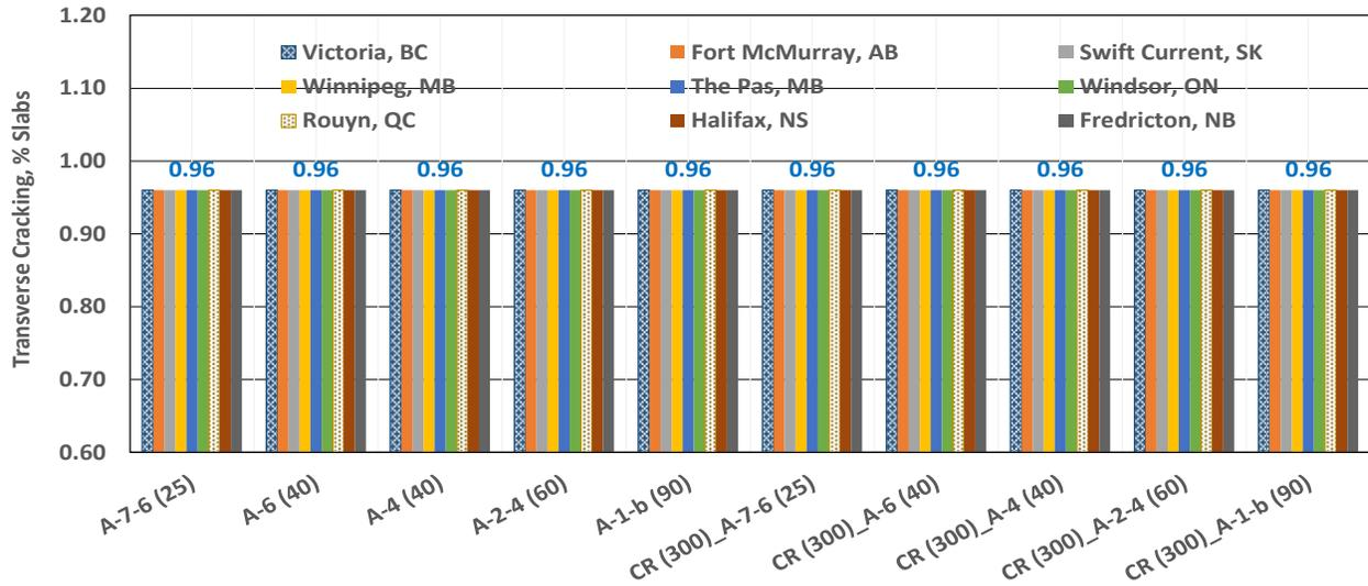
Figure 6. Trends of transverse cracking with variations of subgrade materials (native vs granular subgrade)
