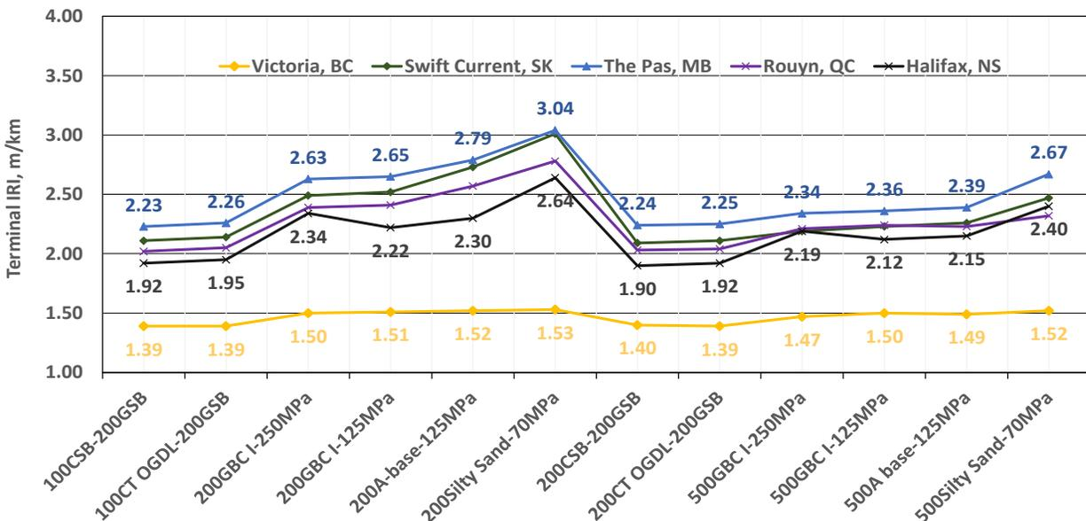
Figure 8. Trends of the predicted IRI with variations of base layer materials and thickness (v2.6)
