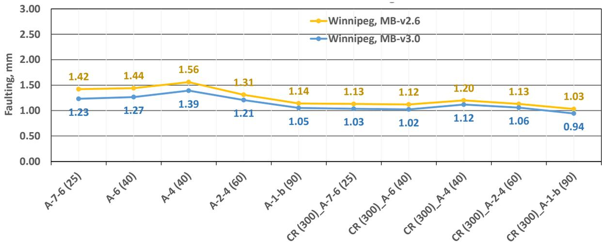
Figure 5. Trends of the predicted faulting with variations of subgrade materials (software v2.6 vs v3.0)
