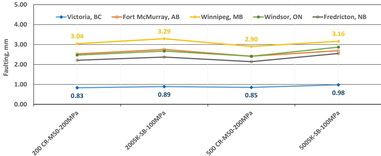
Figure 15. Trends of the predicted faulting with variations of subbase layer materials and thickness (v2.6)
