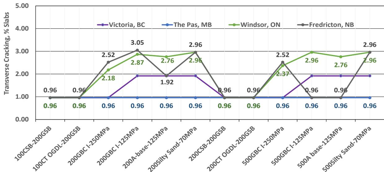
Figure 12. Trends of the predicted transverse cracking with variations of base layer materials and thickness
