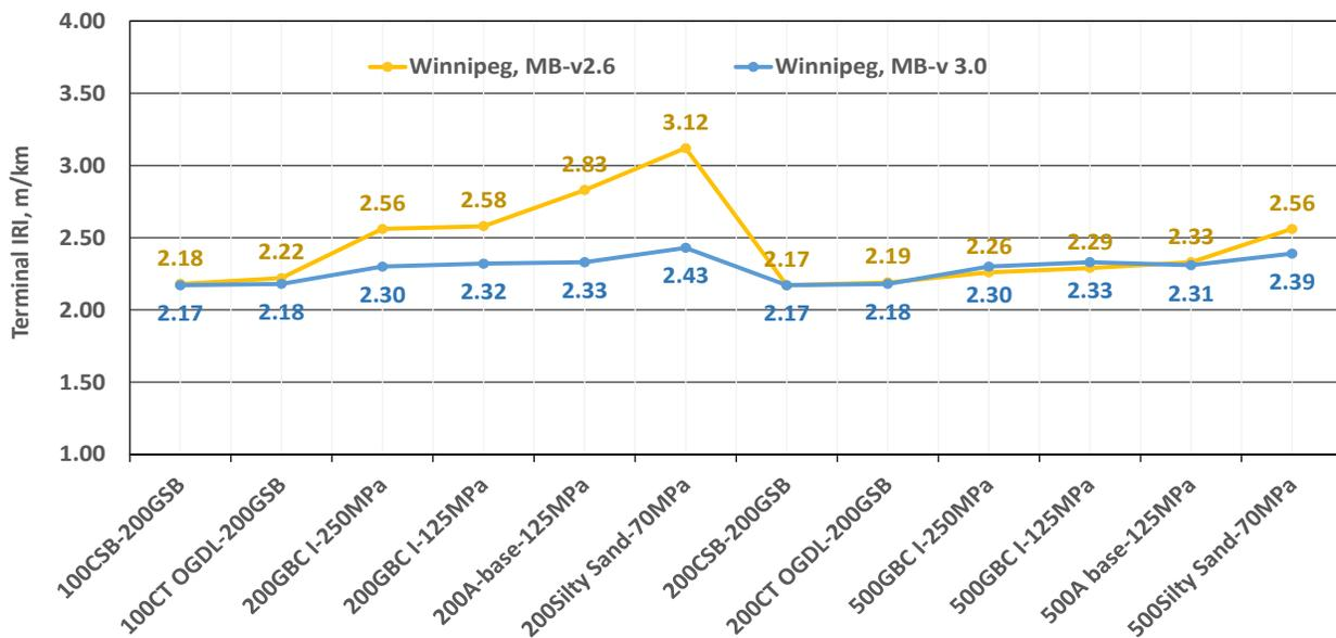
Figure 9. Trends of the predicted IRI with variations of base layer materials and thickness (v2.6 vs v3.0)
