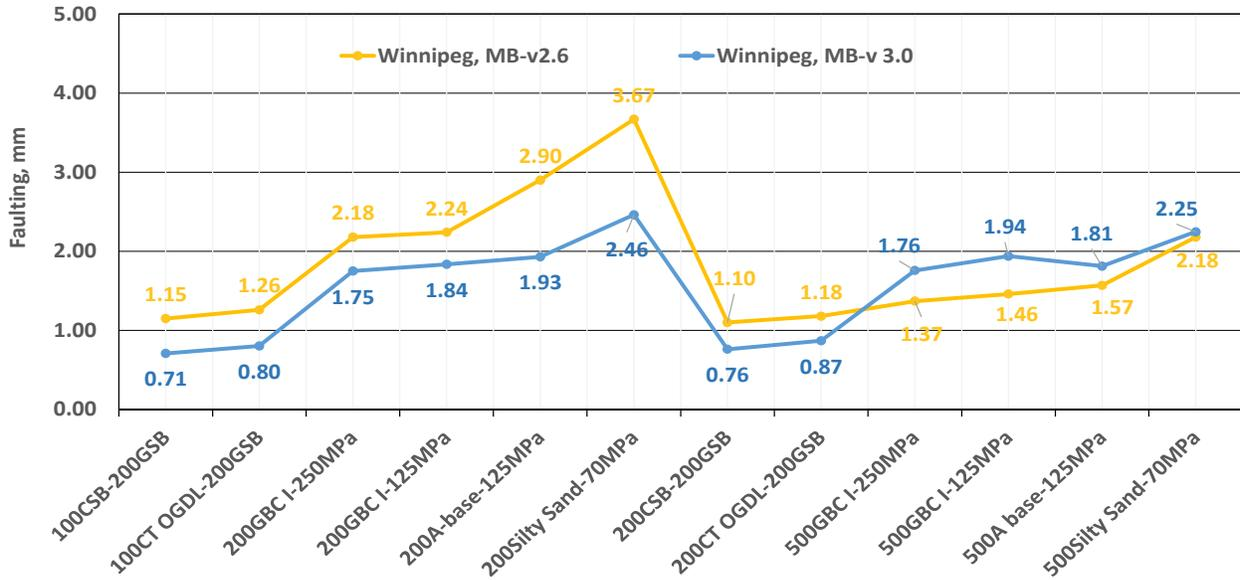
Figure 11. Trends of faulting with variations of base layer materials and thickness (v2.6 vs v3.0)
