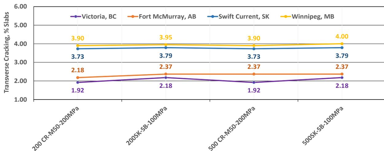
Figure 16. Trends of the transverse cracking with variations of subbase layer materials and thickness (v2.6)
