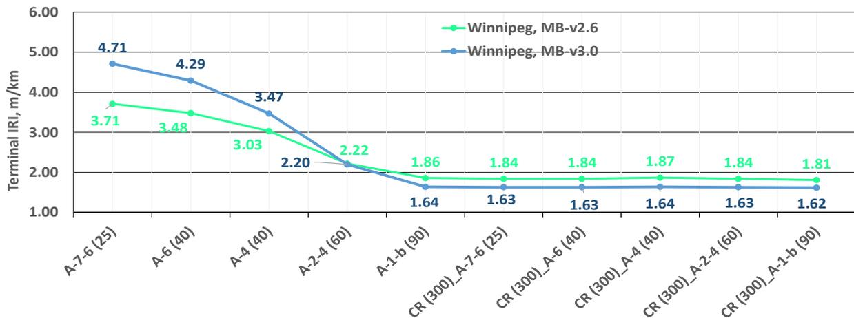
Figure 3. Trends of the predicted IRI with variations of subgrade materials (Software v2.6 vs v3.0)
