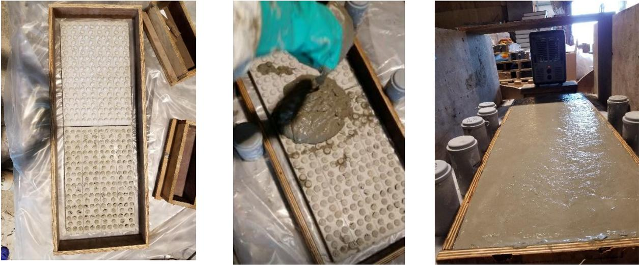
Figure 1 – Restrained plastic shrinkage
