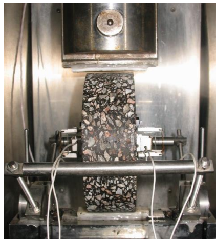
Figure 3. The experimental setup of the Superpave IDT test
