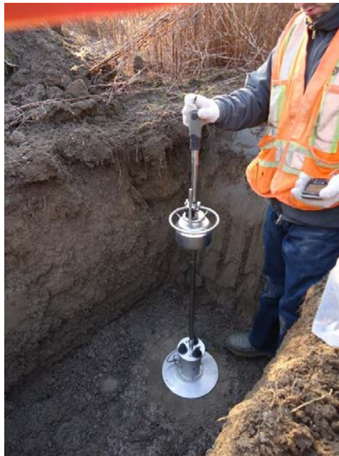
Figure 2: LWD Testing in Test Pits
