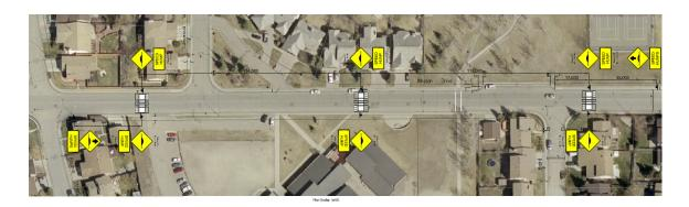
Figure 3 – Layout of Speed Cushions on Whelan Drive
