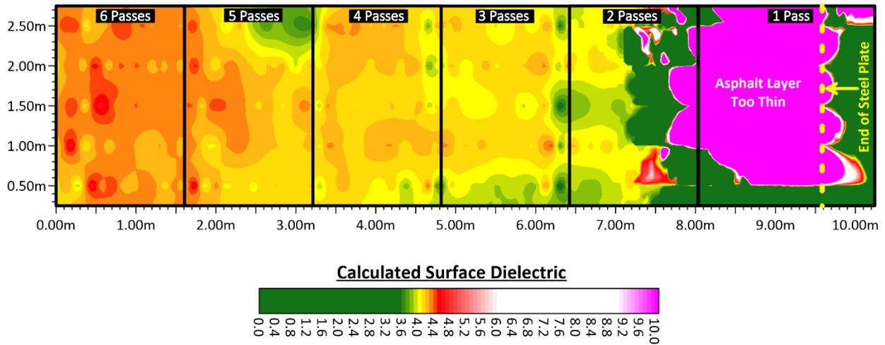
**Figure 2 - Variation in surface dielectric at trial section for MacKay Bridge paving trial.**
