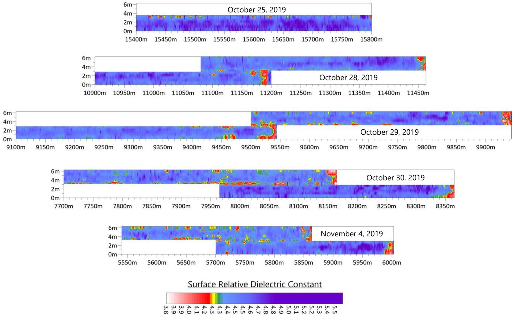
Figure 4 - Variation in surface dielectric value over test sections.
