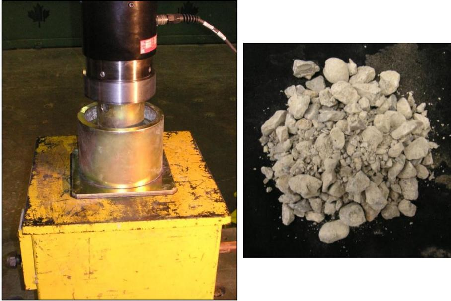
**Figure 1 Aggregate crushing value test apparatus and crushed RCA-1**
