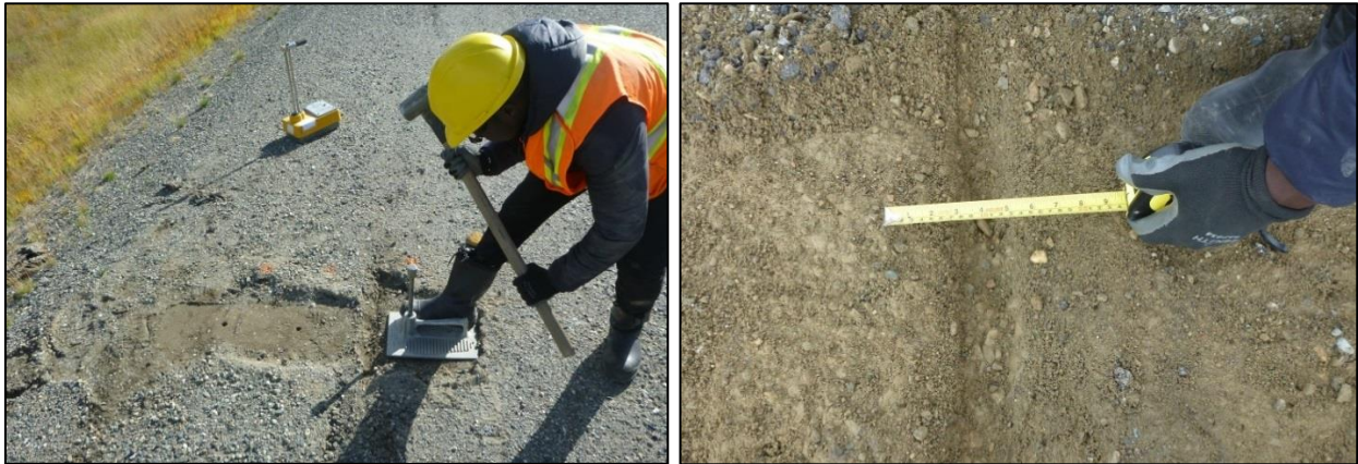
Figure 9. Measuring road density with a nuclear density gauge (left), and edge crack filled with gravel (right) at km 40.
