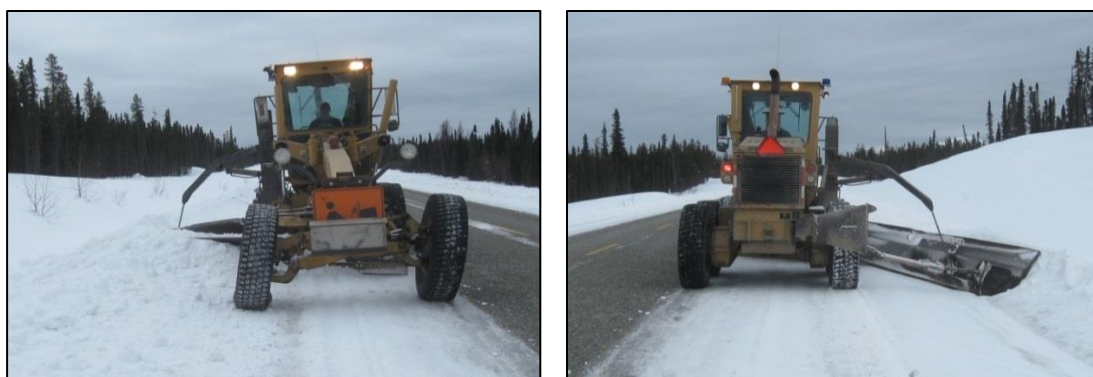
Figure 16. Blading and winging snow off of the road shoulder and sideslope, 7 April 2016.
