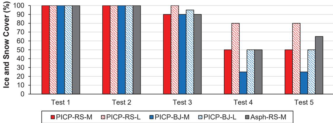
Figure 4-5: Ice and snow coverage during melting and refreeze on 16/Feb/2019.
