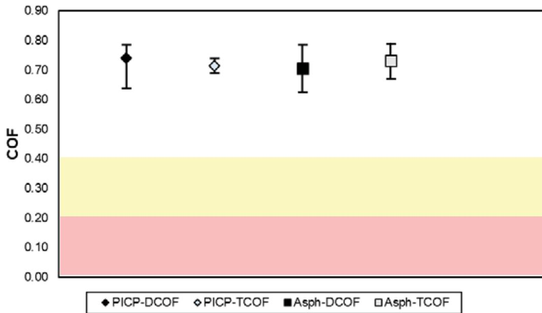
Figure 4-1: Surface friction during dry pavement conditions.
