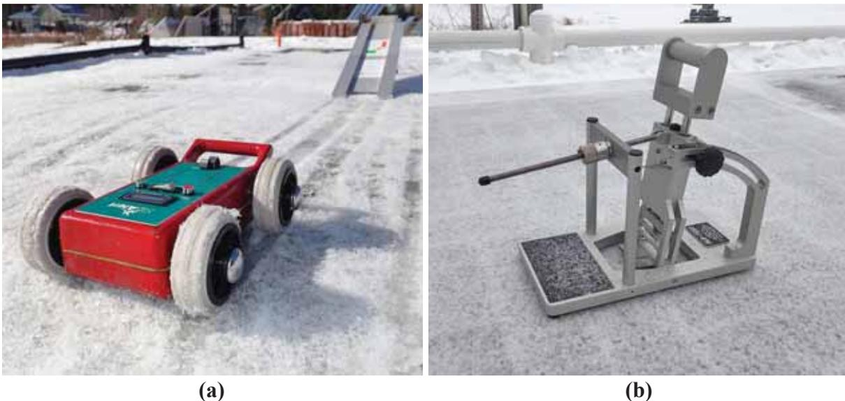
**Figure 3-1: Friction measuring devices in use on ice-covered PICP surfaces: (a) SlipAlert and (b) Mark IIIB.**
