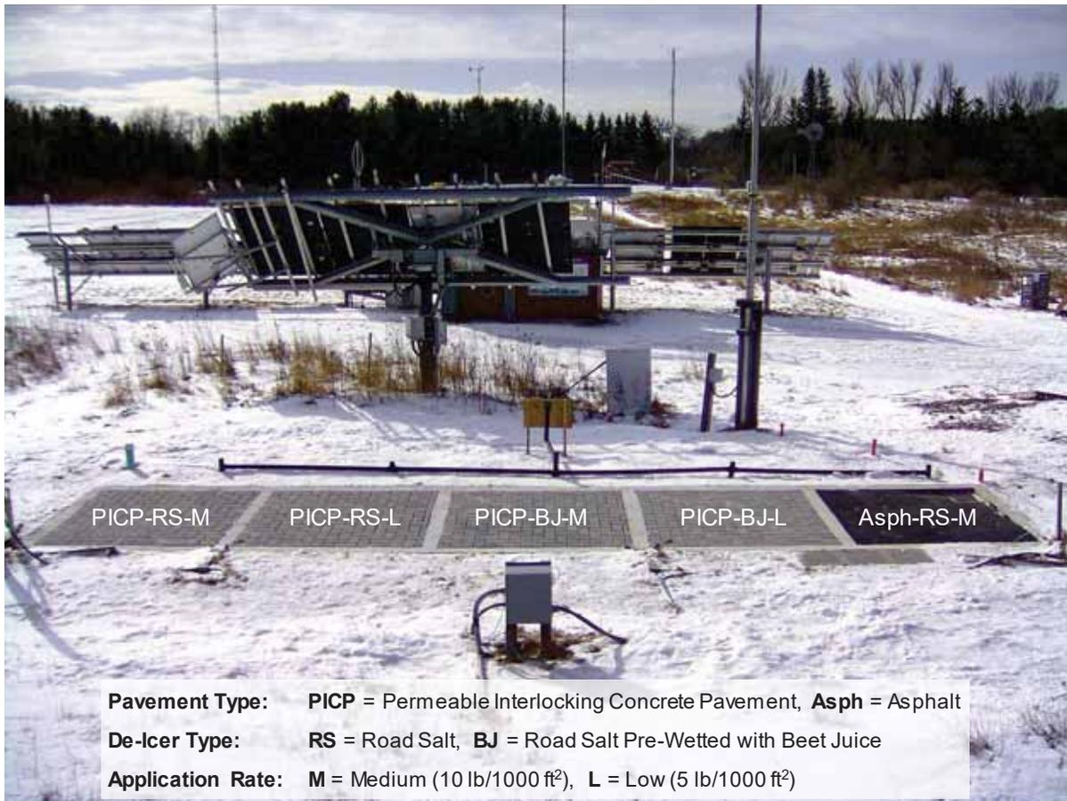
Figure 2-2: Surface layout of the outdoor pavement test site (facing south).
