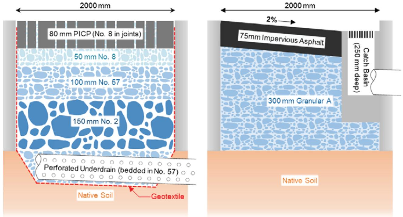
Figure 2-3: Cross-sectional layout of PICP (left) and asphalt test cells (right).
