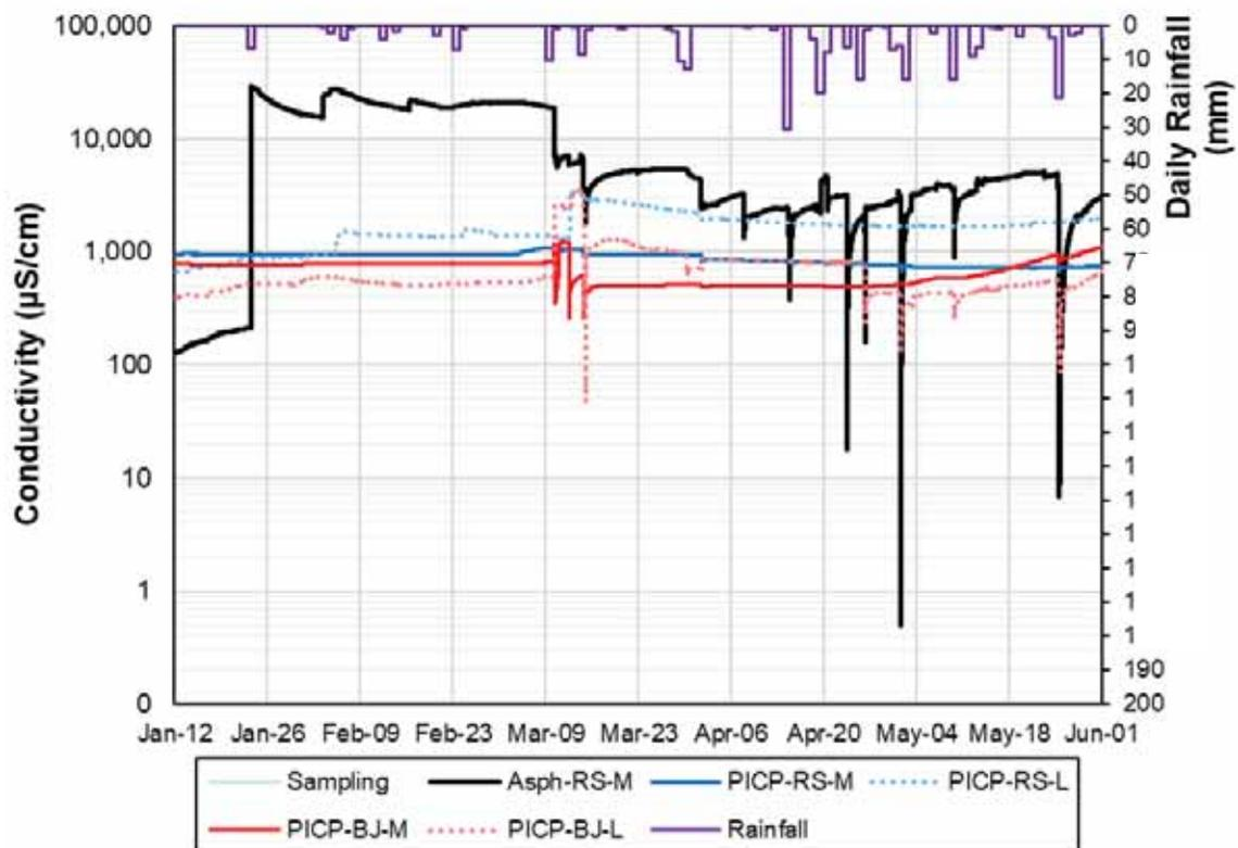
Figure 4-16: Conductivity measurements collected during the 2019 winter and spring.
