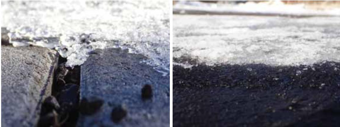
Figure 4-7: Ice cover characteristics on 16/Feb/2019: partially detached ice cover on PICP (left) and ice transition into wet pavement on asphalt (right)
