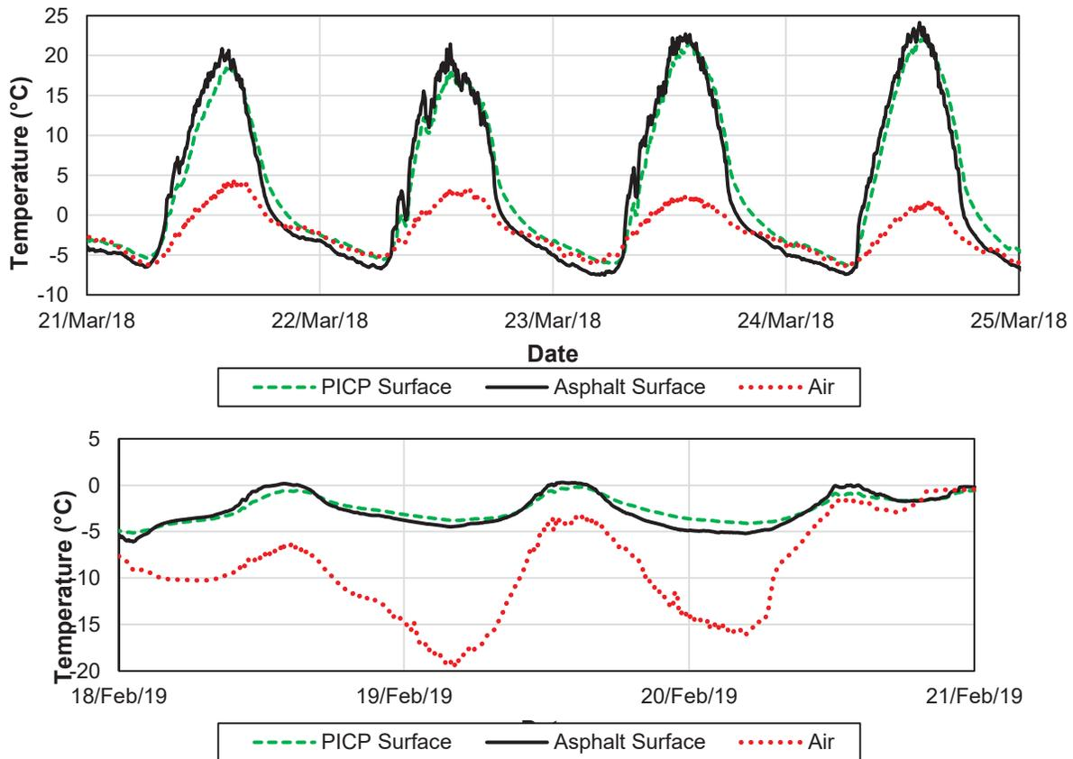
Figure 4-15: Air and surface temperatures during a typical diurnal pattern in March 2018 (top) and during a snow-covered period in February 2019 (bottom).
