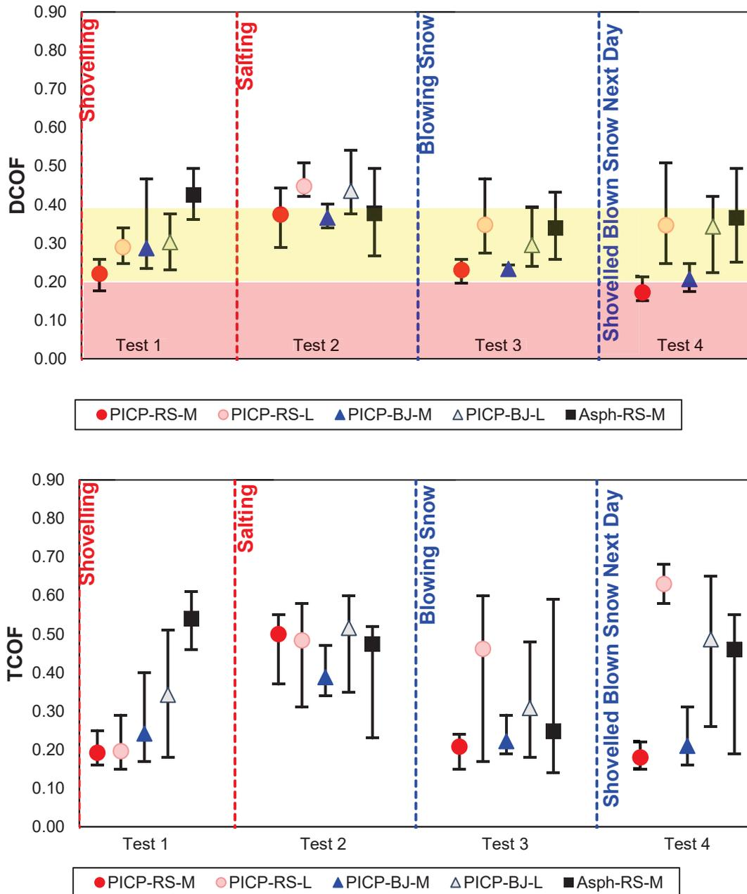
**Figure 4-13: DCOF (top) and TCOF (bottom) data collected on 30/Jan/2019 and 31/Jan/2019 after cells were shovelled to a thin layer of snow.**
