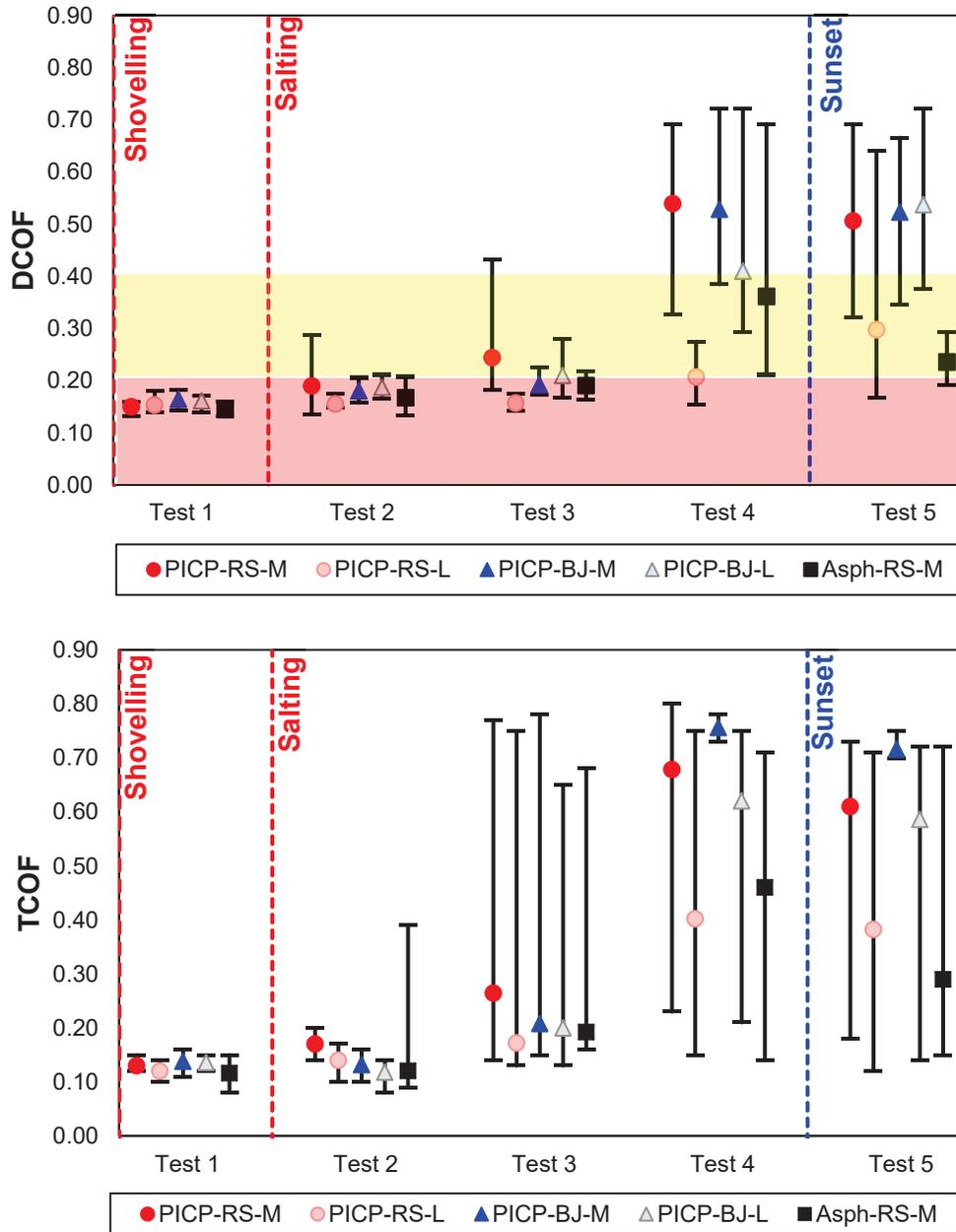
**Figure 4-4: Means and ranges of DCOF (top) and TCOF (bottom) measurements collected during 16/Feb/2019 experiment.**
