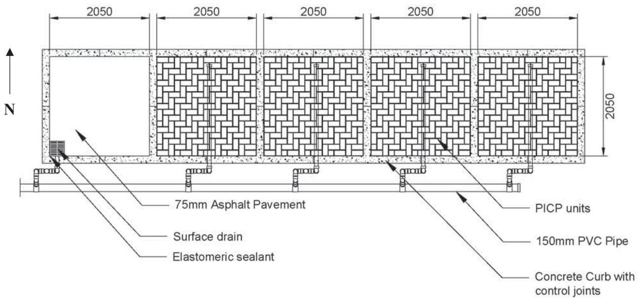
Figure 2-1: Test Pad Layout. Dimensions are presented in mm.
