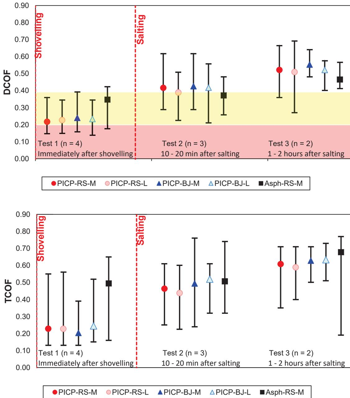
Figure 4-2: Means and ranges of DCOF (top) and TCOF (bottom) measurements for shoveled snow experiments.
