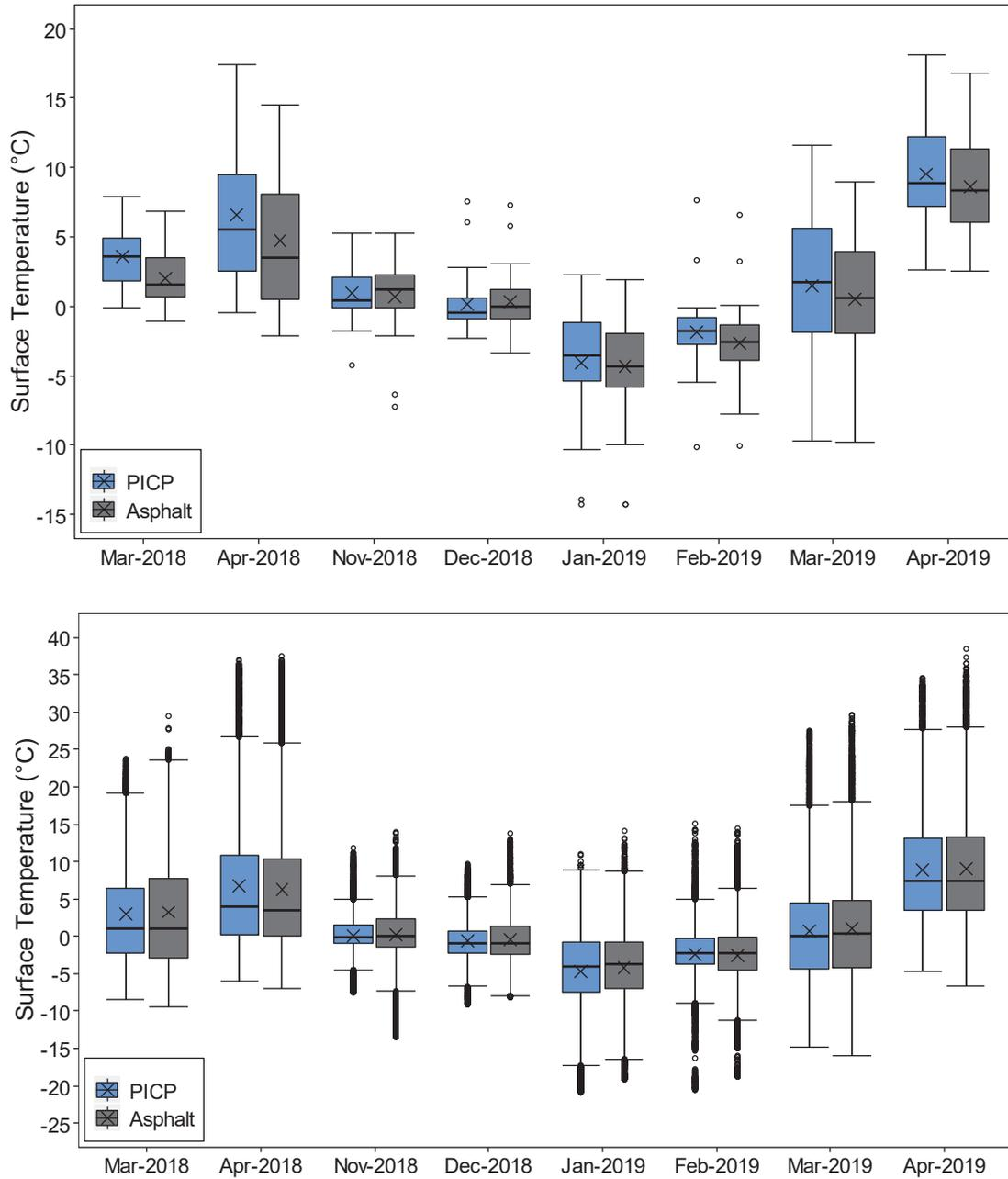
Figure 4-14: Box plots of surface temperatures at sunset (top) and overall (bottom)
