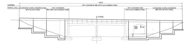
FIGURE 5 - ELEVATION OF TUNNEL PORTAL, SHOWING STEPPED FOOTINGS AND CONTROL BUILDING
