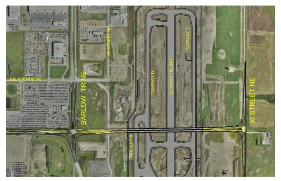
FIGURE 1B - TUNNEL LAYOUT UNDER THE RUNWAY AND TAXIWAYS (NORTH IS UP, AIRPORT TRAIL RUNS EAST WEST)
