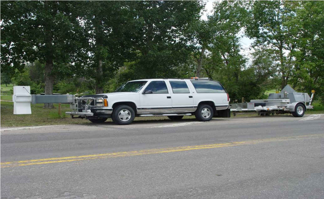
Figure 2 Ground Penetrating Radar and Dynatest Heavy Weight Deflectometer
