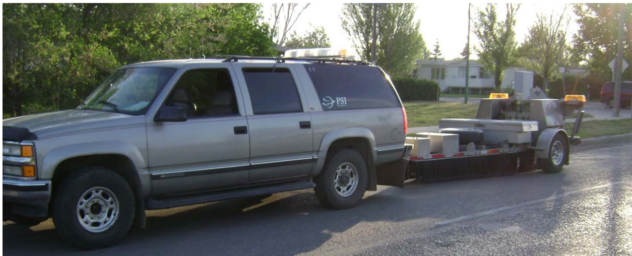
Figure 6 Heavy weight deflectometer on 8 th Street
