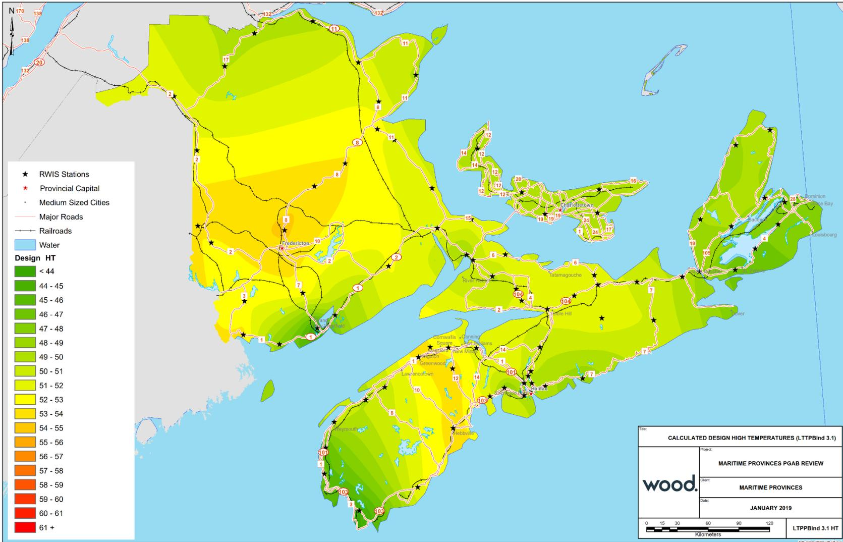
Figure 6. Pavement design high temperatures in the Maritimes (LTPPBind V3.1).
