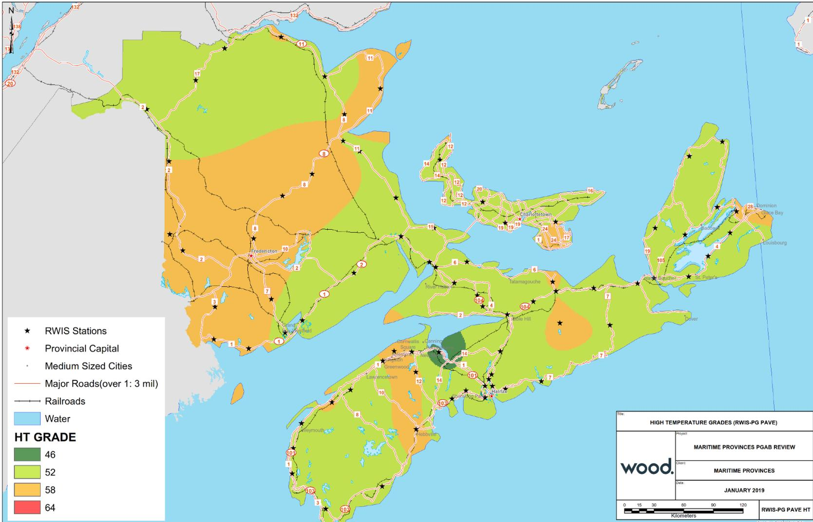
Figure 9. Minimum high temperature performance grades required in the Maritimes (RWIS pavement temperature).
