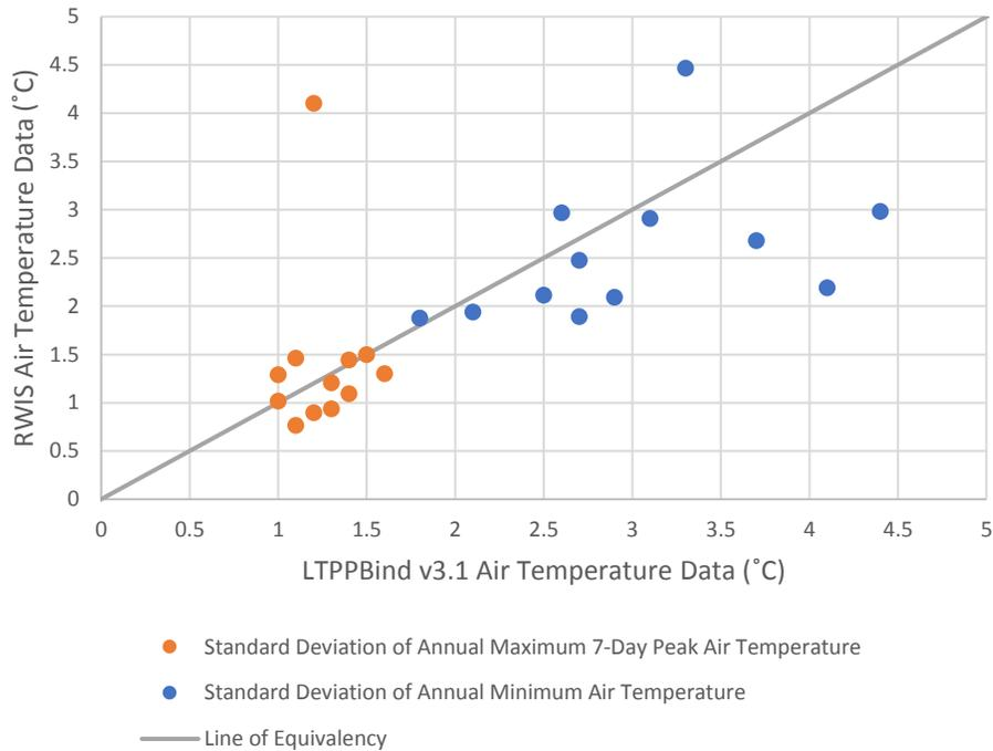
Figure 4. Standard deviations of design temperatures developed using RWIS air temperatures vs. LTPPBind V3.1.
