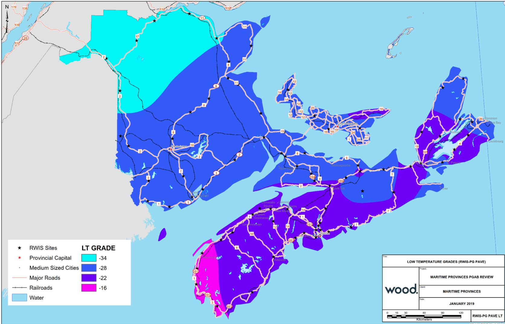
Figure 10. Maximum low temperature performance grades required in the Maritimes (RWIS pavement temperature).
