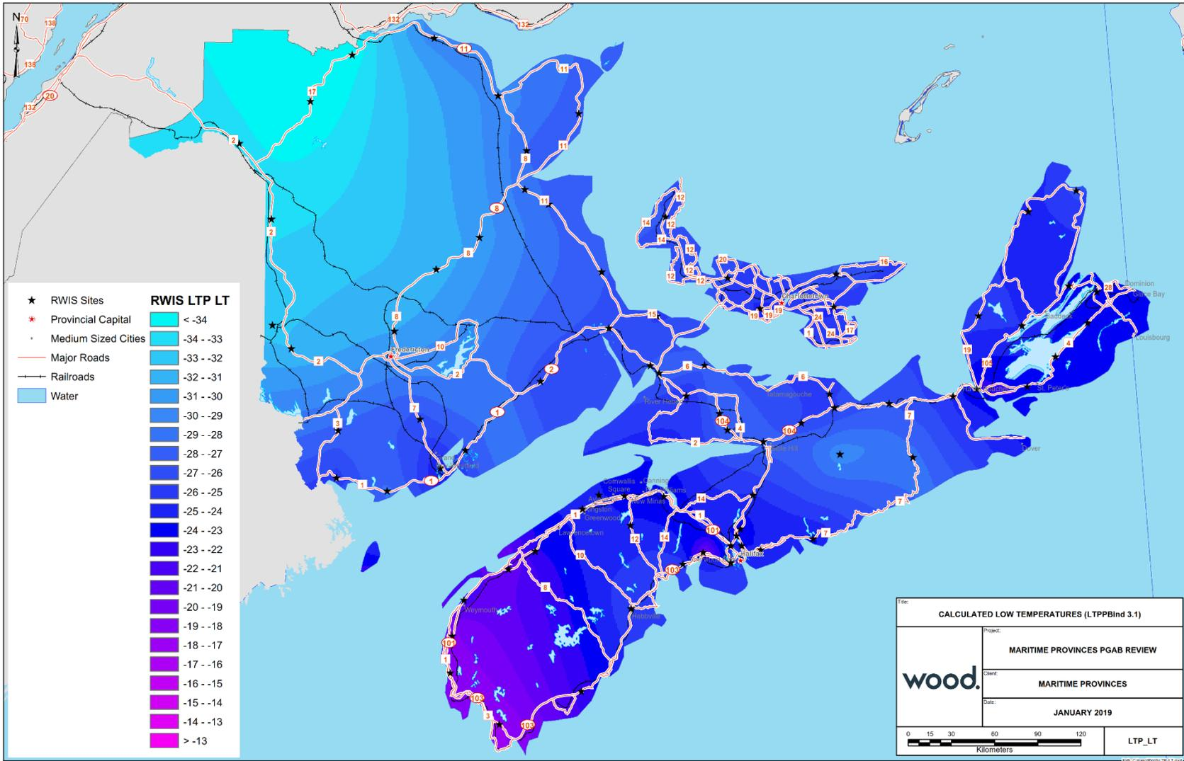
Figure 8. Pavement design low temperatures in the Maritimes (LTPBind V3.1).
