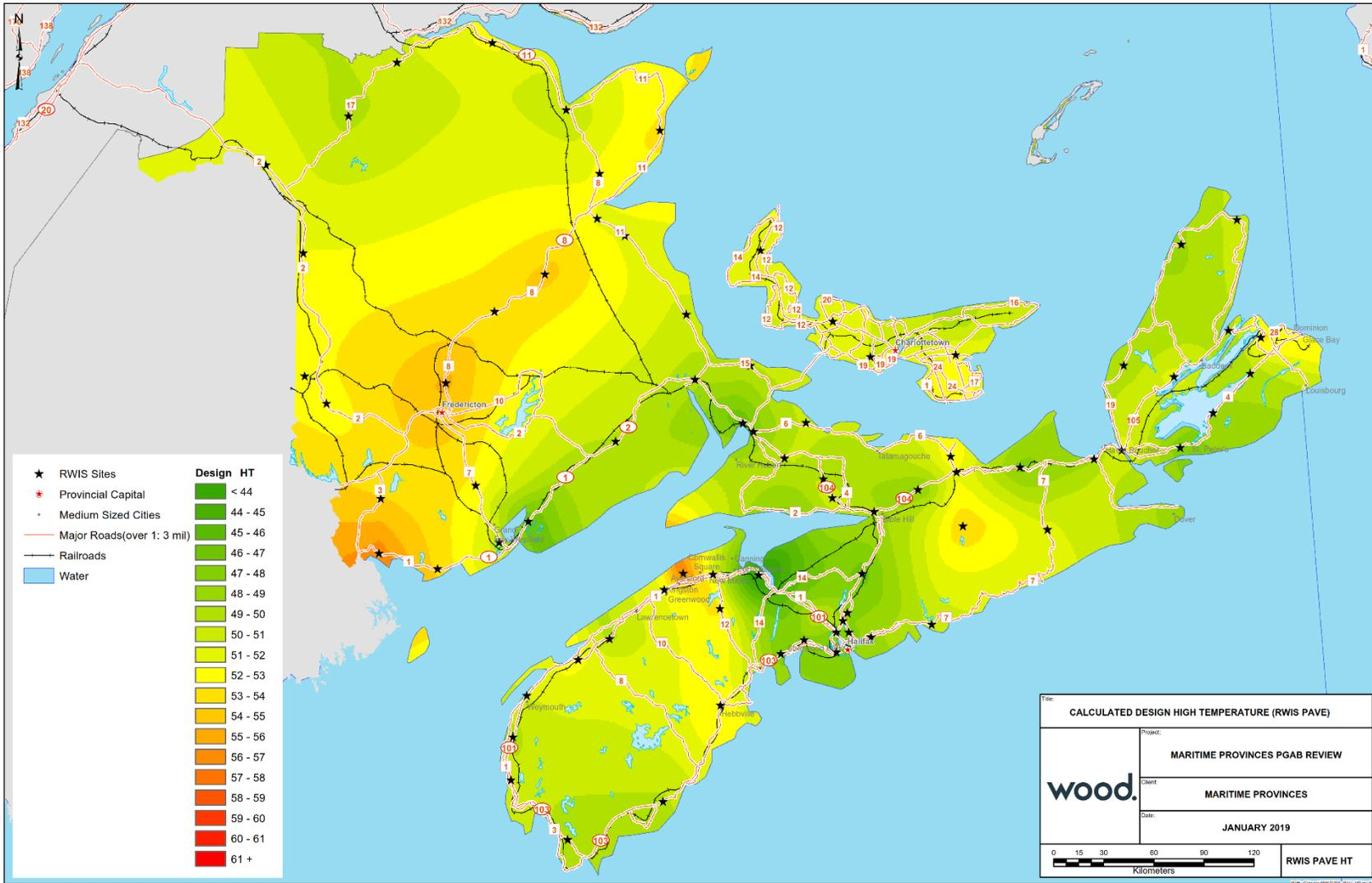
Figure 5. Pavement design high temperatures in the Maritimes (RWIS pavement temperature).
