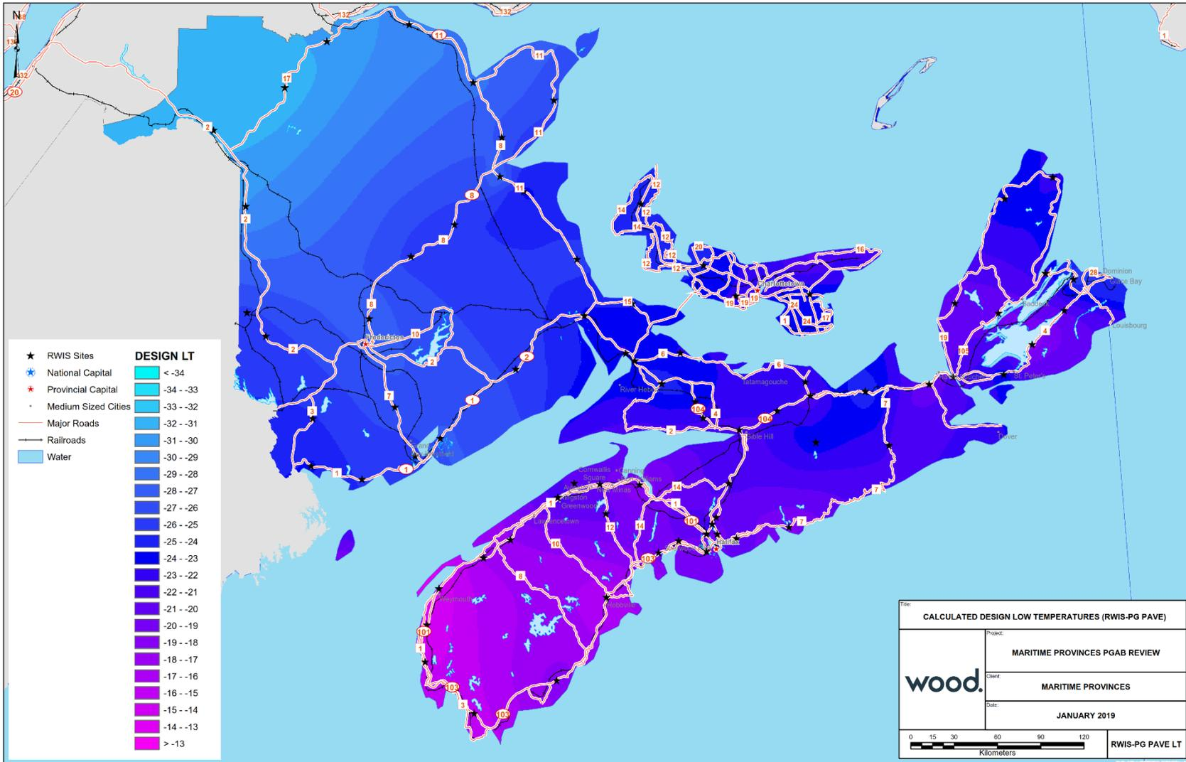
Figure 7. Pavement design low temperatures in the Maritimes (RWIS pavement temperature).
