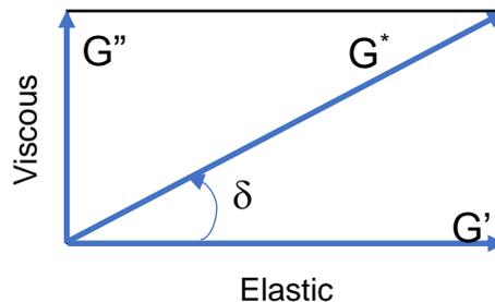
Figure 2 - Schematic of complex shear modulus,  $G^*$ , and phase angle,  $\delta$ .
