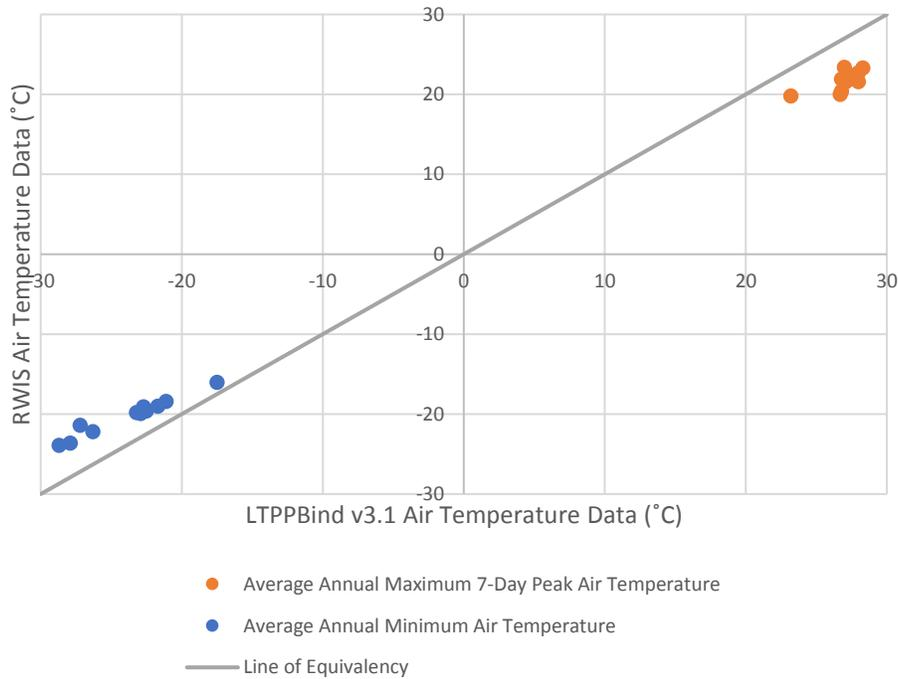
Figure 3. Average design temperatures developed using RWIS air temperatures vs. LTPPBind V3.1.
