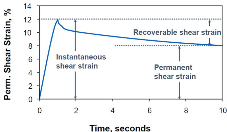
Figure 1. Schematic of MSCR data (from Anderson, 2014).
