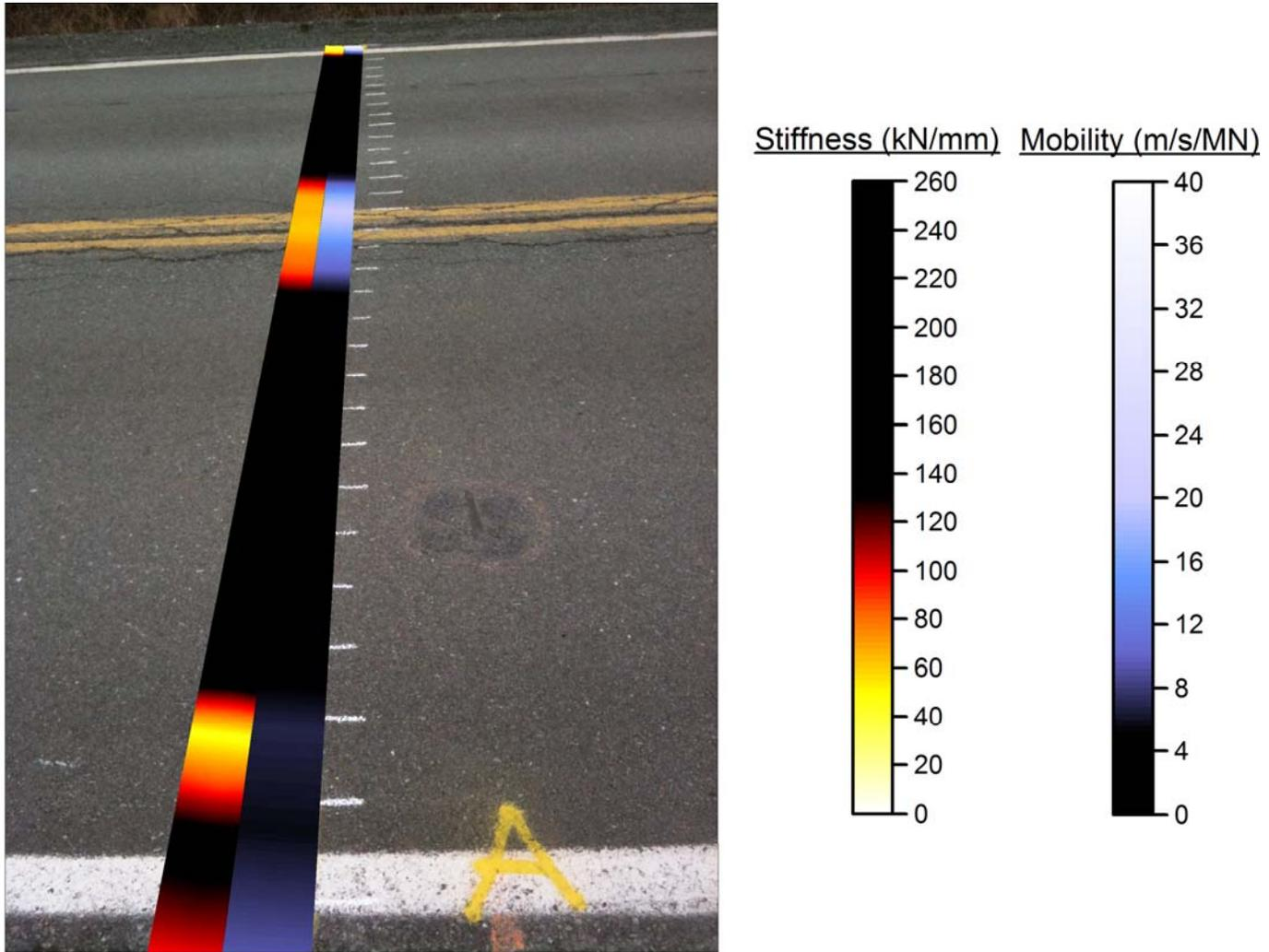
Figure 4 – Variation in dynamic stiffness and mobility across a typical damaged pavement section.
