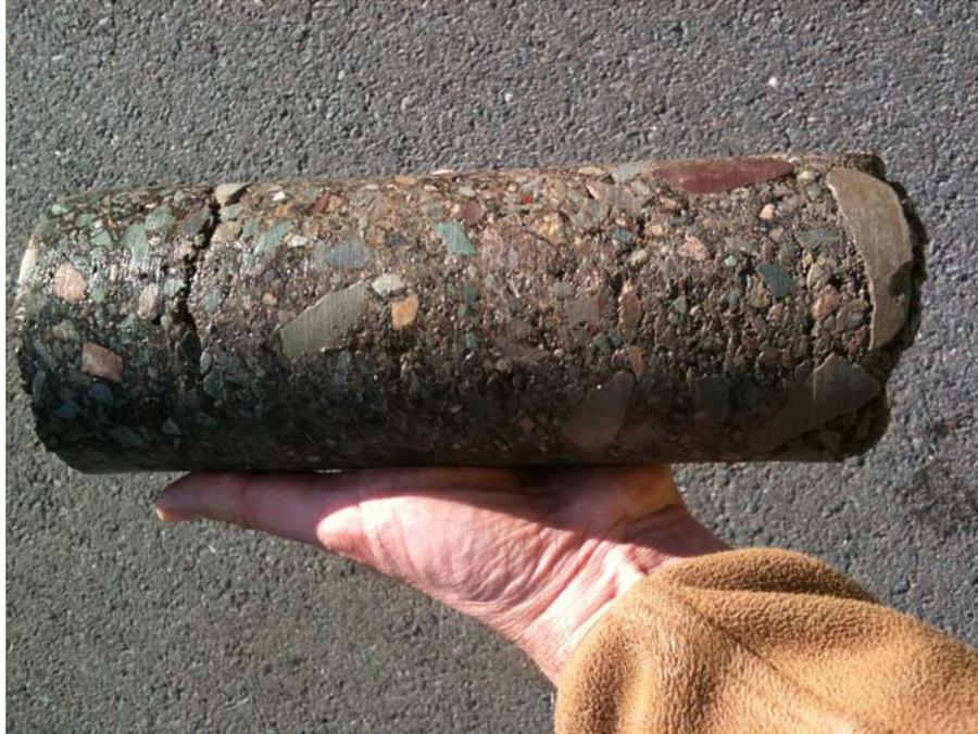
Figure 6 – Photograph of intact asphalt concrete and stabilized base core extracted from outer wheel path area.
