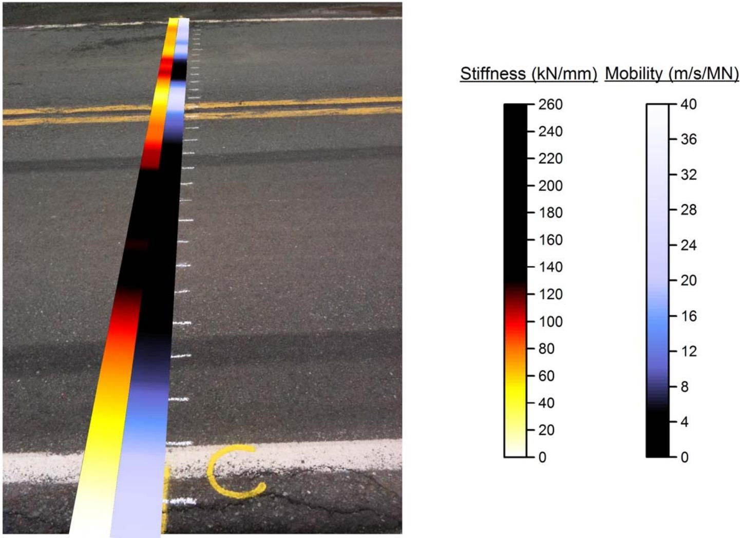
Figure 5 – Variation in dynamic stiffness and mobility across a non-typical damaged pavement section.
