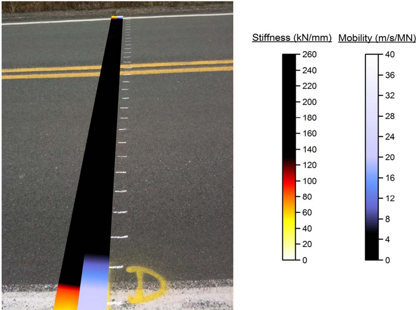
Figure 3 – Variation in dynamic stiffness and mobility across an undamaged pavement section.
