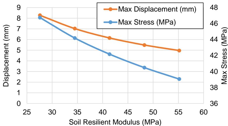
Figure 13: Variations in maximum displacement and stress under different soil stiffness.
