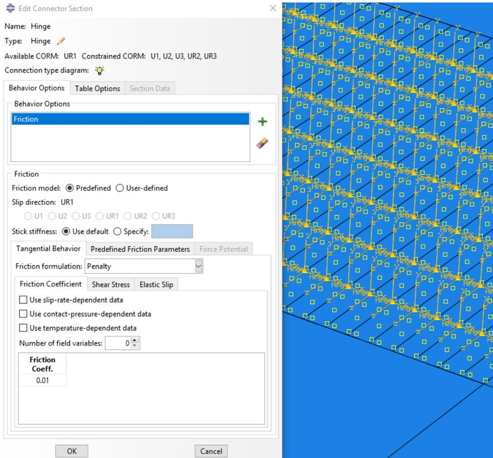
Figure 7: Definition of the hinge connectors in ABAQUS.
