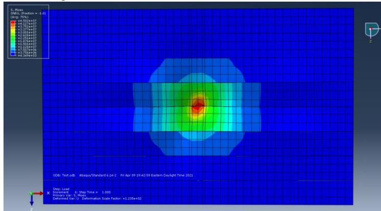
Figure 11: Visualization of stresses at the aluminum matting system, view from the top of the panels.
