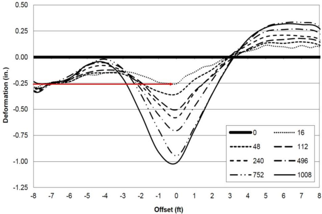
Figure 9: Full-scale panel average deformation along the loaded mat surface. Granted by FAUN Trackway.
