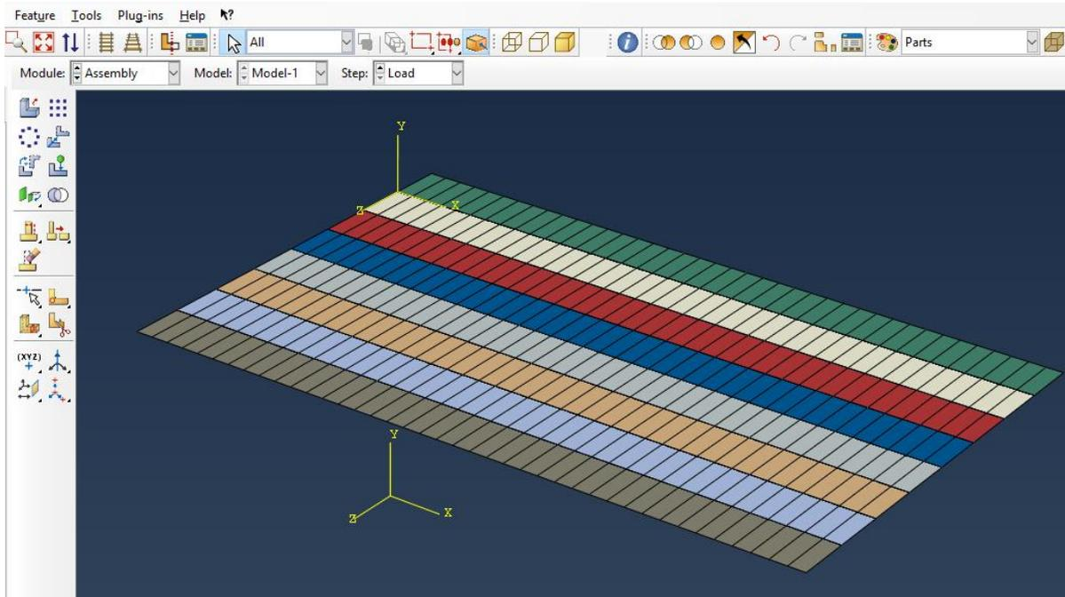
Figure 6: Panels assembly in ABAQUS.
