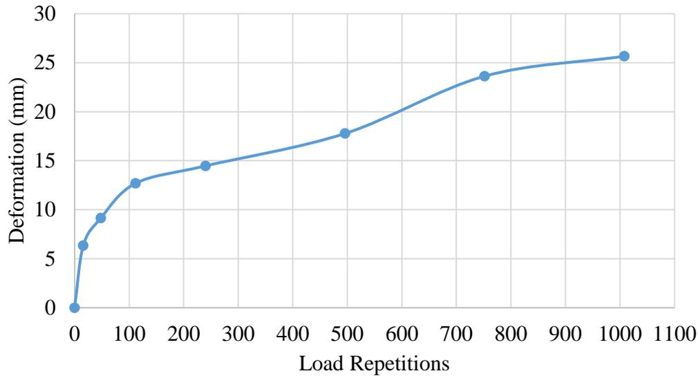
Figure 10: Full-scale maximum deflections under growing load repetitions. Modified from Figure 9.
