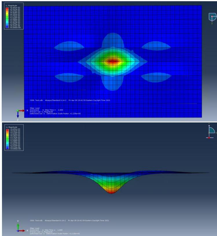
Figure 12: Deformed shape of the aluminum matting system, top figure presents a view from the top of panels, and bottom figure presents a lateral view of the panels.
