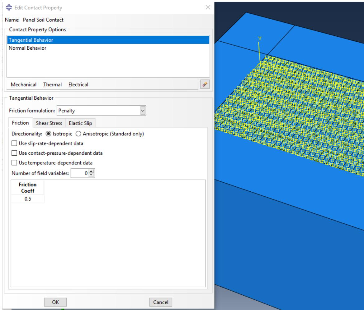
Figure 4: Contact property between panels and soil in ABAQUS.
