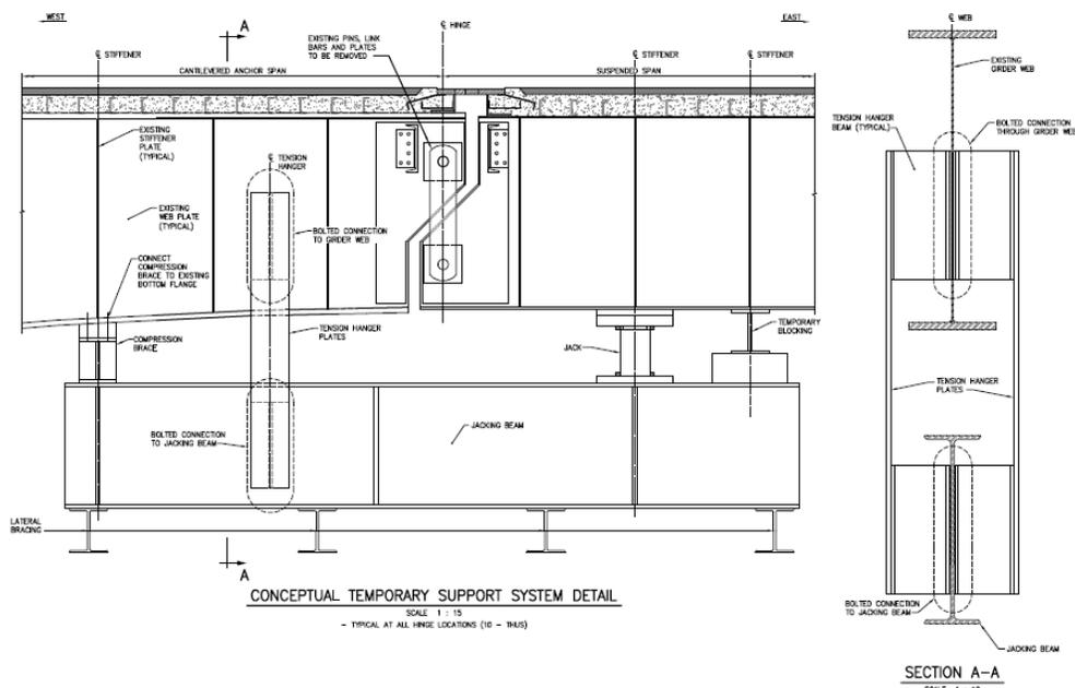
Figure 2 –Conceptual Temporary Support System Detail
