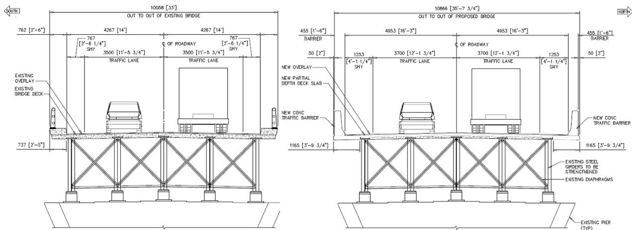
**Figure 2: Original Bridge Cross-Section (Left) and Option 1 Bridge Cross-Section (Right)**
