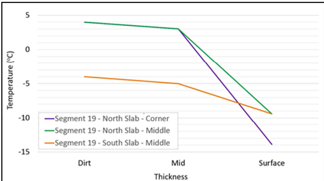
Figure 16. Temperature Distribution along Depth of Section for a Negative Temperature Differential
