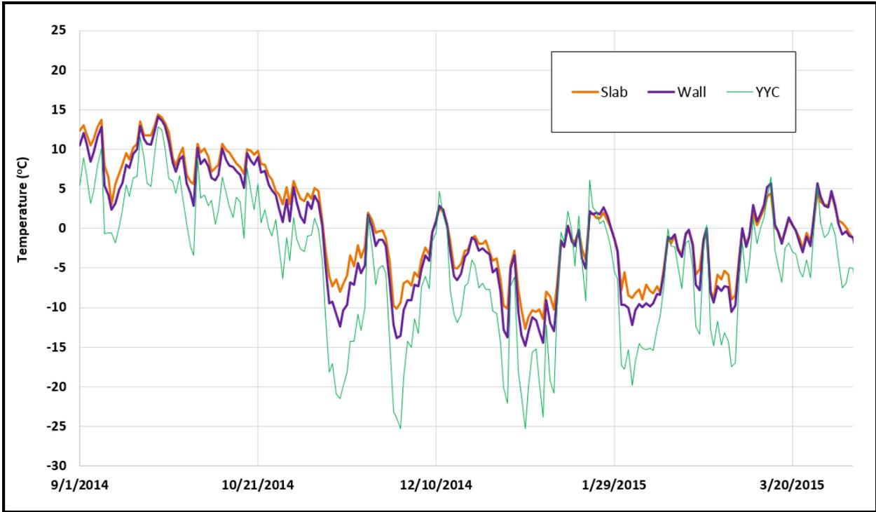
**Figure 9. Average of Minimum Temperatures at Slab and External Wall Surfaces**
