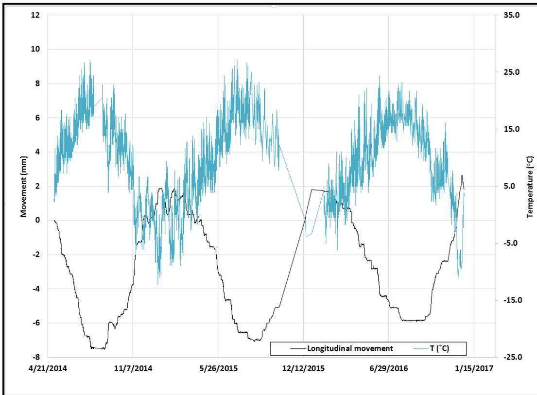
Figure 18. Longitudinal Movements
