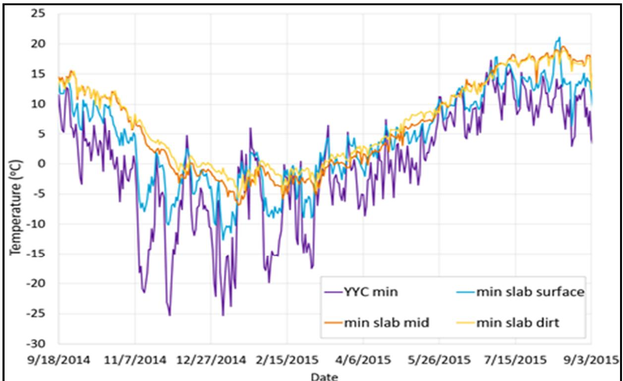
**Figure 8. Average of Minimum Temperatures at Different Locations through the Depth of the Slab**
