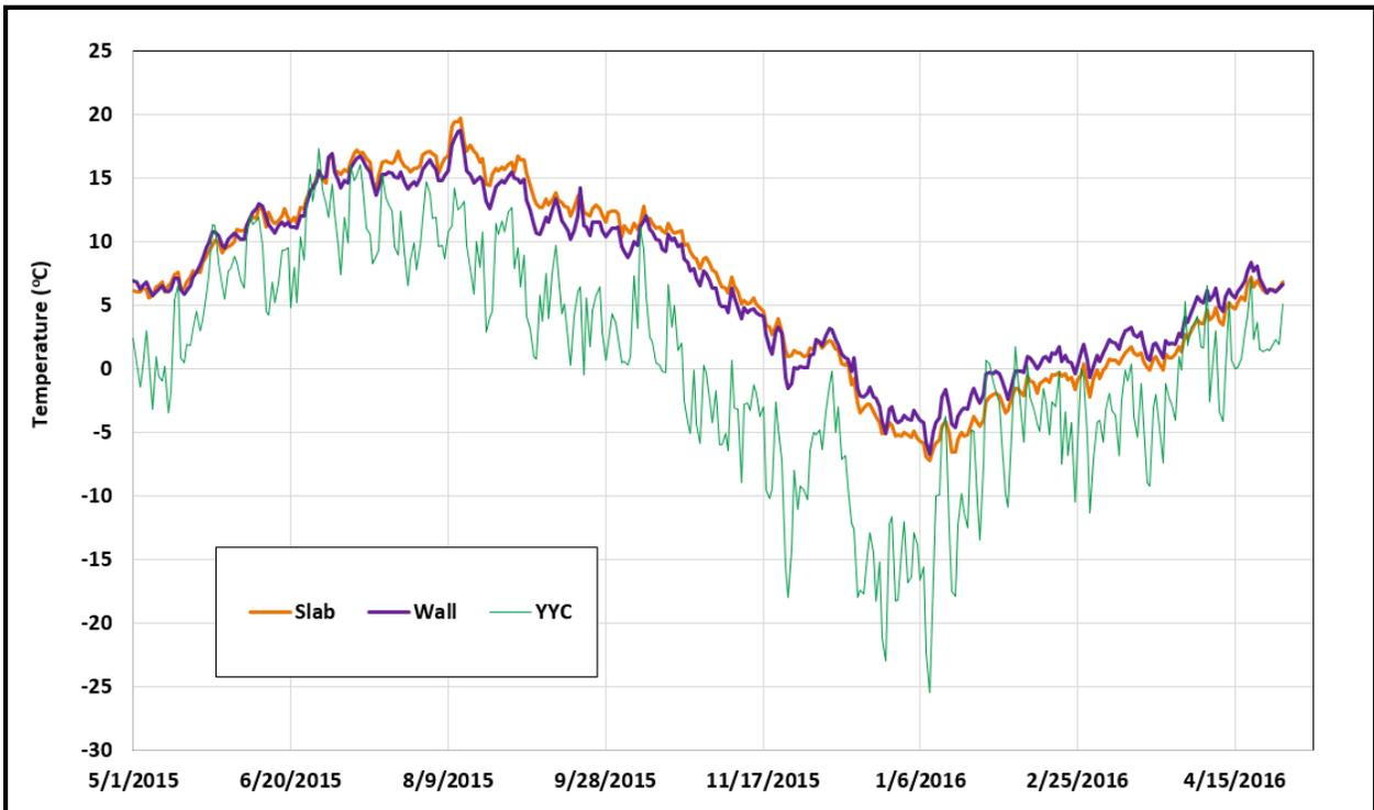
**Figure 12. Average of Minimum Temperatures for all Wall or Slab Sensors**
