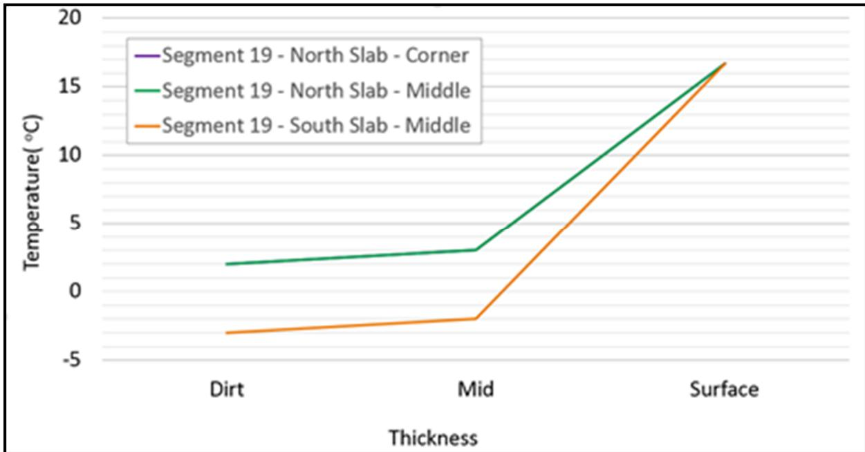
Figure 15. Temperature Distribution along Depth of Section for a Positive Temperature Differential
