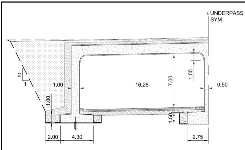
Figure 2. Typical Tunnel Section
