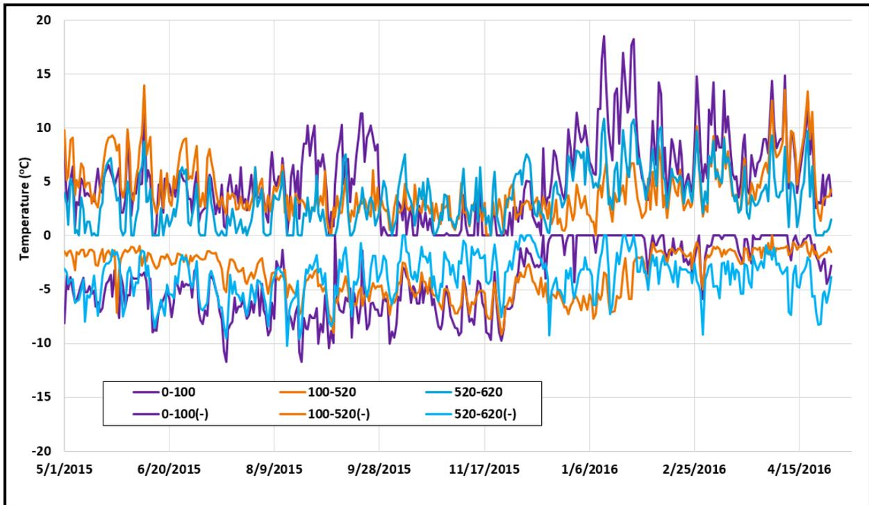
**Figure 13. Average of Temperature Differentials between Surface and Dirt Levels for the Slab**
