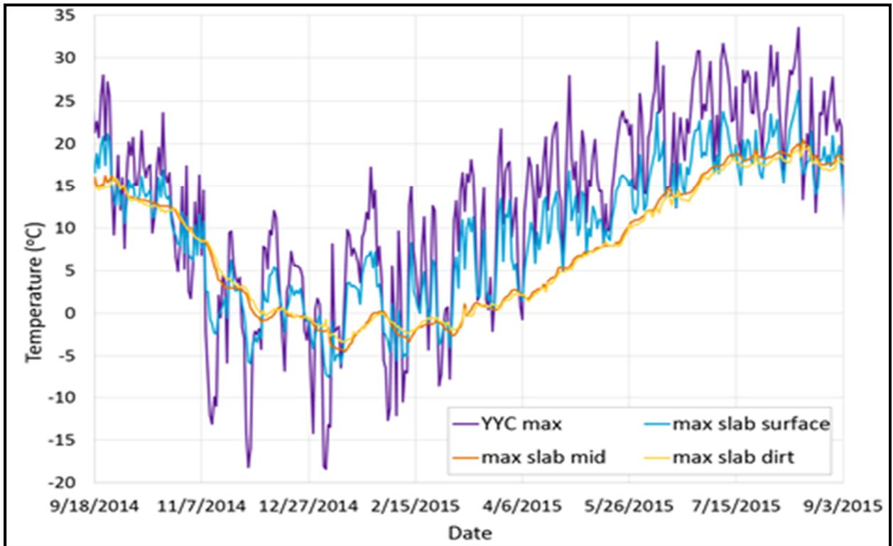
**Figure 7. Average of Maximum Temperatures at Different Locations through the Depth of the Slab**
