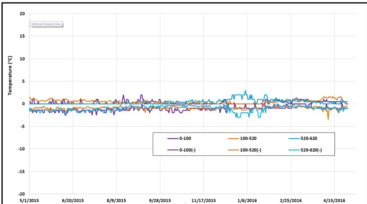
**Figure 14. Average of Temperature Differentials between Mid-depth and Dirt Level for the Slab**
