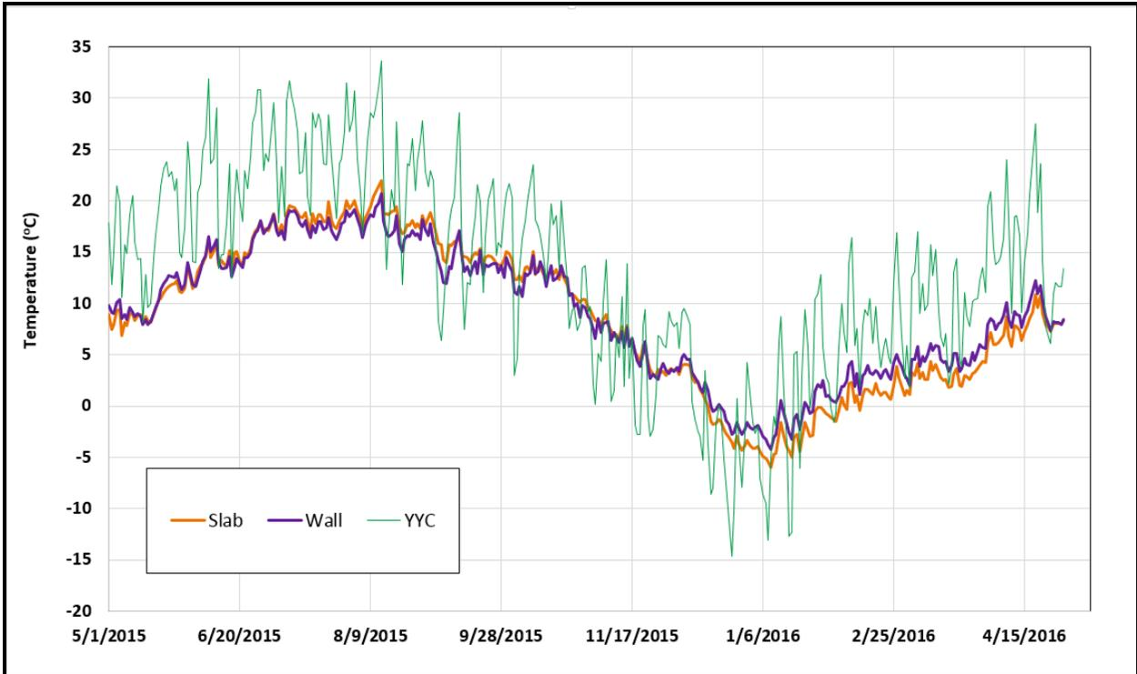
**Figure 11. Average of Maximum Temperatures for all Wall or Slab Sensors**
