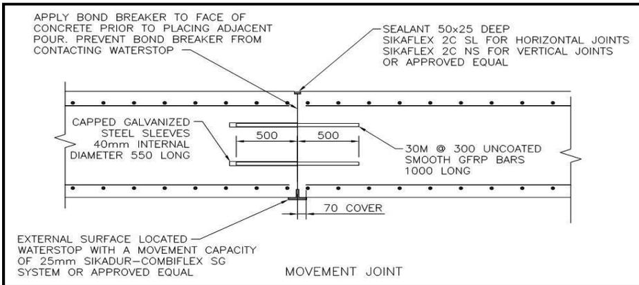
Figure 3. Movement Joint Details
