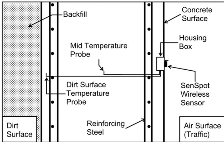
**Figure 5. Typical Cross-section through Tunnel Wall Showing SenSpot™ Sensor and Probes**
