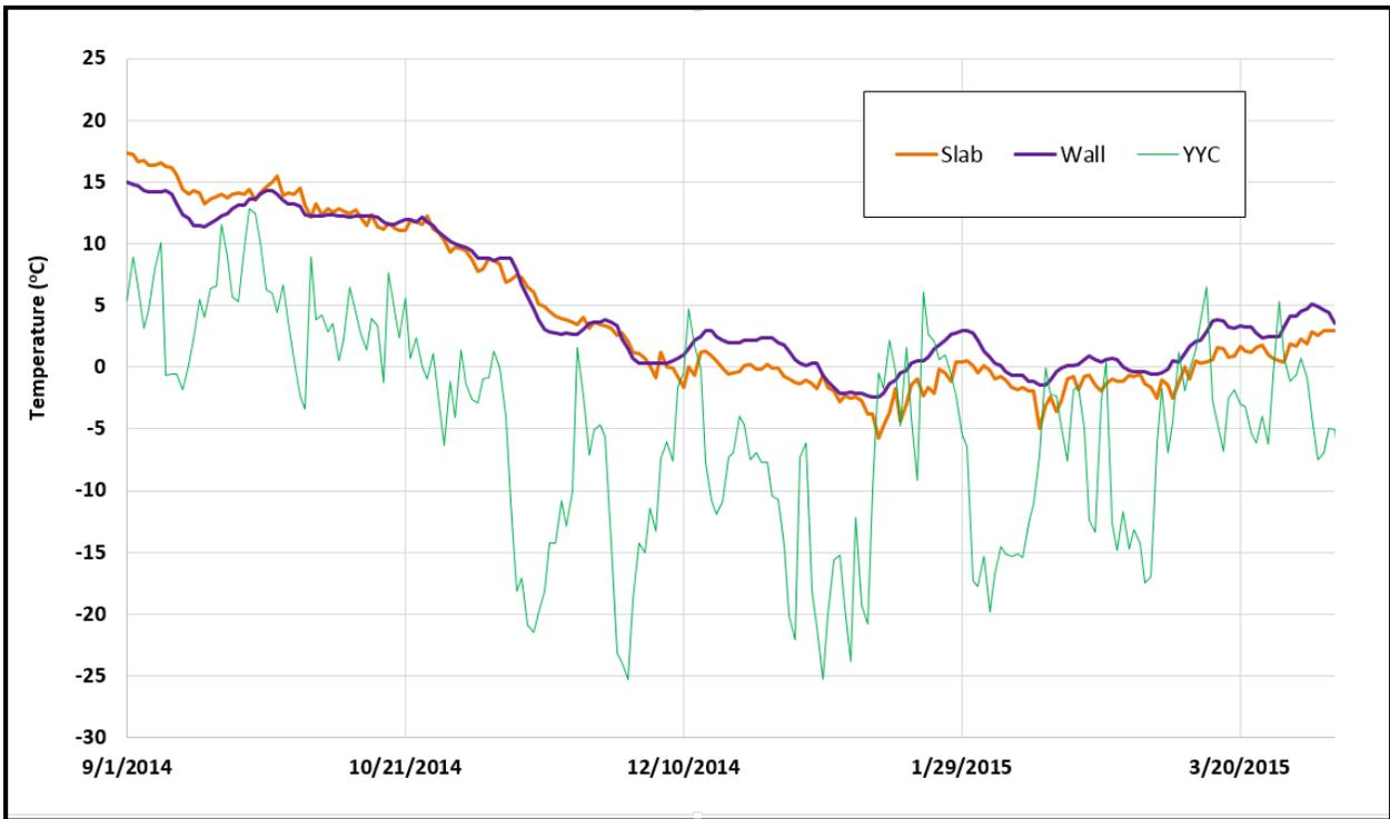
**Figure 10. Average of Minimum Temperatures at Slab and External Wall, Dirt Side**
