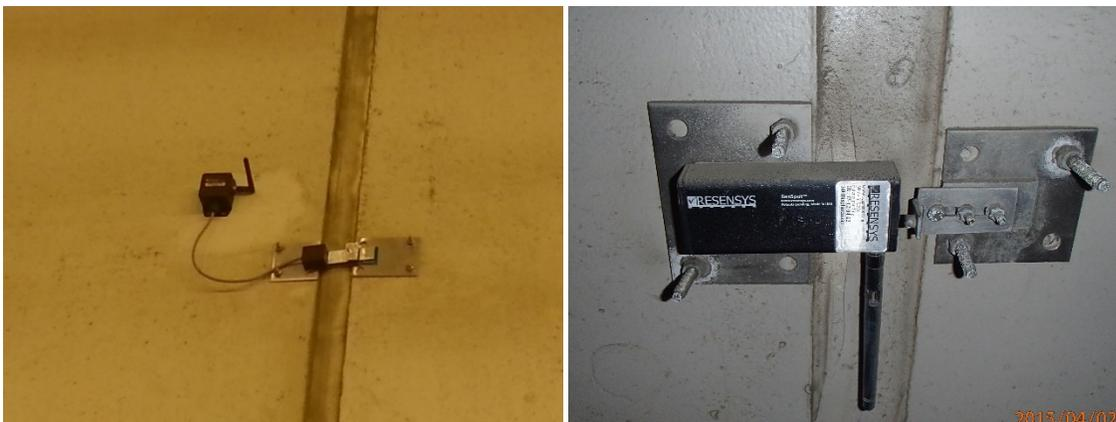
**Figure 6. Installation of the 1D and 3D Displacement Sensors**
