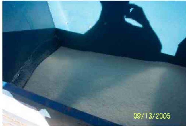
Figure 3 Sasobit – Prill Form Used for the Trial
