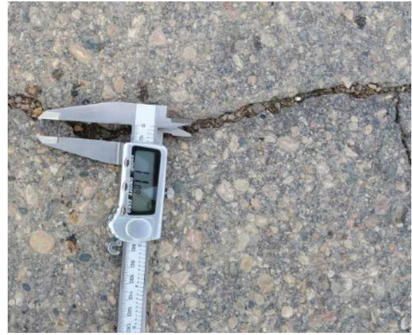
Figure 18 & 19: Crack widths measured using Automotive Brake Gauges (left) and digital calipers (right)
