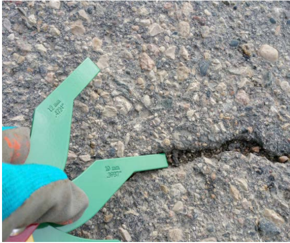
Figure 18 & 19: Crack widths measured using Automotive Brake Gauges (left) and digital calipers (right)
