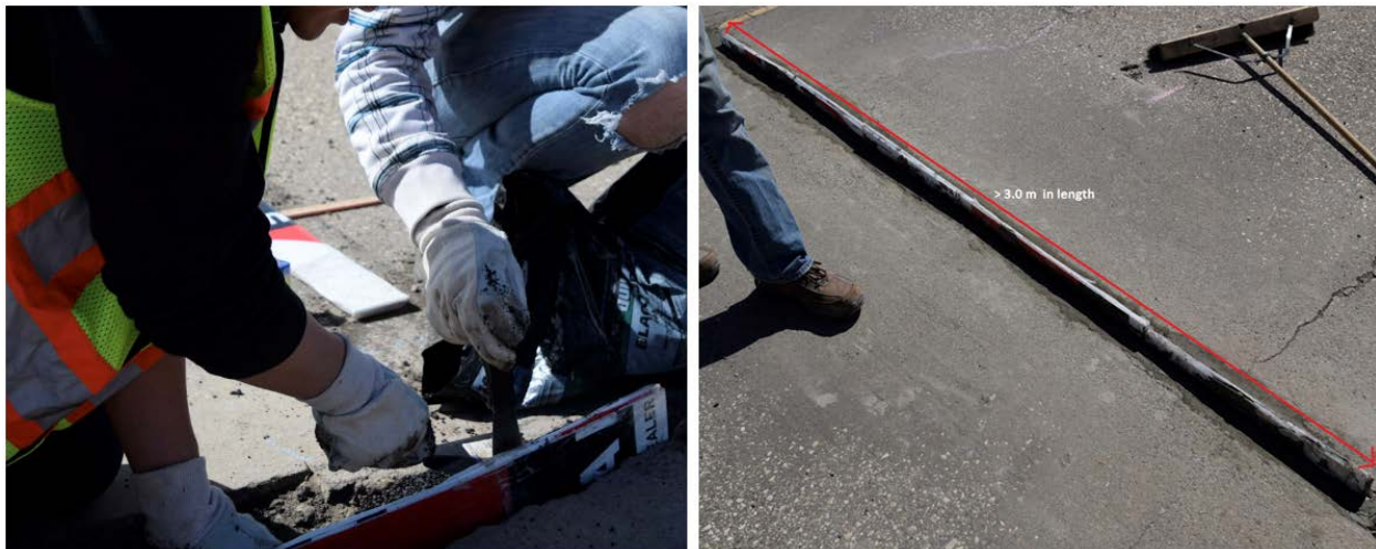
Figure 6: Manually Creating a Severe Transverse Crack (left) & Finished Transverse Crack (right)
