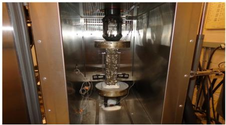
Figure 2: Typical TSRST Test Setup
