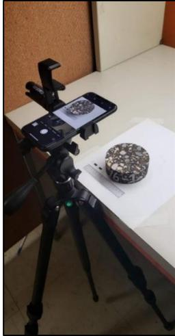
**Figure 7.** Digital camera imaging set-up.
