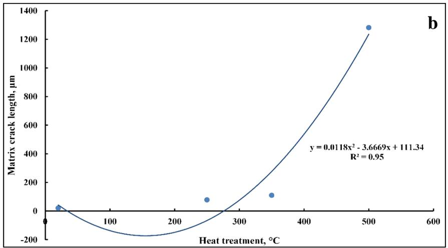
Figures. 19: Behavior of matrix cracks properties through heat treatment:- a: width, b: length
