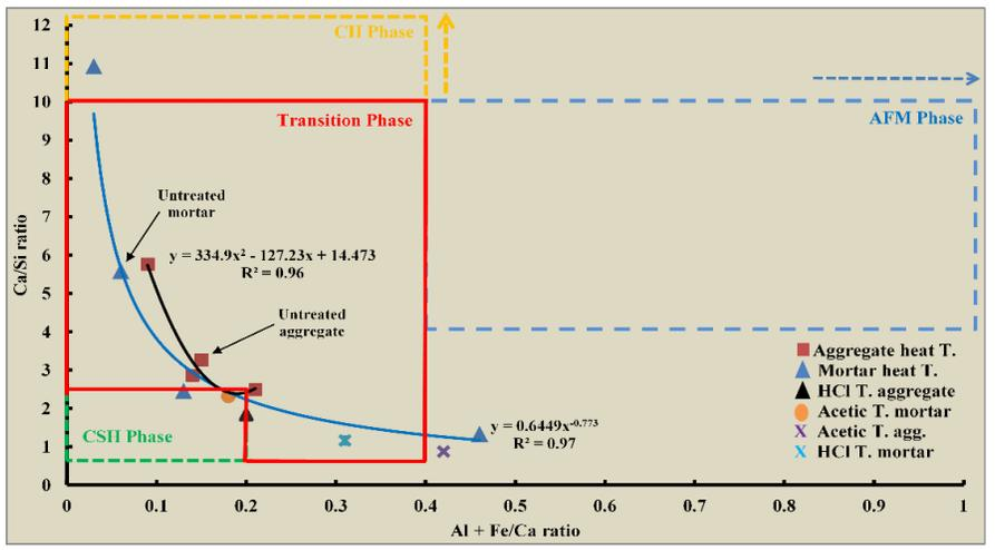
Figure 11: Intermix phases to mortar and aggregate of CRCA through heat treatment
