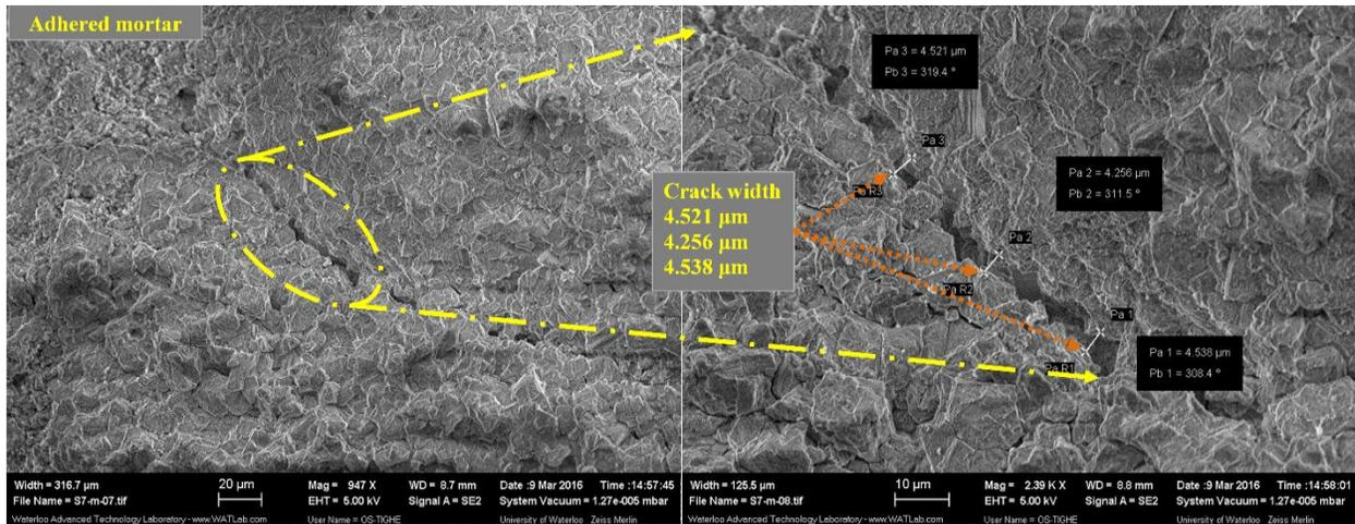
Fig. 25: Matrix cracks on mortar surface through C<sub>2</sub>H<sub>4</sub>O<sub>2</sub> treatment
