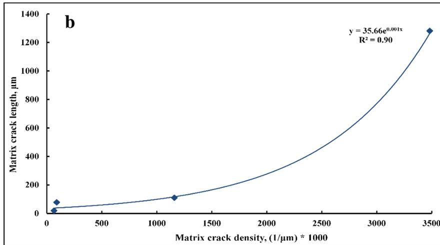
Figure 27: Relationship between matrix crack density and cracks properties:- a: width, b: length
