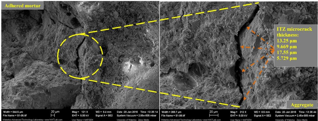
Figure 4: ITZ microcrack width to CRCA through heat treatment at 250°C
