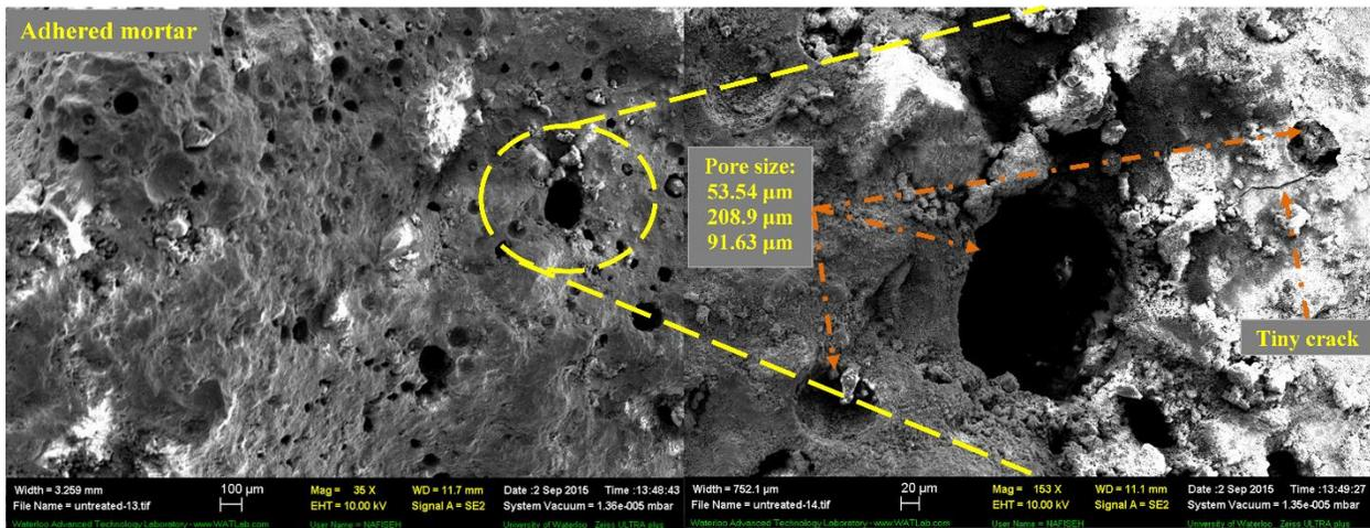
Figure 13: Pore size of mortar surface to untreated CRCA
