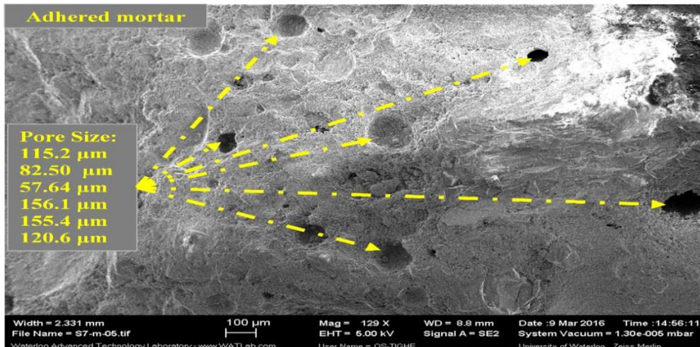
Figure 18: Pore size of mortar surface to CRCA through C<sub>2</sub>H<sub>4</sub>O<sub>2</sub> treatment
