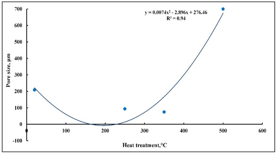
Figure 12: Pore size behavior through heat treatment
