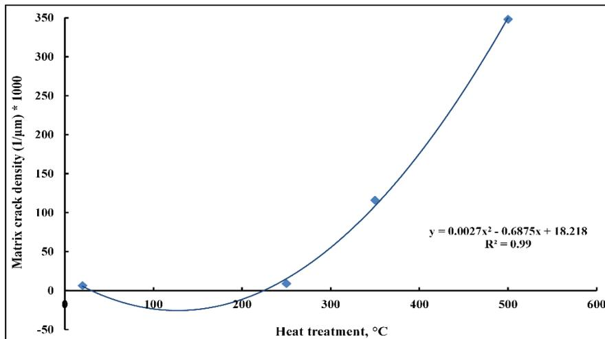
Figure 26: Behavior of matrix crack density through heat treatment
