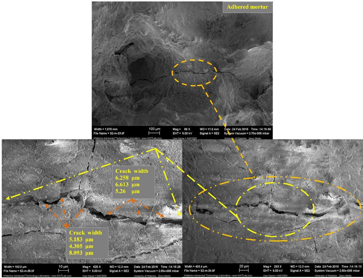
Figure 23: Matrix cracks on mortar surface through heat treatment at 500°C
