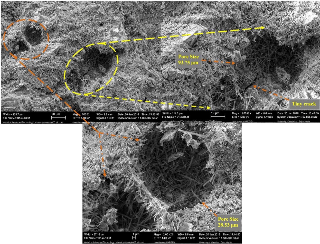
Figure 14: Pore size of mortar surface to CRCA through heat treatment at 250°C
