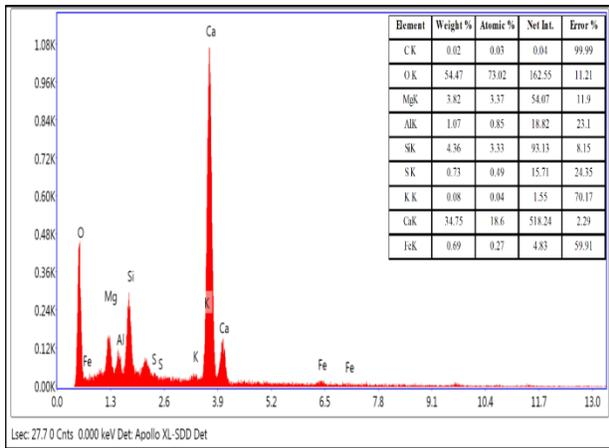
Fig. A2-a: EDAX of untreated mortar surface
