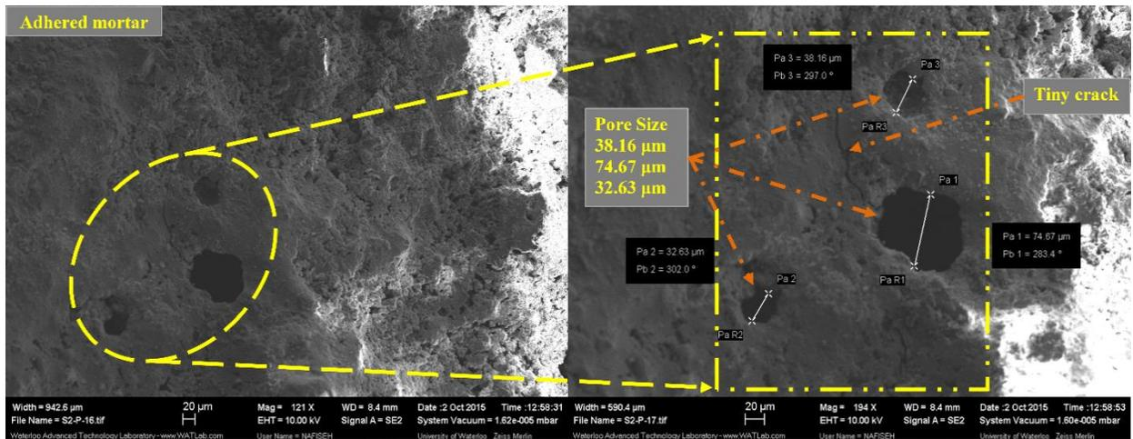
Figure 15: Pore size of mortar surface to CRCA through heat treatment at 350°C
