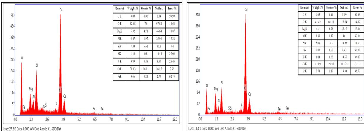
Fig. A1-c: EDAX of aggregate surface at 350°C Fig. A1-d: EDAX of aggregate surface at 500°C
