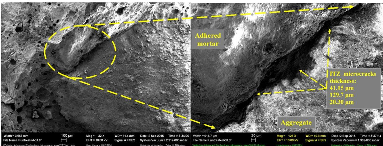
Figure 3: ITZ microcrack width to untreated CRCA
