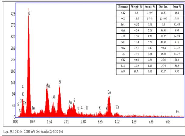
Fig. A1-e: EDAX aggregate surface HCl T.
