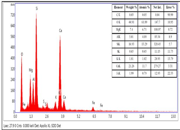
Fig. A1-f: EDAX aggregate surface acetic T.
