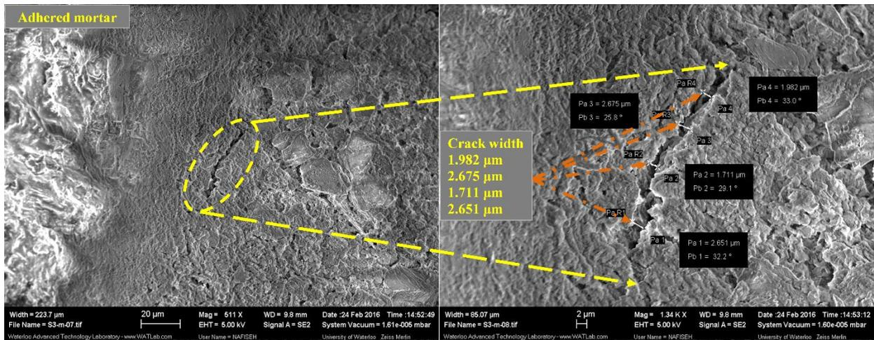
Figure 24: Matrix cracks on mortar surface through HCl treatment
