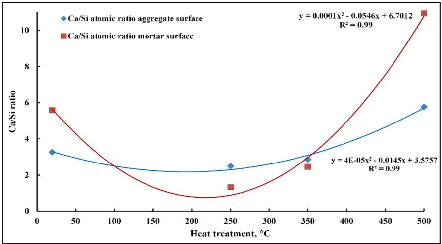
Figure 10: Ca/Si atomic ratio for aggregate and mortar surface through heat treatment
