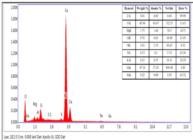
Fig. A2-d: EDAX of mortar surface at 500°C
