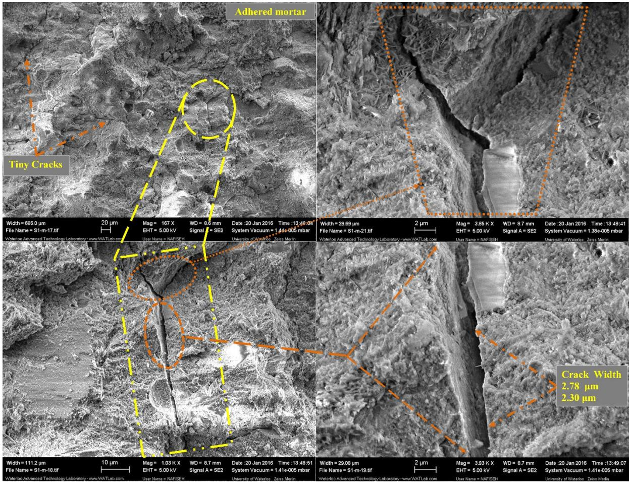
Fig. 21: Matrix cracks on mortar surface through heat treatment at 250°C
