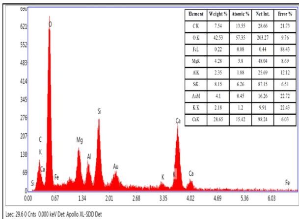
Fig. A2-c: EDAX of mortar surface at 350°C
