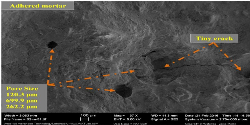
Figure 16: Pore size of mortar surface to CRCA through heat treatment at 500°C
