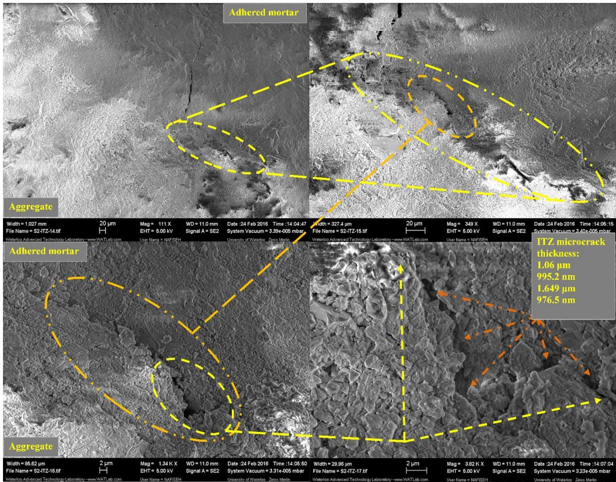
Figure 6: ITZ microcrack width to CRCA through heat treatment at 500°C
