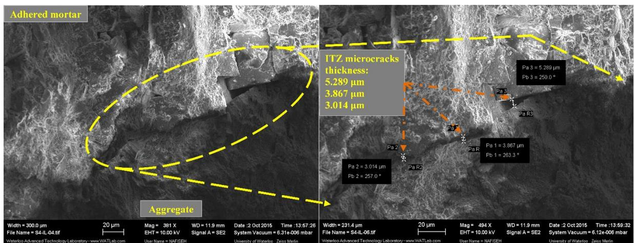
Figure 7: ITZ microcrack width to CRCA through acidic treatment with HCl
