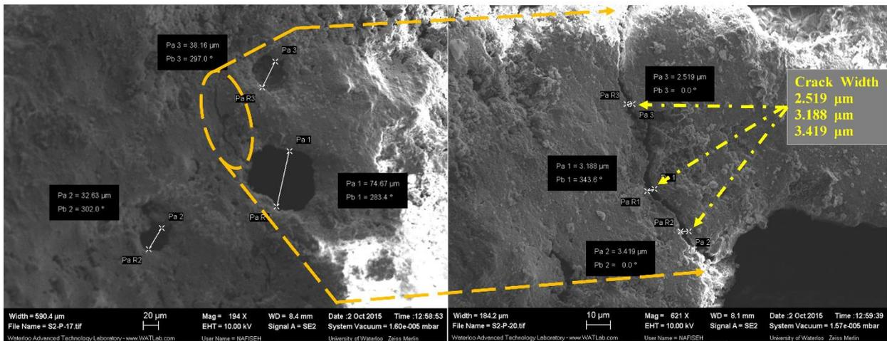
Figure 22: Matrix cracks on mortar surface through heat treatment at 350°C
