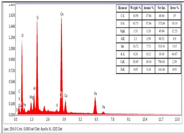
Fig. A2-b: EDAX of mortar surface at 250°C
