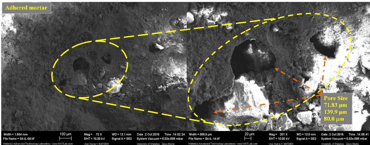
Figure 17: Pore size of mortar surface to CRCA through HCl treatment
