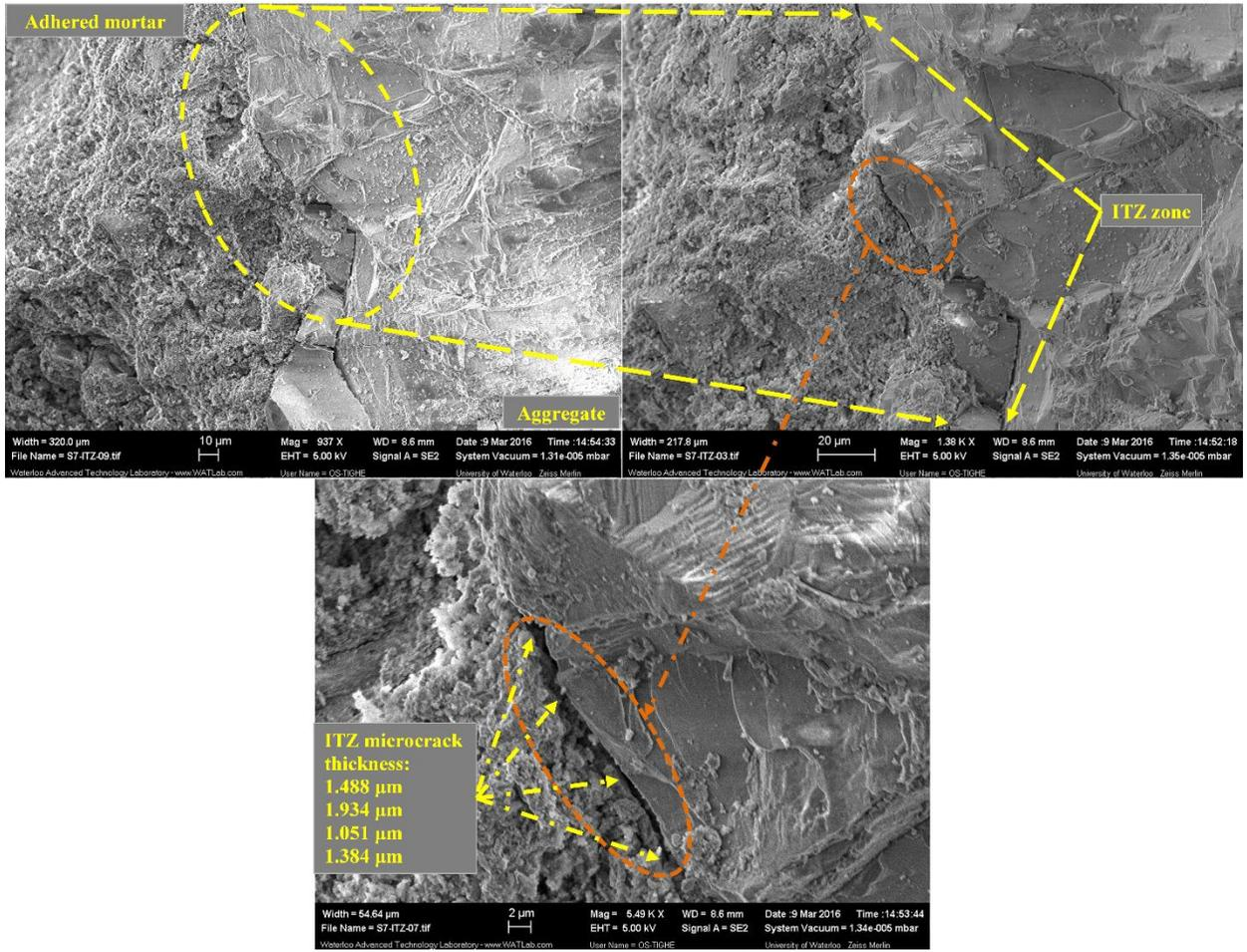
Figure 8: ITZ microcrack width to CRCA through acidic treatment with  $C_2H_4O_2$
