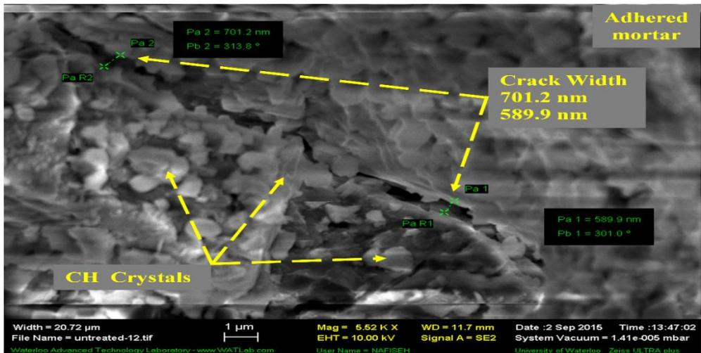
Figure 20: Matrix cracks on mortar surface to untreated CRCA
