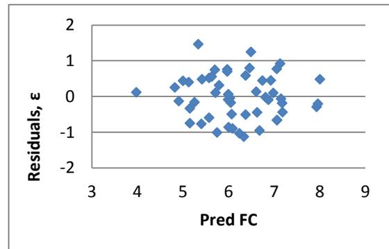
Figure 6: Residual Plot for Alligator damage with 4<sup>th</sup> Set of Parameter ( $\beta_{f1} = 1.0$ ,  $\beta_{f2} = 0.7$ ,  $\beta_{f3} = 0.7$ )
