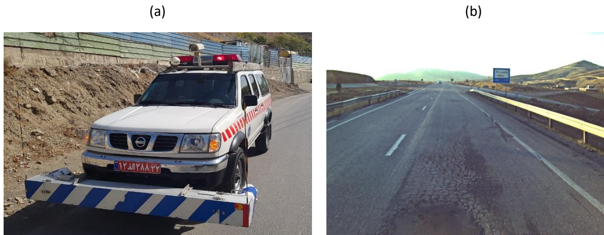
Fig. 1(a). Road Surface Profiler mounted on a vehicle, (b). Forward view image captured by the camera placed on the vehicle's roof
