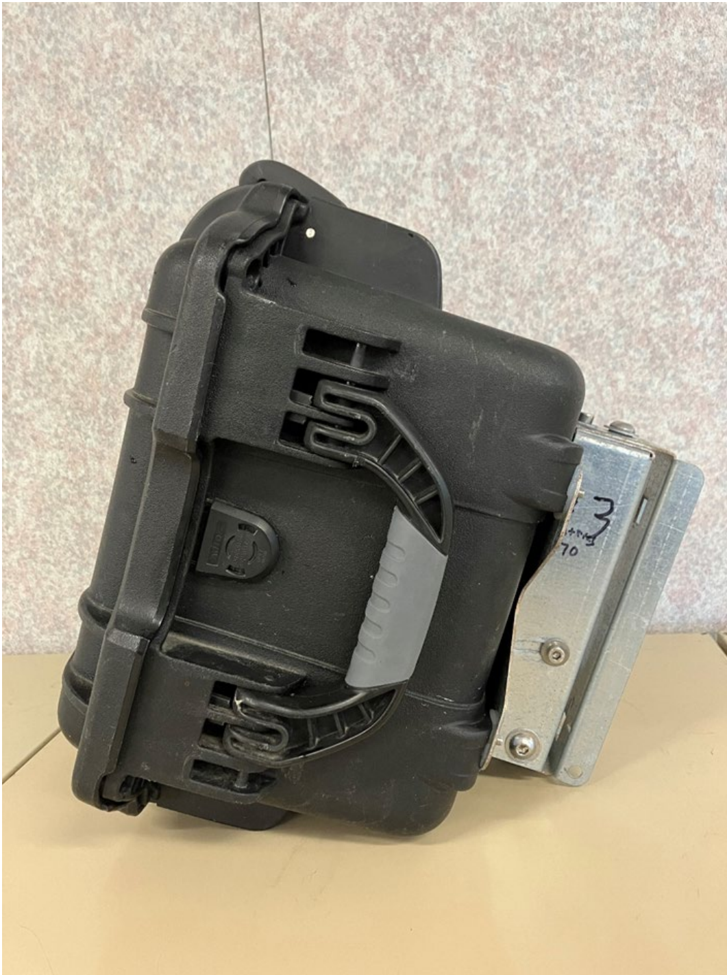
Figure 1: Radar Traffic Counter exterior view
