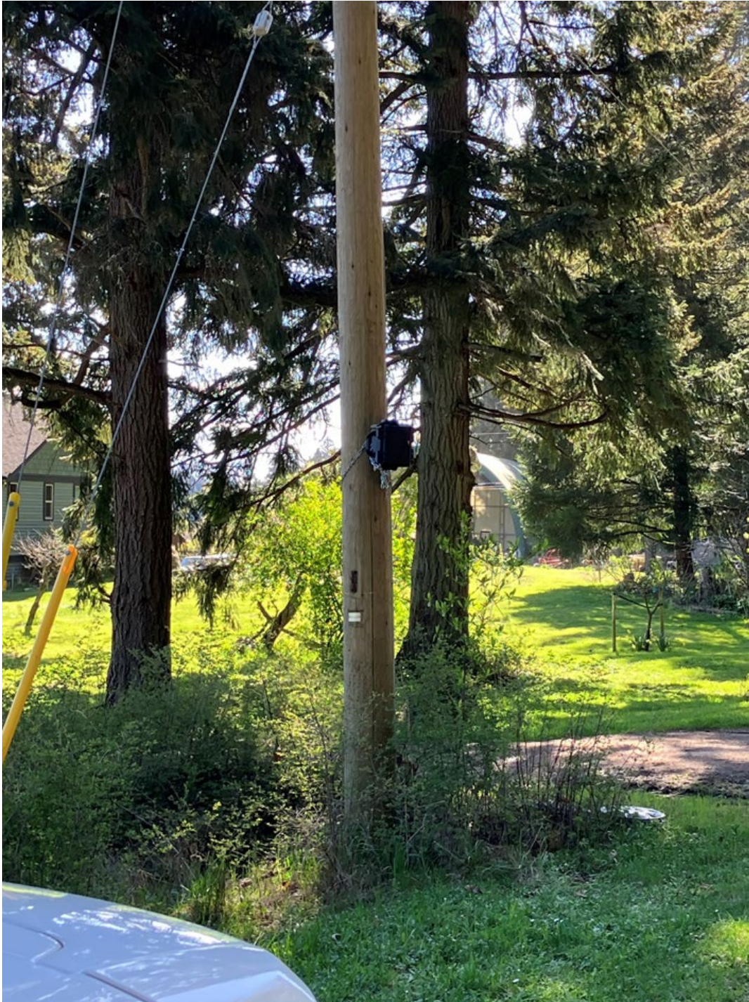
Figure 7: Radar traffic counter deployed on a side road for speed surveying.
