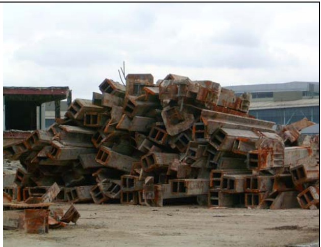
Figure 8: Plate and Structural (P+S) Scrap Steel
