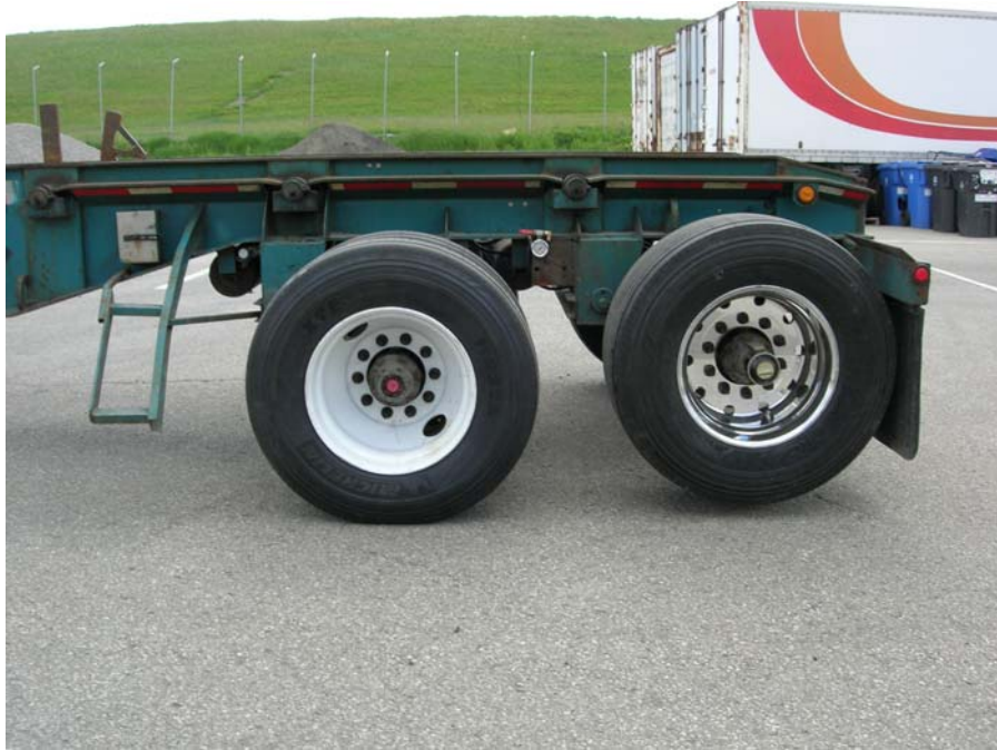
Figure 3 Liftable dual axles for testing dual and SWB tires
