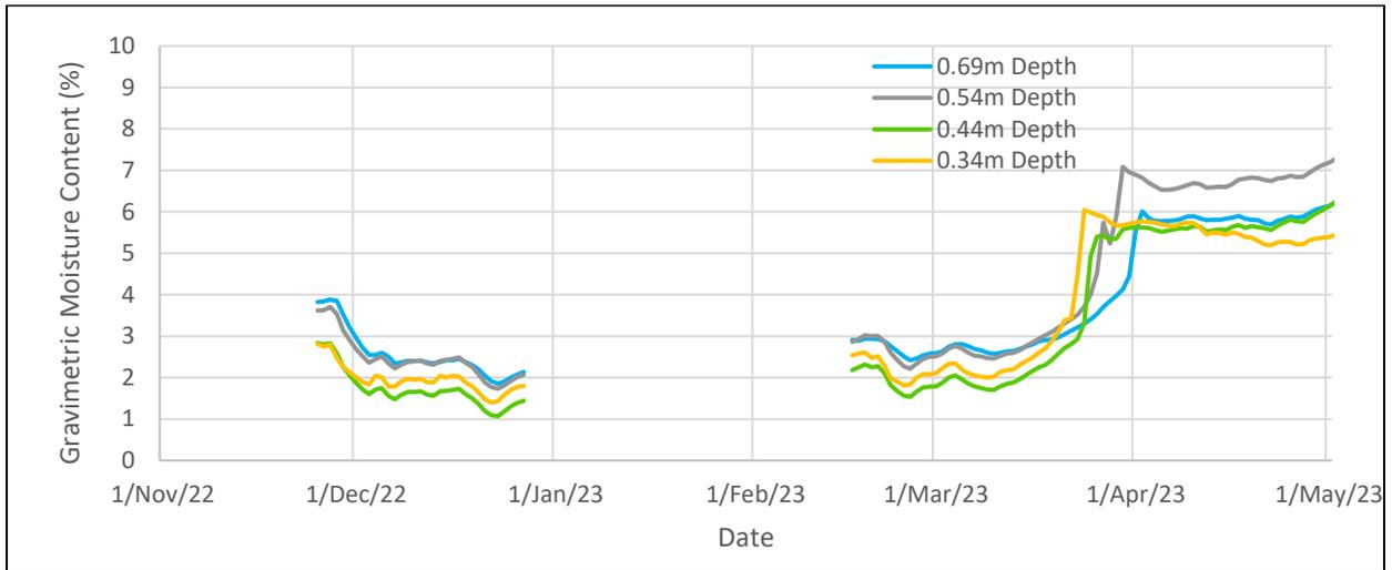
Figure 10: 150mm Geocell gravimetric moisture content profile (2023-2024 winter)
