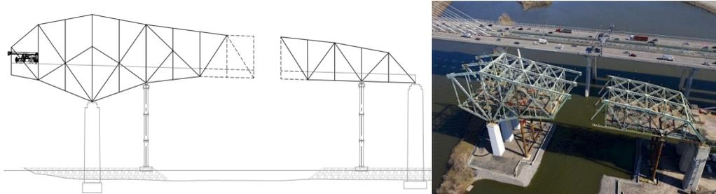
Since it was not possible to deconstruct the bridge by reversing its original construction sequence, the new sequence induced new forces in the members for which they were not designed for originally. A global model integrating all the different construction stages was developed. Some stages of the model are shown in Figure 24.
