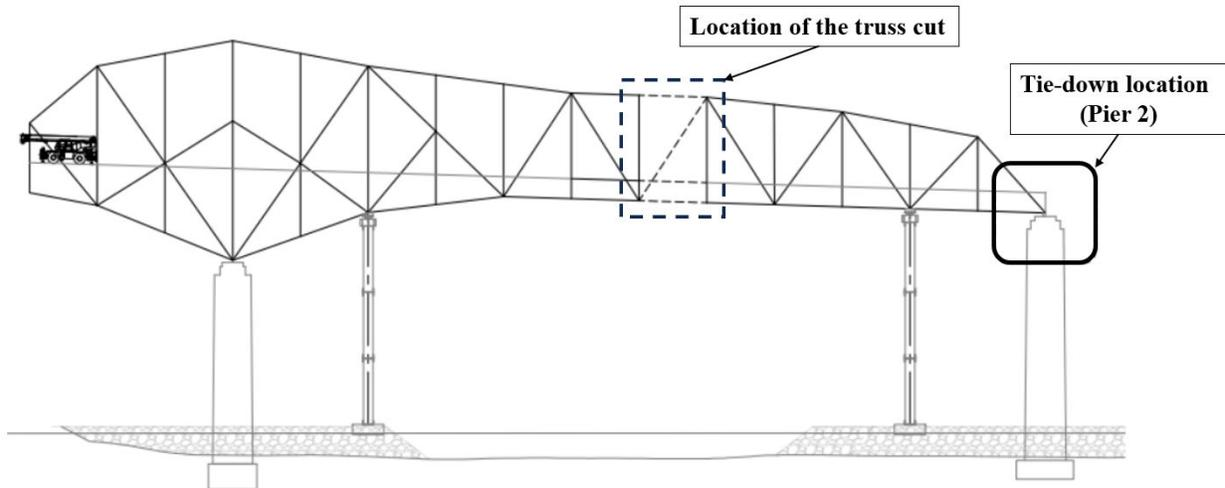
The bridge was now separated into two independent halves. Each of the half was supported on a pier and a temporary support tower.
