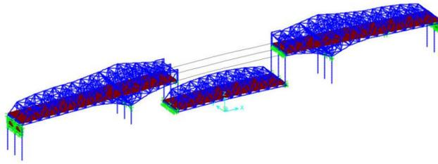
Figure 16. Local structural analysis model for the deconstruction of the suspended span on the barge
