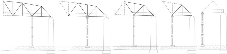
The distinctive feature of the half supported by pier 1 was related to its sequence of the deconstruction. The removal sequence of the members had to minimize the asymmetry of the truss on either side of the pier and the temporary tower to reduce moment and the uplift at the pier. The sequence is shown on Figure 26.
