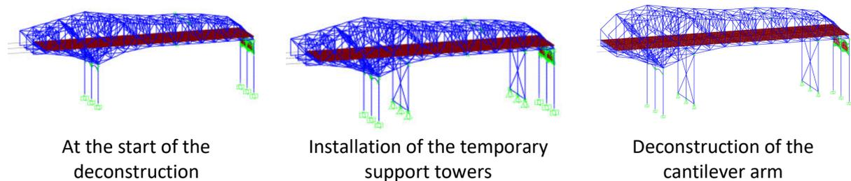
Following the detailed structural analysis, it was found that some members became overloaded during certain steps of the new sequence. The overloaded members were reinforced before starting the deconstruction process.
