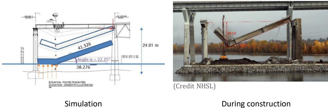
As depicted in Figure 12, the simulation accurately predicted the manner in which the girder would fall, validating the structural analysis conducted.
