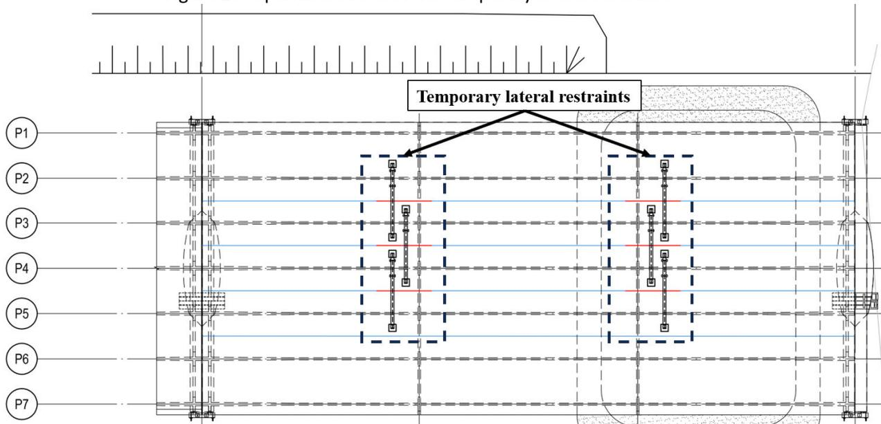
Another main challenge of this method was the resistance of the piers when the girders were being dropped. The method involved cutting the girder at approximately one third of the span so that when it fell, it would break into two pieces, with one part hitting the piers. Analysis and simulations were performed to determine the most probable fall trajectory resulting in the most critical forces on the piers. The projected trajectory of the girder's fall is shown in Figure 11.
