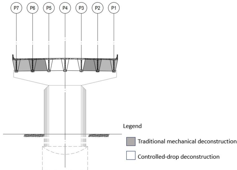
Unlike the controlled drop method used for the other spans of Section 7, the girders were not longitudinally cut before being dropped ensuring no issue with their lateral stability. Additionally, due to the lower height of fall for the girders, no additional measures were required to protect the piers from impact.
