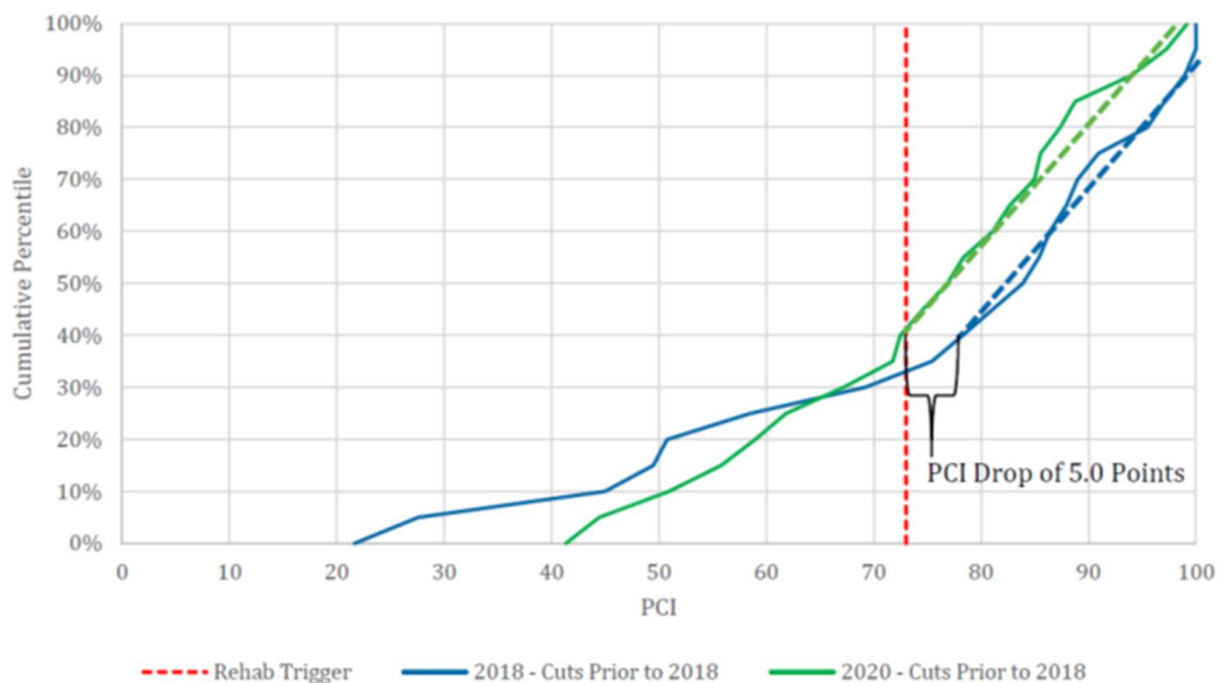
Figure 9. PCI Deterioration Trend for Dataset 2
