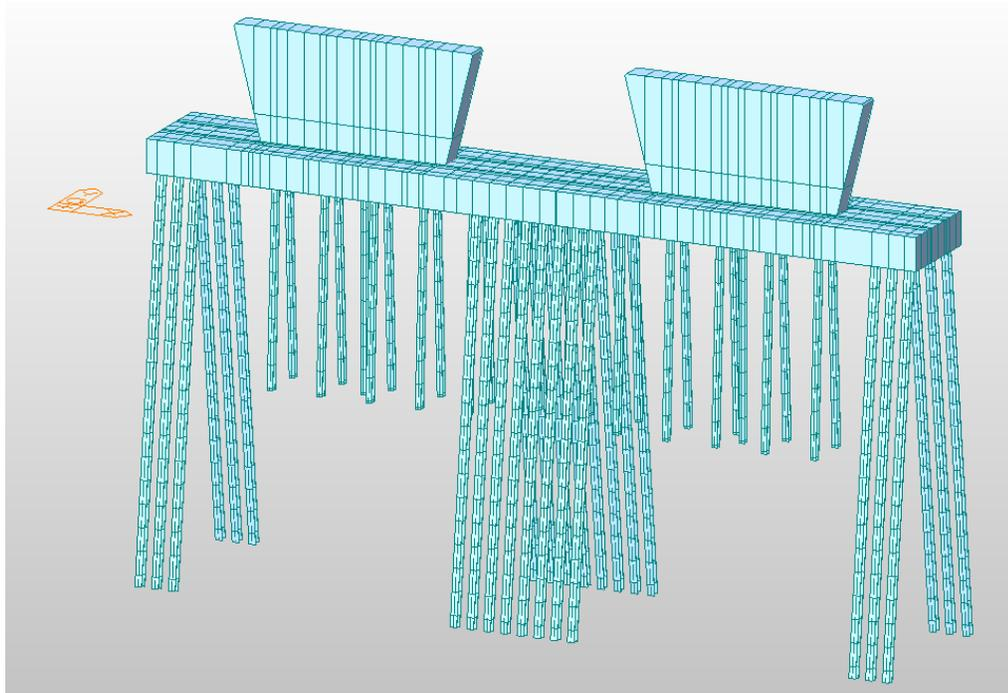
The final design, shown in Figure 12 and Figure 13, consisted of 28 piles placed at offsets around the existing pier. Spatial constraints of the existing bridge substructure and superstructure and the bridge rehabilitation construction being in-progress only permitted piles to be installed at the transverse edges of the pier and in between the carriageways. The piles are embedded into a new encasement pile cap that is 4.5 m wide by 1.5 m tall.
