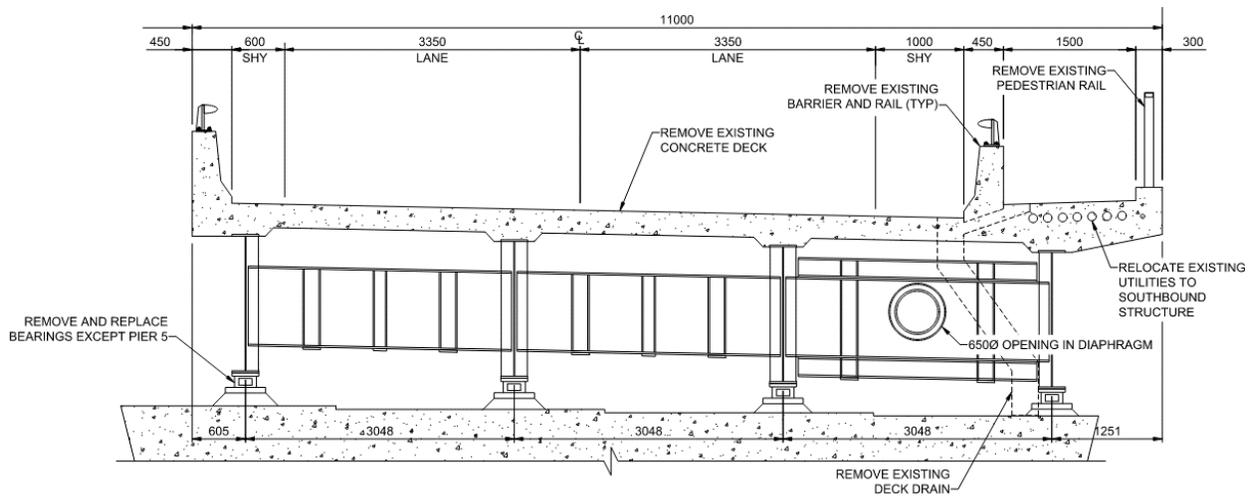
Figure 2: Bridge Half Cross Section Following Rehabilitation
