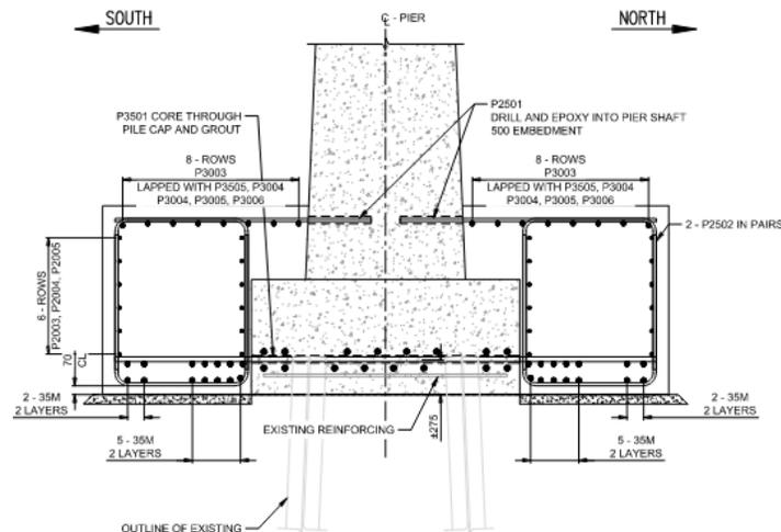
Figure 13: Foundation Underpinning Pile Layout
