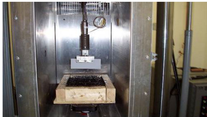
Figure 5. Blade resistance workability test apparatus from [19].
