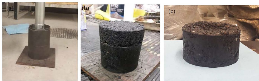
Figure 6. Procedure of the adhesiveness test: (a) CMA compaction on top of HMA, (b) sample extrusion, (c) weighing the remnants after inverting the sample and measuring the separation time from [19].
