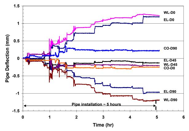
Figure 7: Open cut HDPE installation ring deflections.
