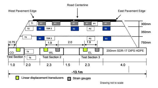
Figure 5: Open trench pipe installation test section and instrumentation locations
