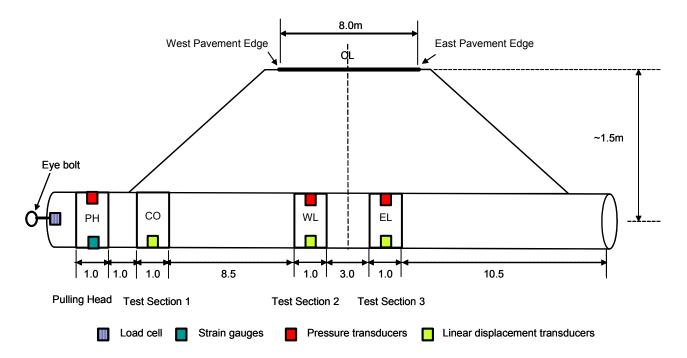
Figure 3: Layout of the 20 sensors placed inside the HDD installed pipe.
