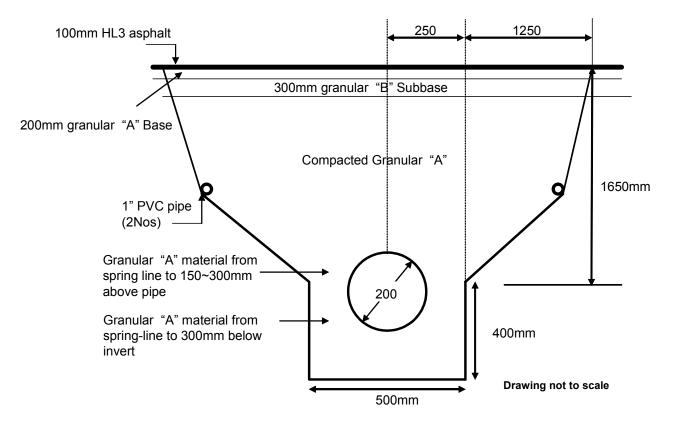
Figure 4: Open cut trench construction geometry and pipe location.
