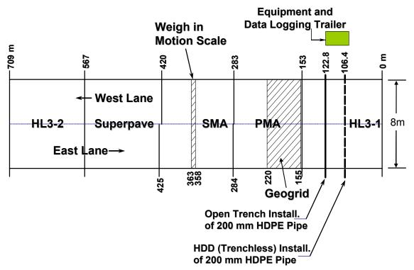
Figure 2: Test track layout.
