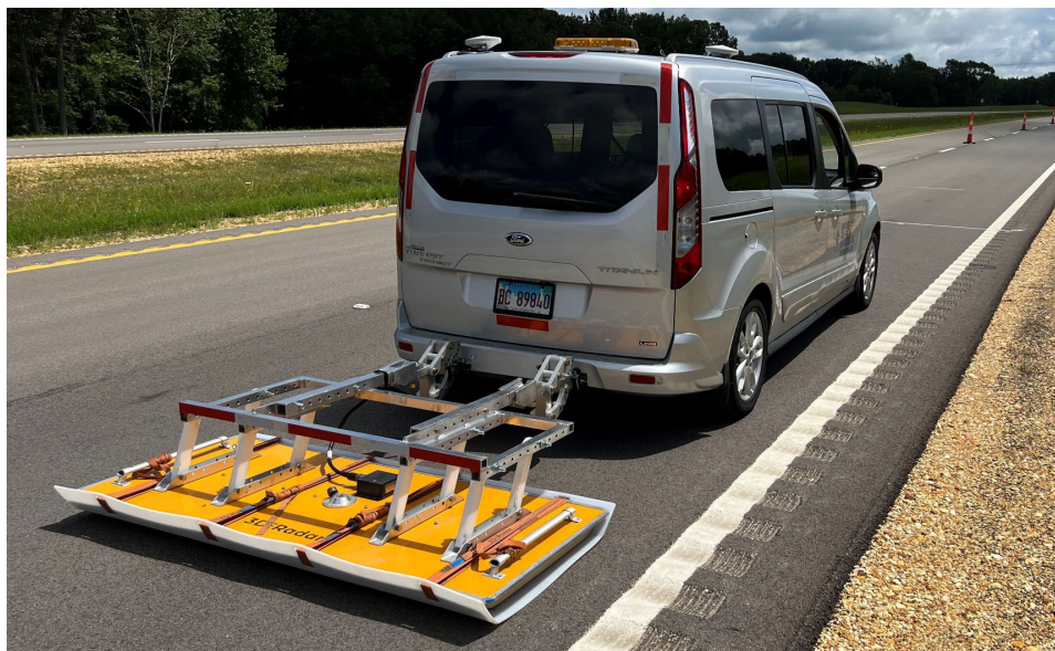
Figure 8: 3D-GPR Ground Coupled Antenna Mounted to Data Collection Vehicle
