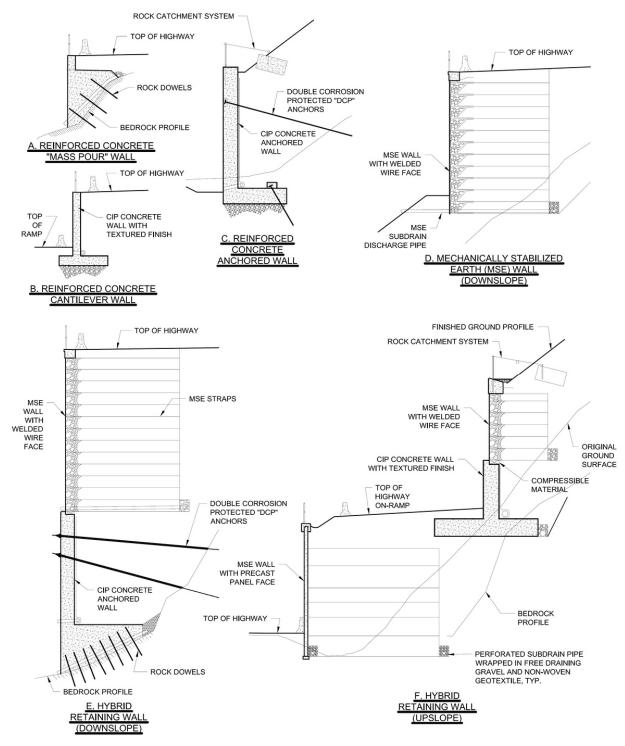
Figure 22 – Typical Retaining Wall Combinations
