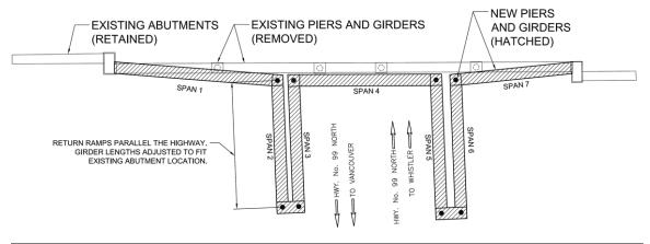
Figure 21 – Garibaldi Pedestrian Overpass - Bridge Layout
