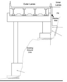
Figure 25 - Typical Half-Bridge Cross-Section (6900 Structure)
