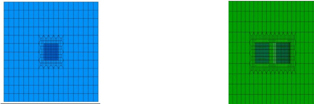
Figure 3. Schematic plan view of FEM meshes for (left) single tires and (right) dual tires. Shaded zones indicate tire contact patch(es).
