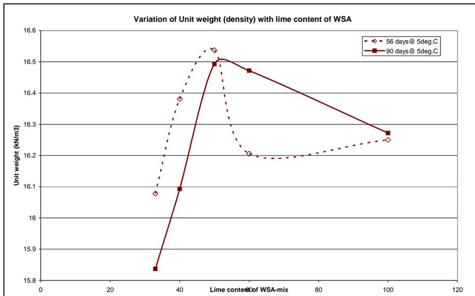
Fig. 4: Variation of sample unit weight with lime content of the lime-WSA mixture
