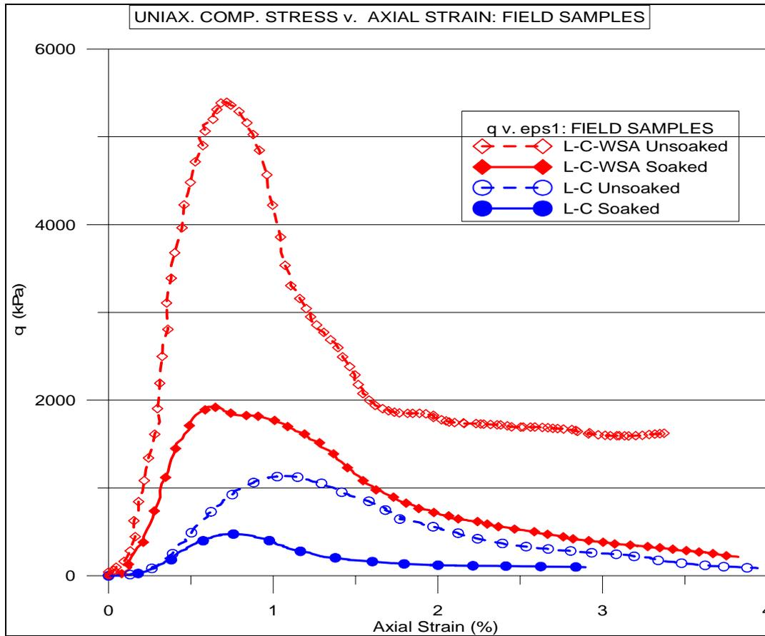
Fig. 9: Stress-strain curves for uniaxial compression of stabilized field samples
