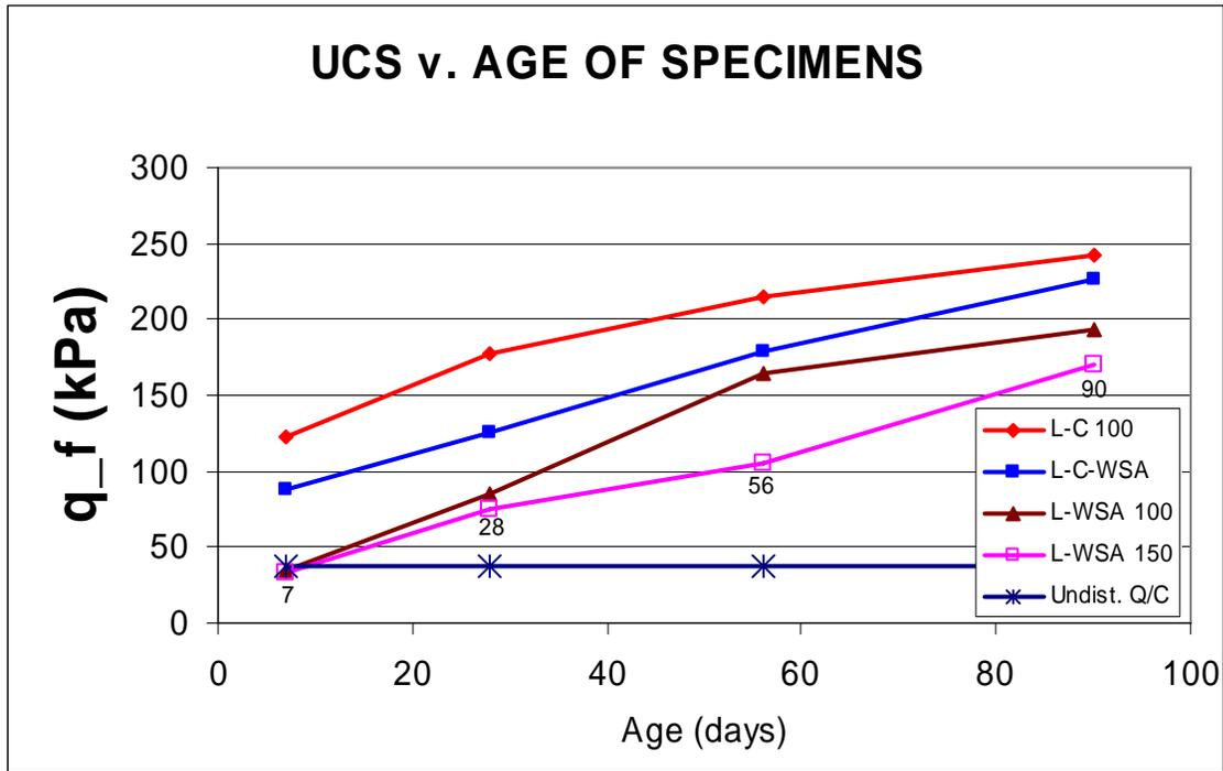
Fig. 5: Variation of compressive strength with sample curing period
