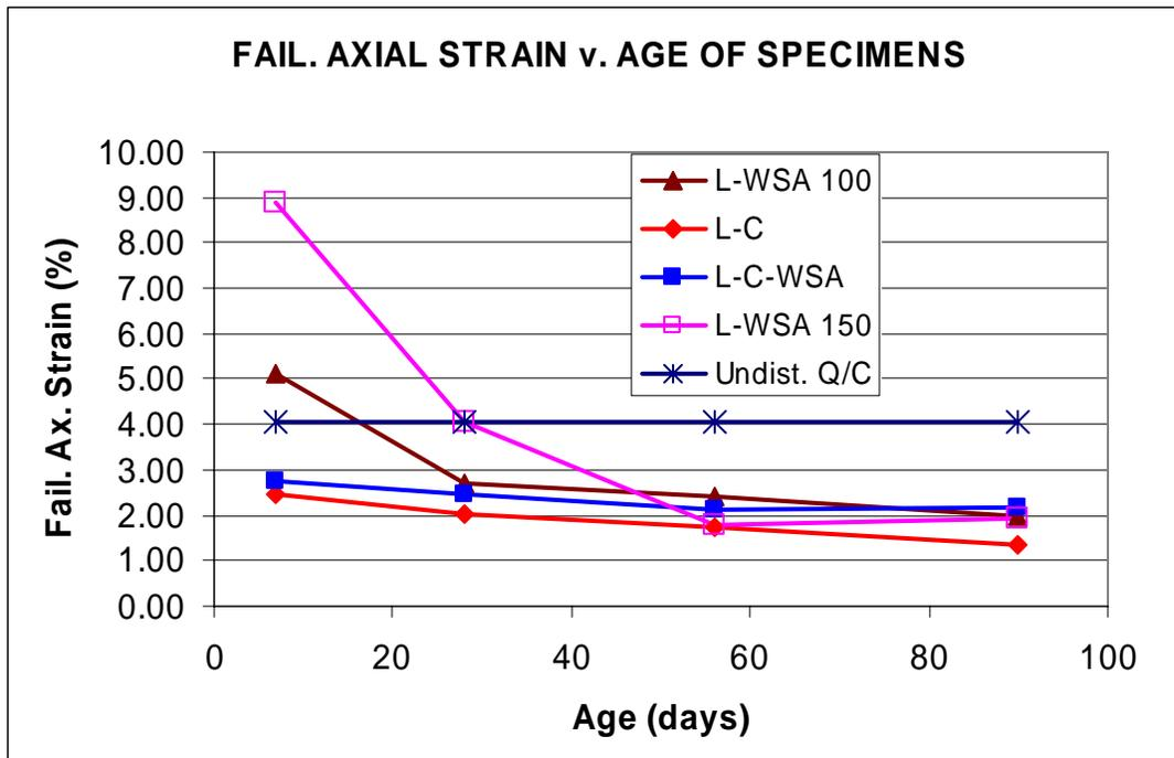
Fig. 8: Variation of the failure axial strain with sample curing period
