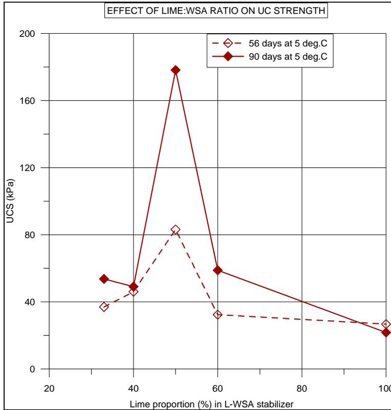
Fig. 3: Variation of uniaxial compressive strength with lime content of lime-WSA mixture
