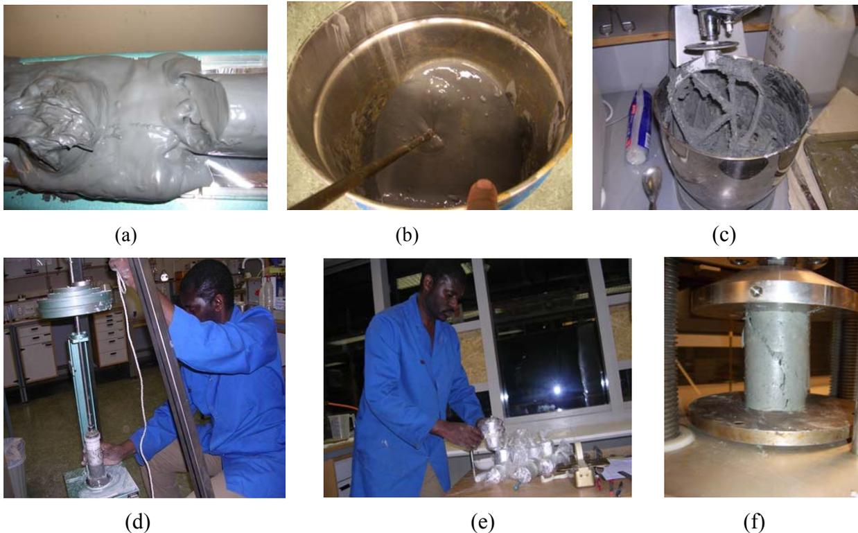
Fig. 1: Preparation of deep-mix laboratory samples: (a) Extrusion of quick clay from sampling cylinder; (b) Homogenization of natural clay; (c) Mixing of quick clay and binder materials; (d) Compaction of the mixture in cylindrical moulds; (e) Wrapping and labeling (f) Uniaxial compression test on lab specimen
