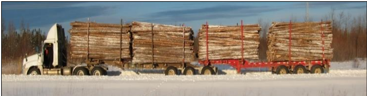
Figure 2. 72.5-tonne tandem-drive 9-axle log hauling configuration
