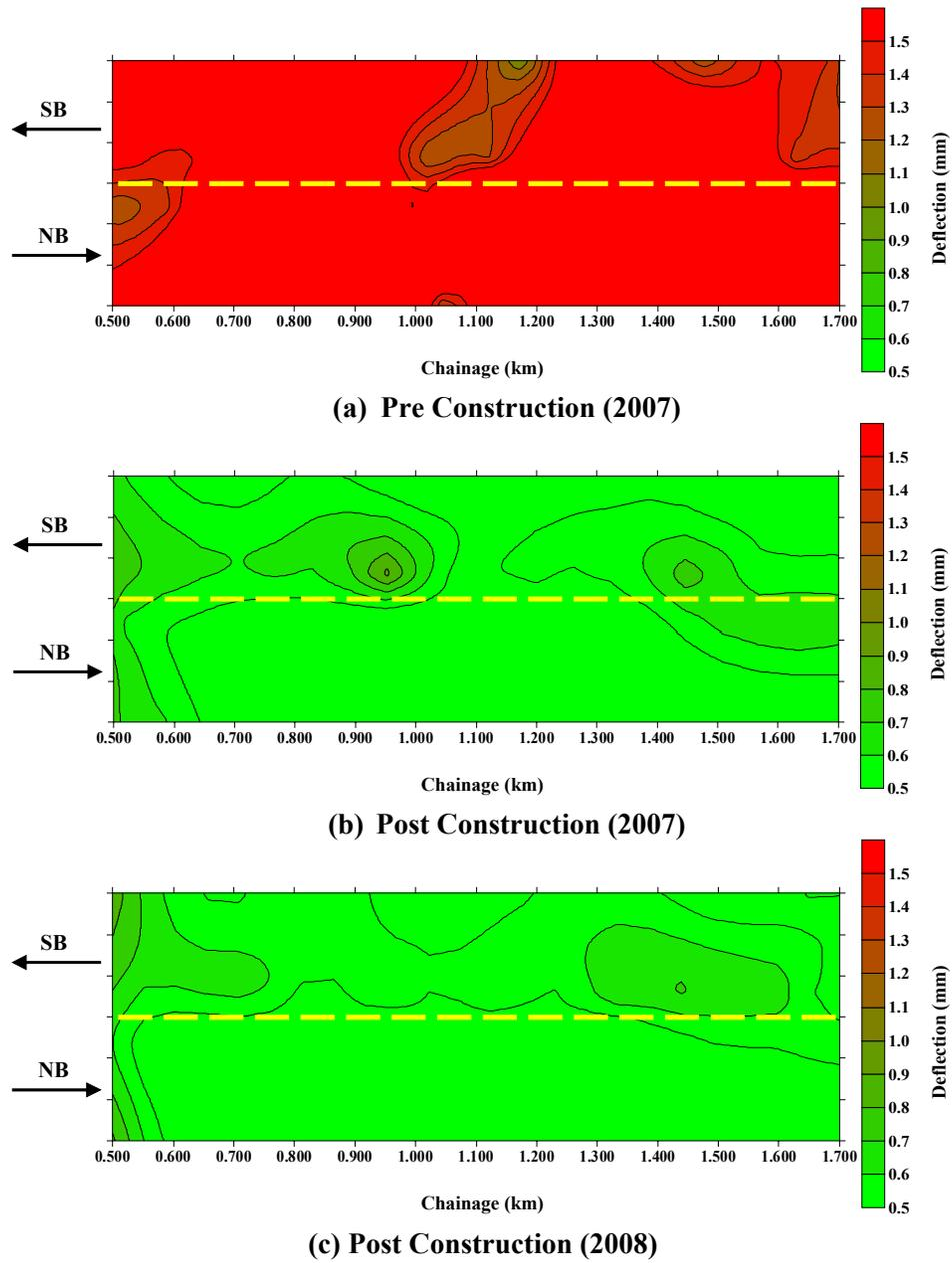
**Figure 9** Idylwyld Service Road Peak Surface Deflection Profiles at Primary Weight Limit + 50 %
