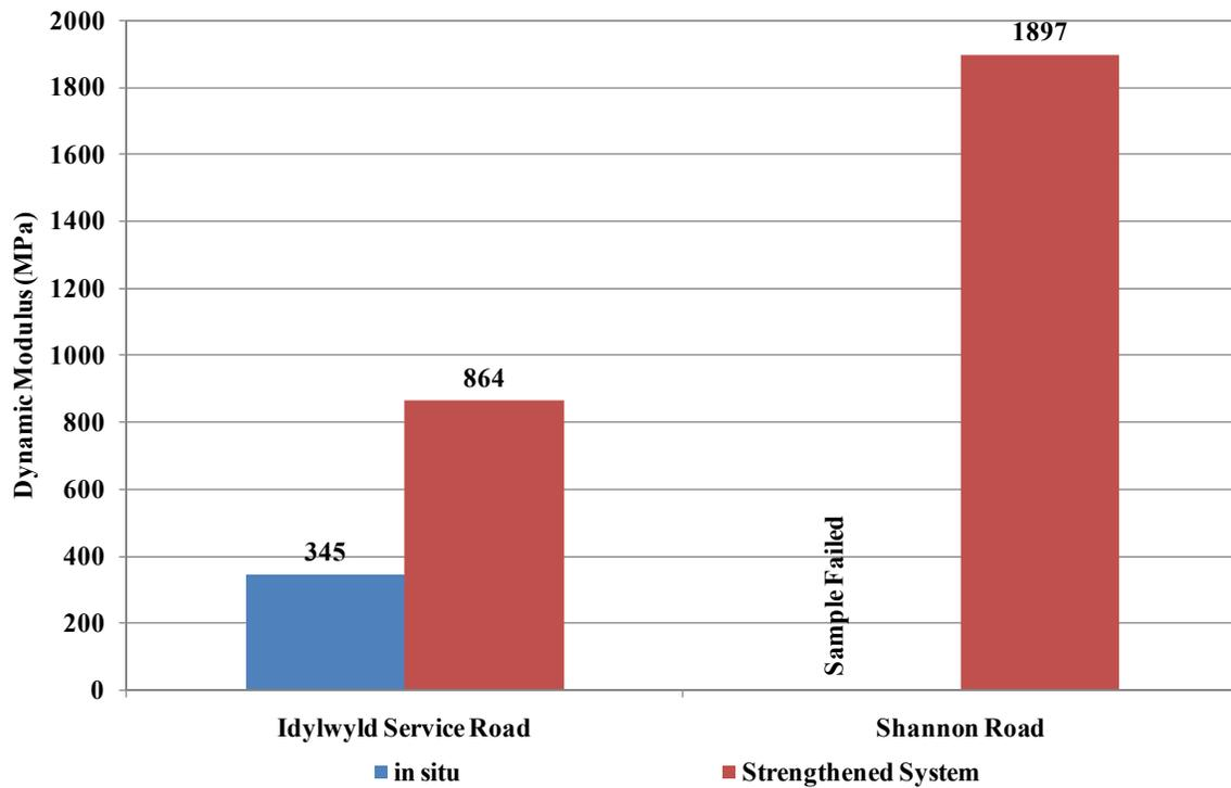
**Figure 1** Dynamic Modulus Averaged Across Stress State and Frequency
