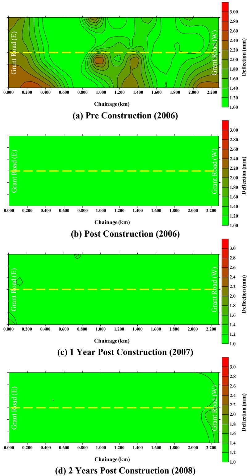
Figure 16 Shannon Road Peak Surface Deflection Profiles at Primary Weigh Limit+25%
