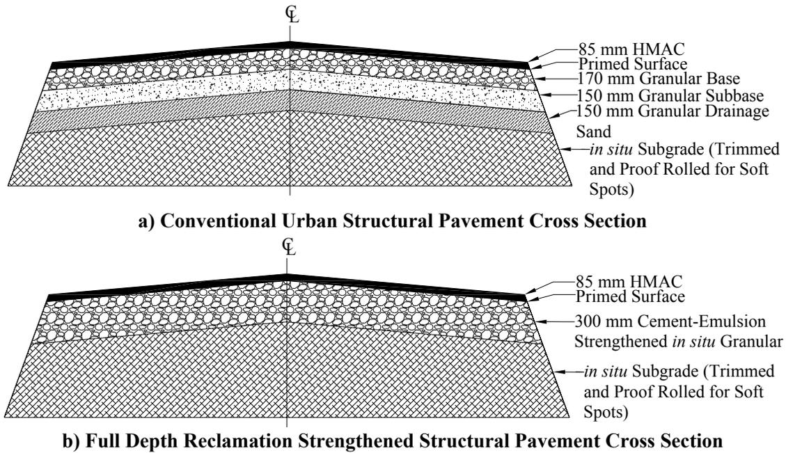
**Figure 11** Shannon Road Proposed Design Conventional and FDR Strengthened Design Cross Sections
