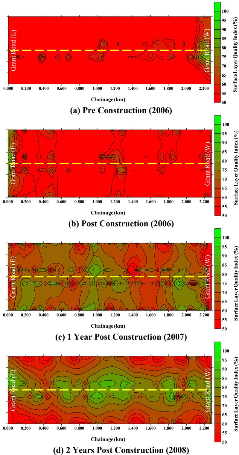
Figure 13 Shannon Road Surface Layer Quality Index Contour Profiles
