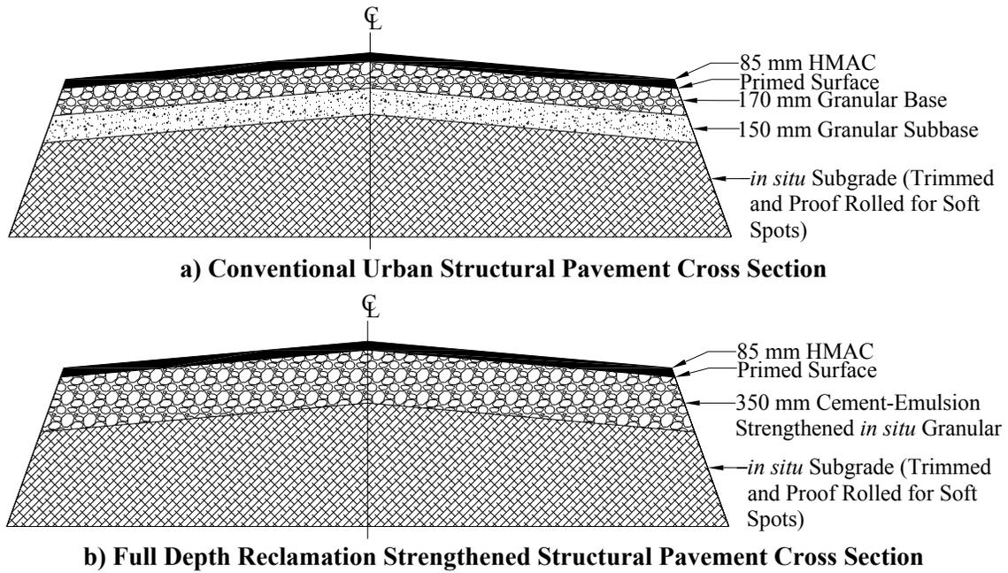
**Figure 4** Idylwyld Service Road Proposed Conventional and FDR Strengthened Design Cross Sections
