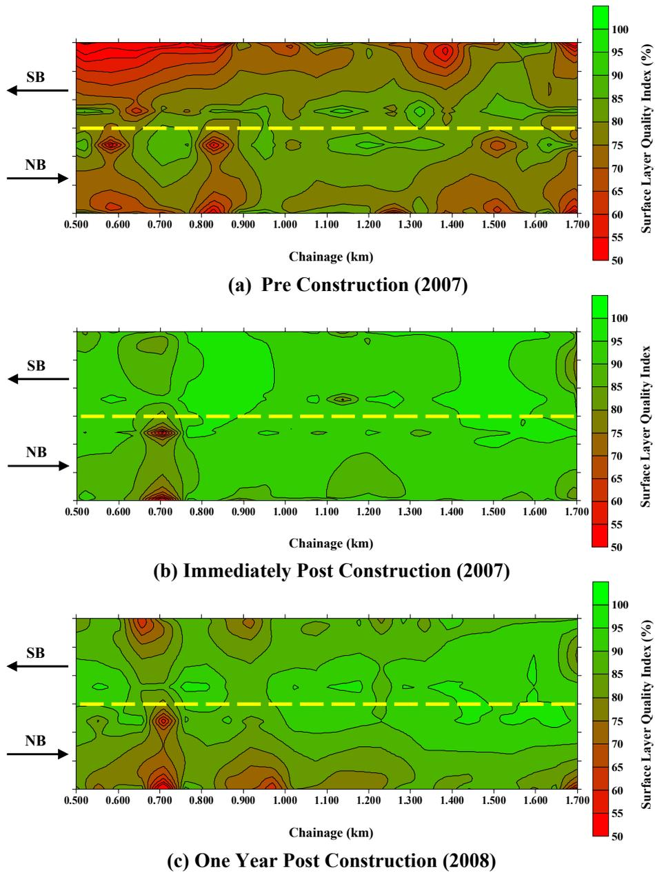
Figure 6 Idylwyld Service Road Surface Layer Quality Index Contour Profile
