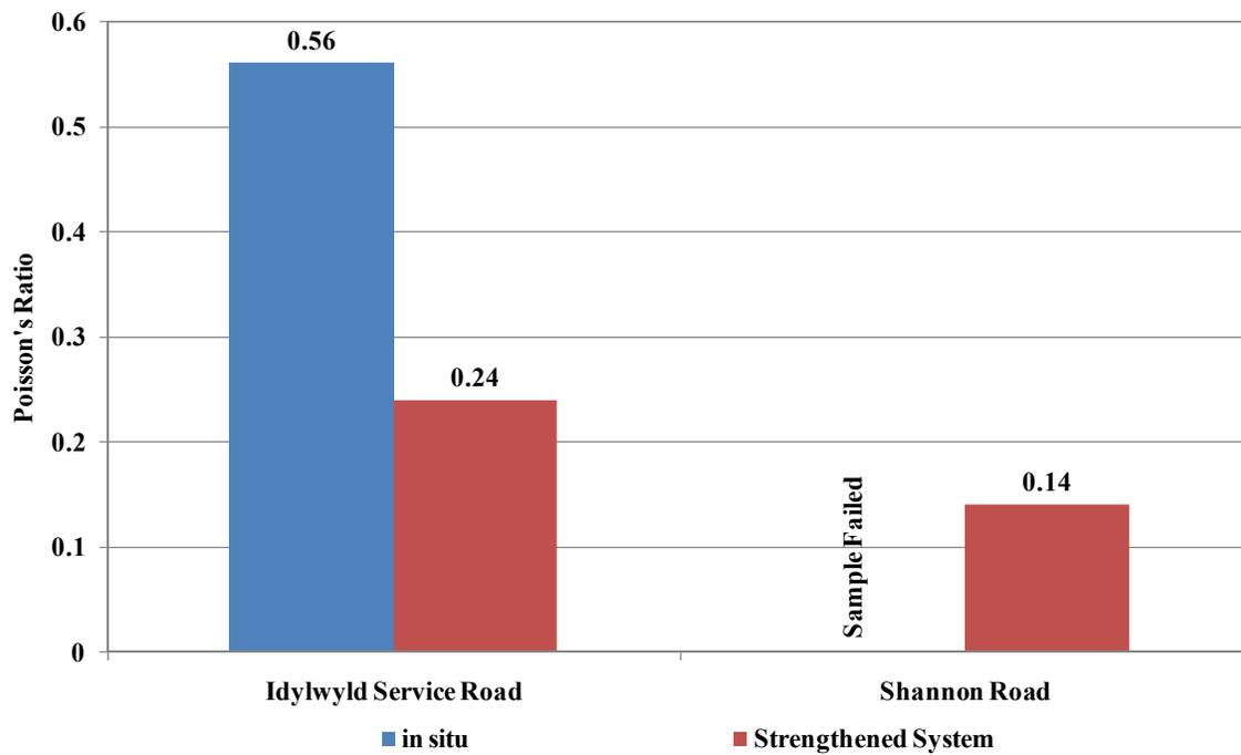
**Figure 2** Poisson's Ratio Averaged Across Stress State and Frequency
