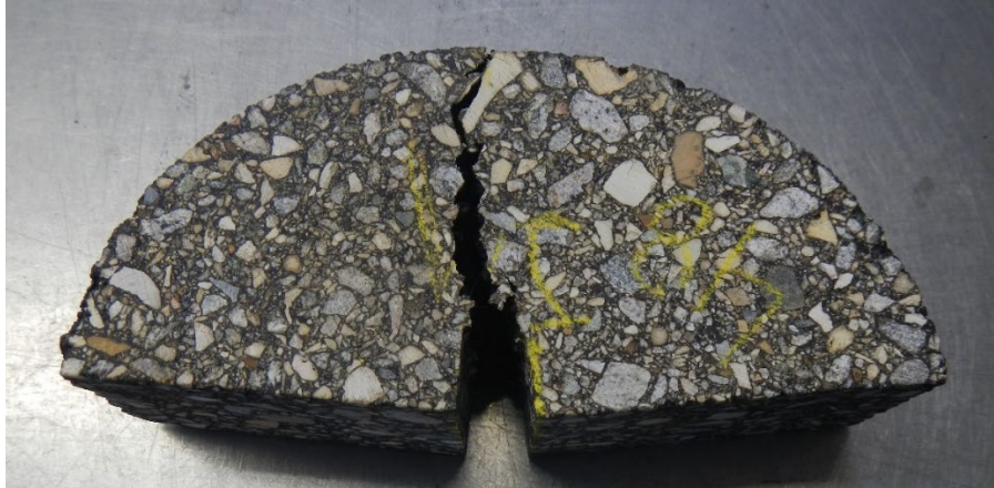
Figure 12. Example Photo of an Asphalt Concrete Core Specimen after I-FIT Testing
