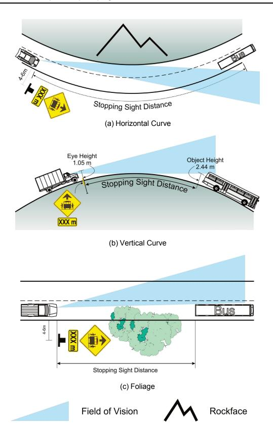
FIGURE 5.3 STANDARD LAYOUTS FOR WC-9 SIGN PLACEMENT
