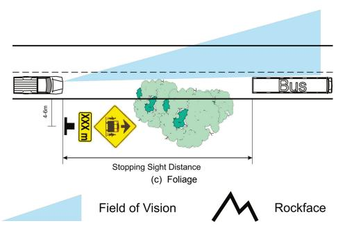
FIGURE ES.2 STANDARD LAYOUTS FOR WC-9 SIGN PLACEMENT
