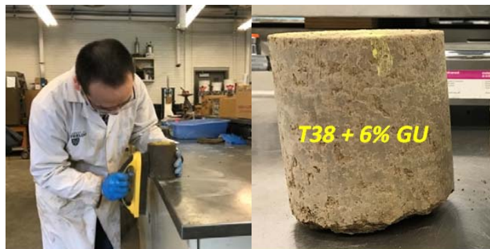
Figure 9. Brush strokes at surface (left), condition of T38 + 6% GU after the test (right)
