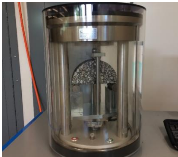
Figure 5: I-FIT Test using Semi-Circular Bending (SCB) specimen geometry.
