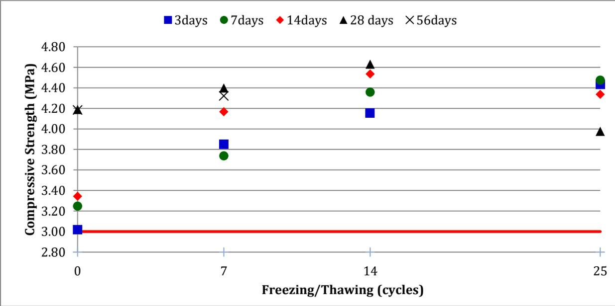
Figure 5: Compressive Strength for Regular and Conditioned Samples
