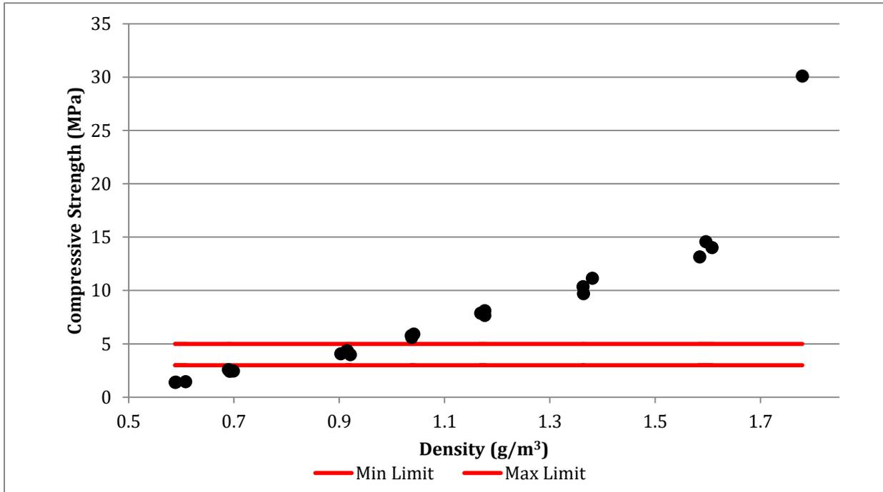
Figure 4: Compressive Strength Variations with Density
