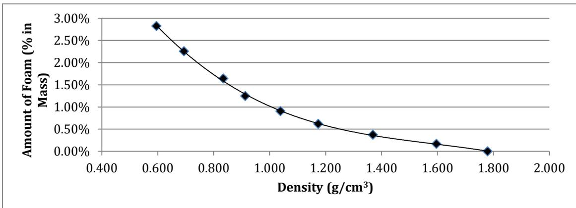
Figure 3: Mix Proportioning Curve
