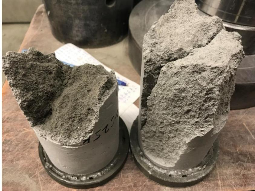
Figure 8: Water Absorption Samples Before (right) and After Conditioning (left).
