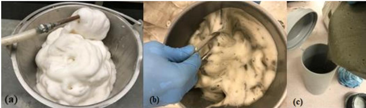
Figure 2: Sample Preparation. (a) Pre-formed dry foam. (b) Mixing. (c) Pouring in the molds
