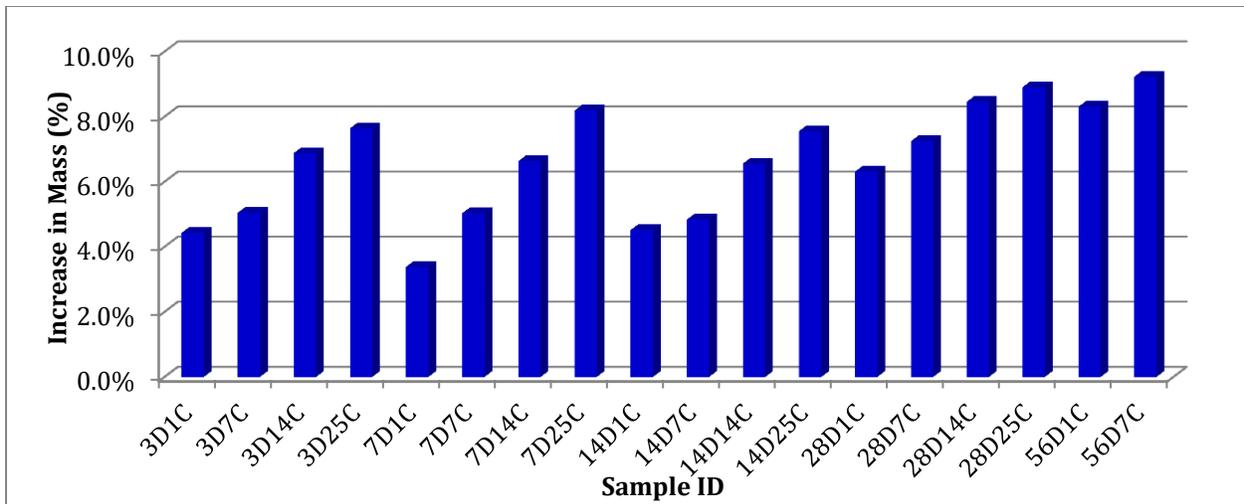
Figure 7: Water Absorption
