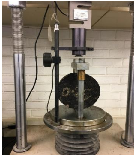
Figure 5 Indirect Tensile Test Set up
