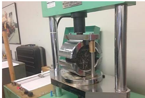
Figure 4 Marshall Stability Test
