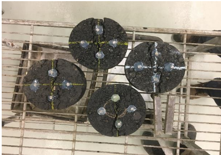
Figure 9 Mode of Failure of Indirect Tensile Specimens
