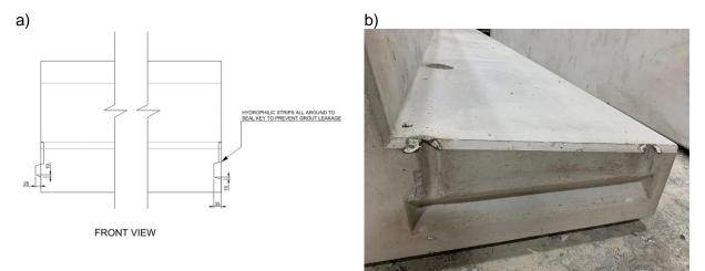
Figure 7 - Shear key: a) front view and; b) picture of the recessing portion of the shear key on the precast curbs
