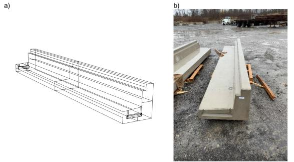
Figure 6 - Curbs designed for the corridor replacement program: a) 3D isometric view and; b) picture of a precast curb
