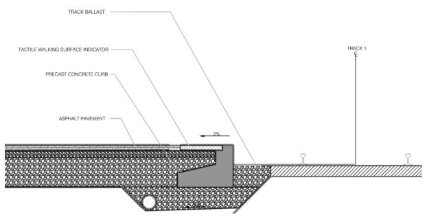
Figure 5 - Section cut of the new platform
