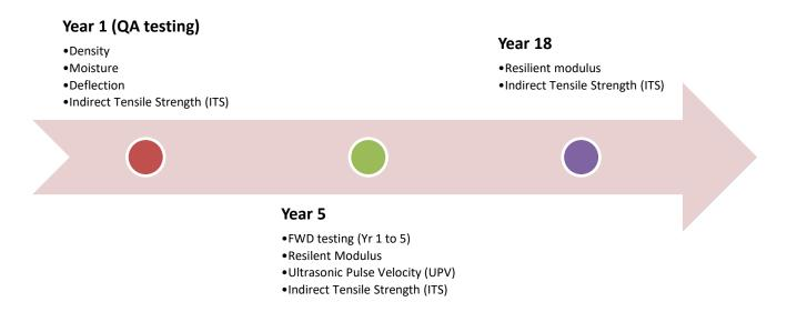
Figure 5: Performance Testing Timeline
