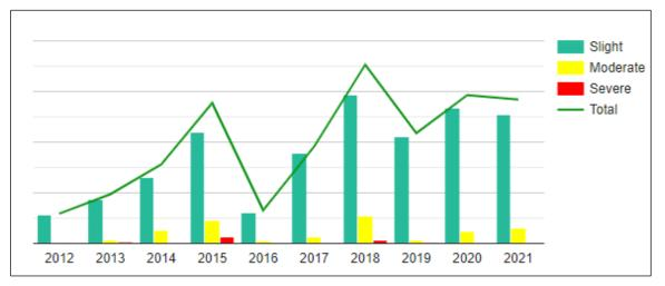
Figure 9. 2012 to 2021 Total Crack Length for Combined CIR and CIREAM Sections
