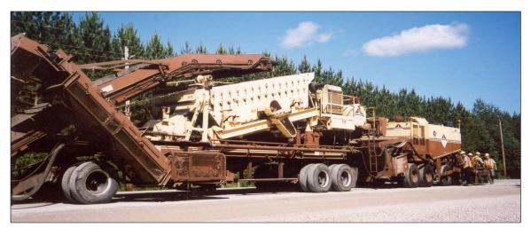
Figure 2. Cold-In-Place Recycling Train
