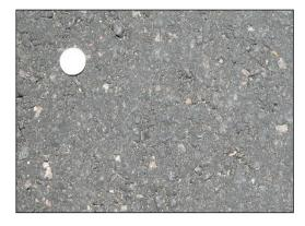
Figure 4. a) Finished Surface of CIR Mix
