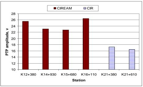
Figure 6. UPV Test Results of CIR and CIREAM
