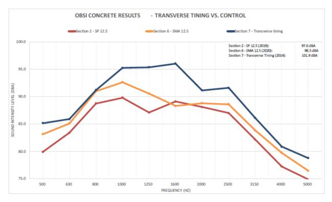
Figure 11. Comparison Between Concrete Transverse Tining and Asphalt Control Section
