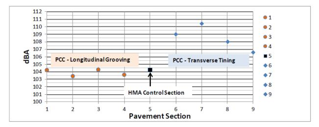
Figure 4. Longitudinal Grooved and Transverse Tined Noise Level
