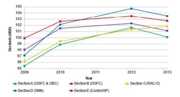
Figure 1. Noise Reduction Performance of Asphalt Surface Course Trials
