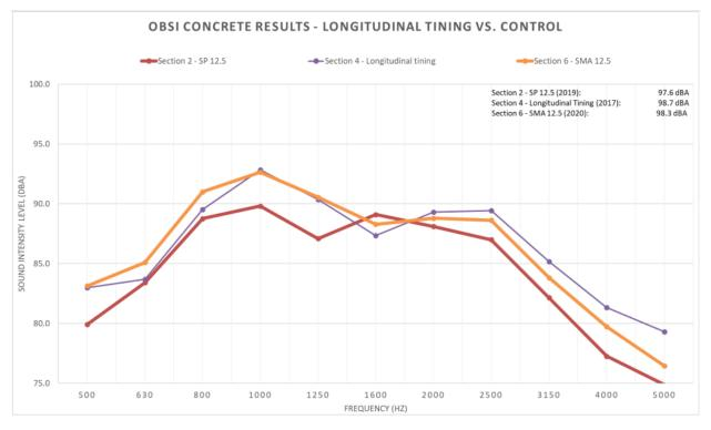
Figure 10. Comparison Between Concrete Longitudinal Tining and Asphalt Control Section
