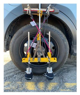
Figure 6. AASHTO-Compliant OBSI Test Rig Used in Measurements
