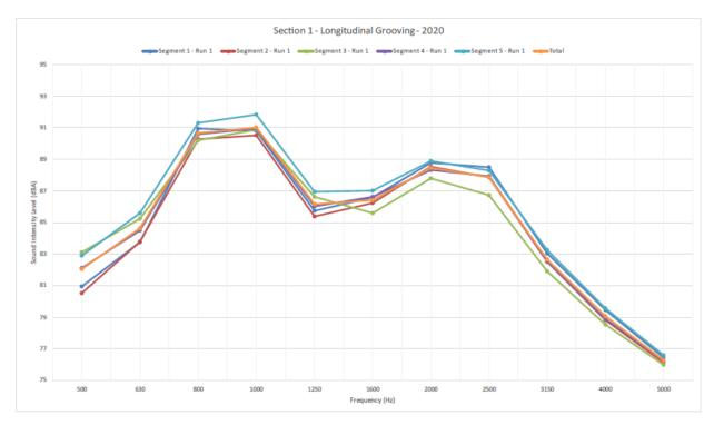
Figure 8. Variability in Measured Sound Intensity Within the Test Sections
