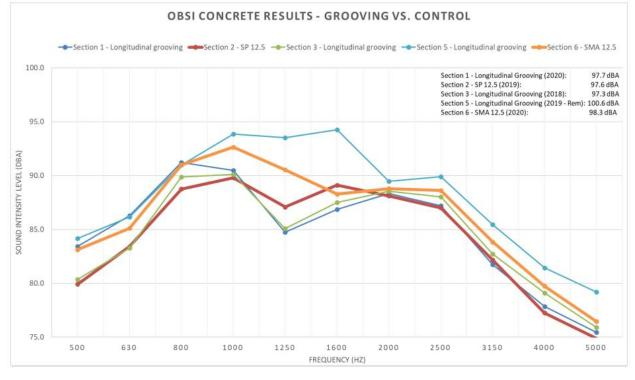
Figure 9. Concrete Longitudinal Grooving versus Asphalt Control Section
